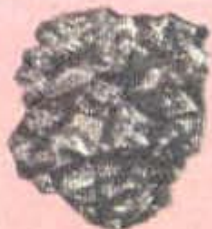
Uneven fracture: arsenopyrite
