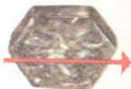
Basal cleavage: mica
