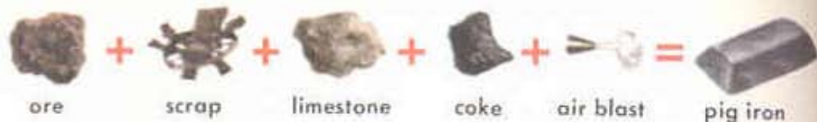
ore + scrap + limestone + coke + air blast = pig iron
