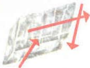
Rhombohedral cleavage: calcite
