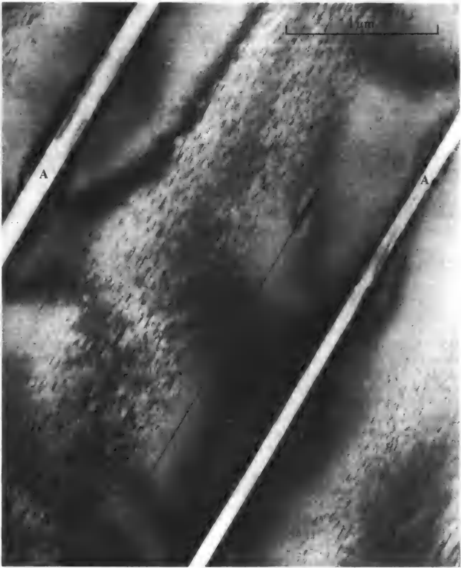
Fig. 16. Electron micrograph showing large (100) augite lamellae (A) and a fine distribution of Ca-rich platelets in orthopyroxenes (Champness and Lorimer, 1973).
