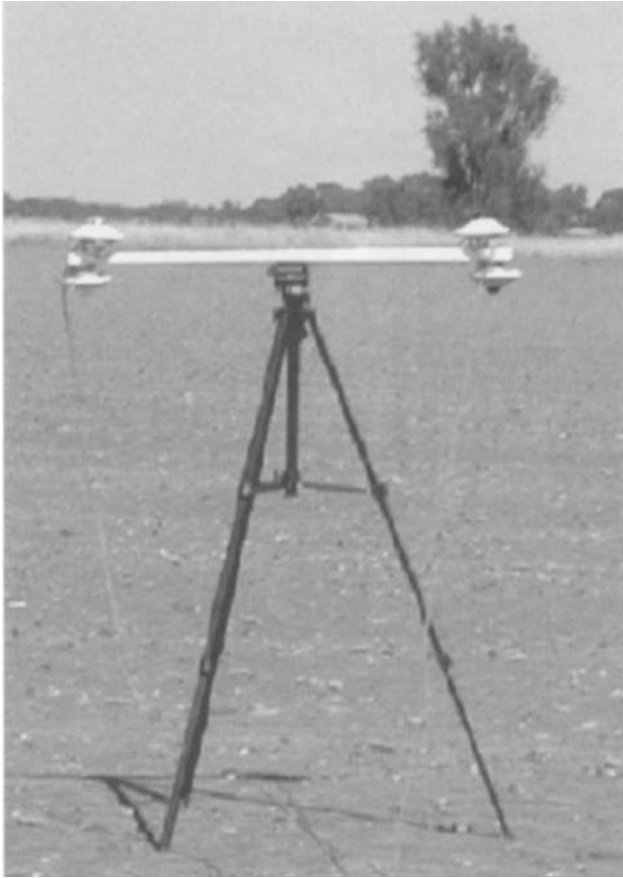
Figure 12.5 Two albedometers at the two ends of a tripod in the field.
