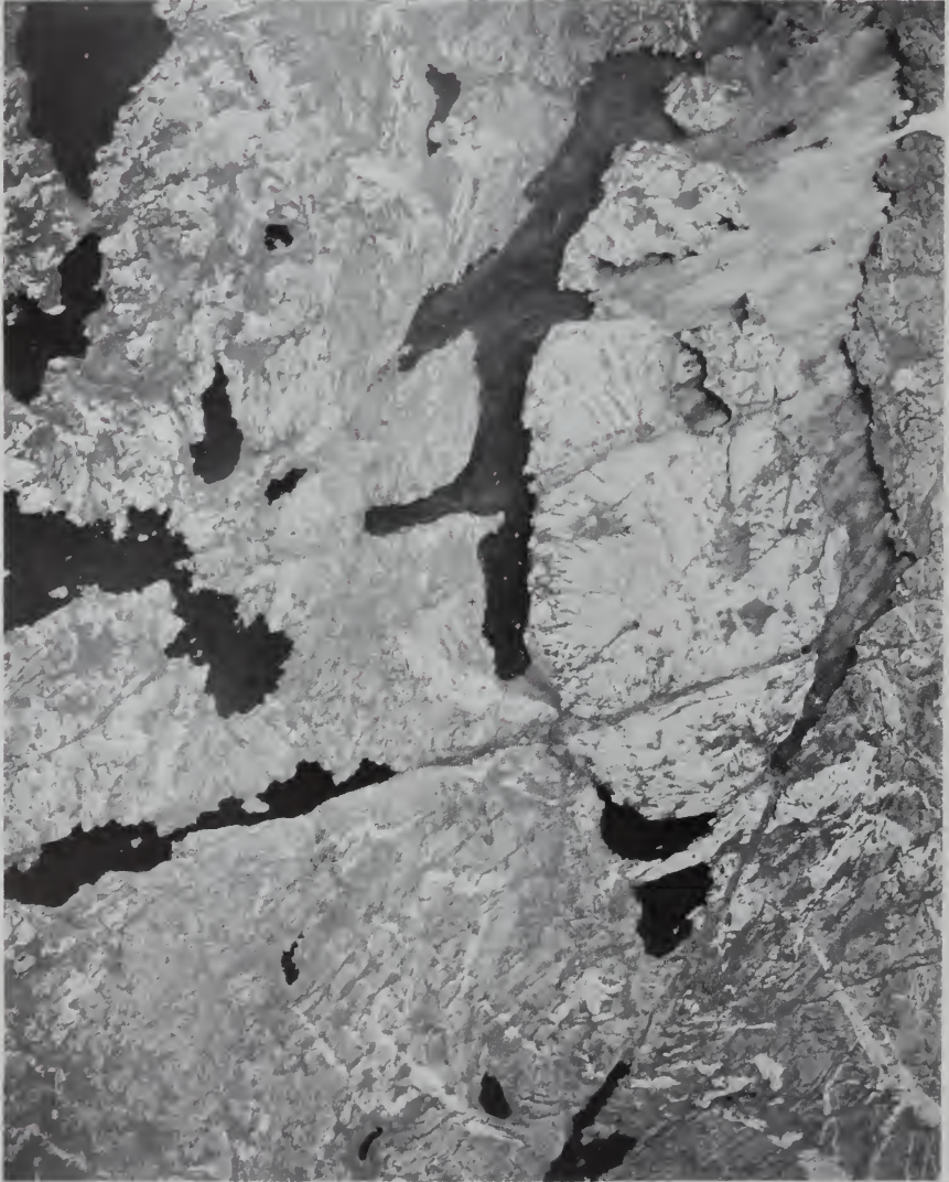
FIG. 21.15. Vertical photo showing early Pre-Cambrian sediments (dark gray) near Duncan Lake Northwest Territories, Canada, intruded by granite (light gray) bodies as much as one-half mile wide. Both of these are intruded by later Pre-Cambrian diabase dikes (dark gray). (Royal Canadian Air Force photo.)
