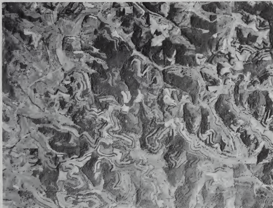
FIG. 21.12. Vertical photo of a portion of Gellie County, Ohio, on which the contour pattern of the fields and vegetation indicate nearly horizontal sedimentary rock strata. (Production and Marketing Administration photo.)
