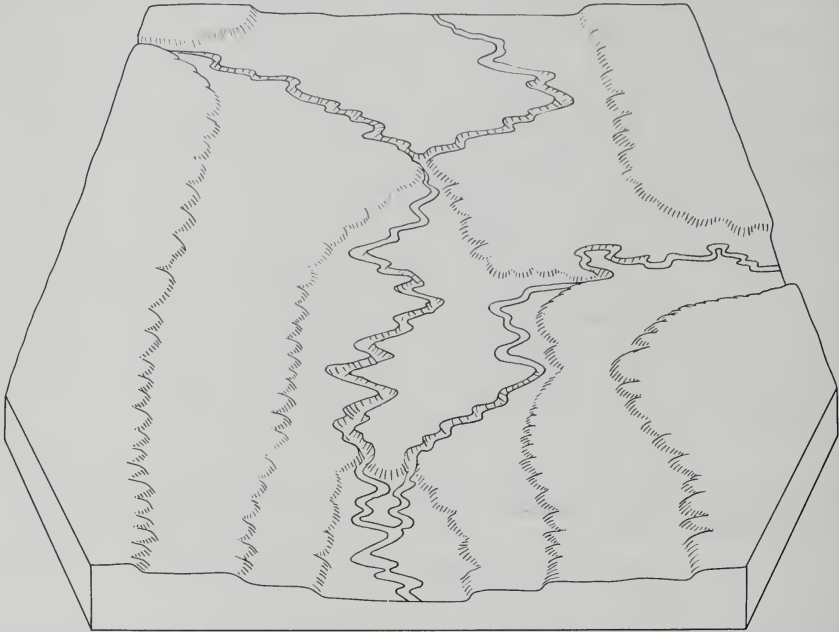
FIG. 8.7. Three stages of terrace development, according to the treppen concept of upstream migration of nickpoints and parallel retreat of slopes. (After H. A. Meyerhoff and M. Hubbell.)
