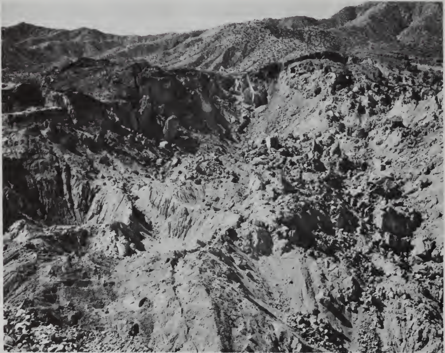
FIG. 22.4. Subsidence resulting from block caving at Ray, Arizona. This artificially induced subsidence simulates oxidation subsidence. (Photo by Paul Whitehead, Kennecott Copper Co.)
