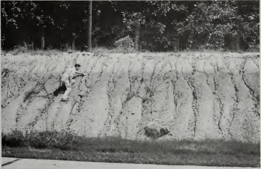
FIG. 4.5. A soil profile in Illinoian till. The man's hand rests at the contact between the A and B horizons, and his foot is at the contact between the B and C horizons. (Photo by Engineering Experiment Station, Purdue University.)
