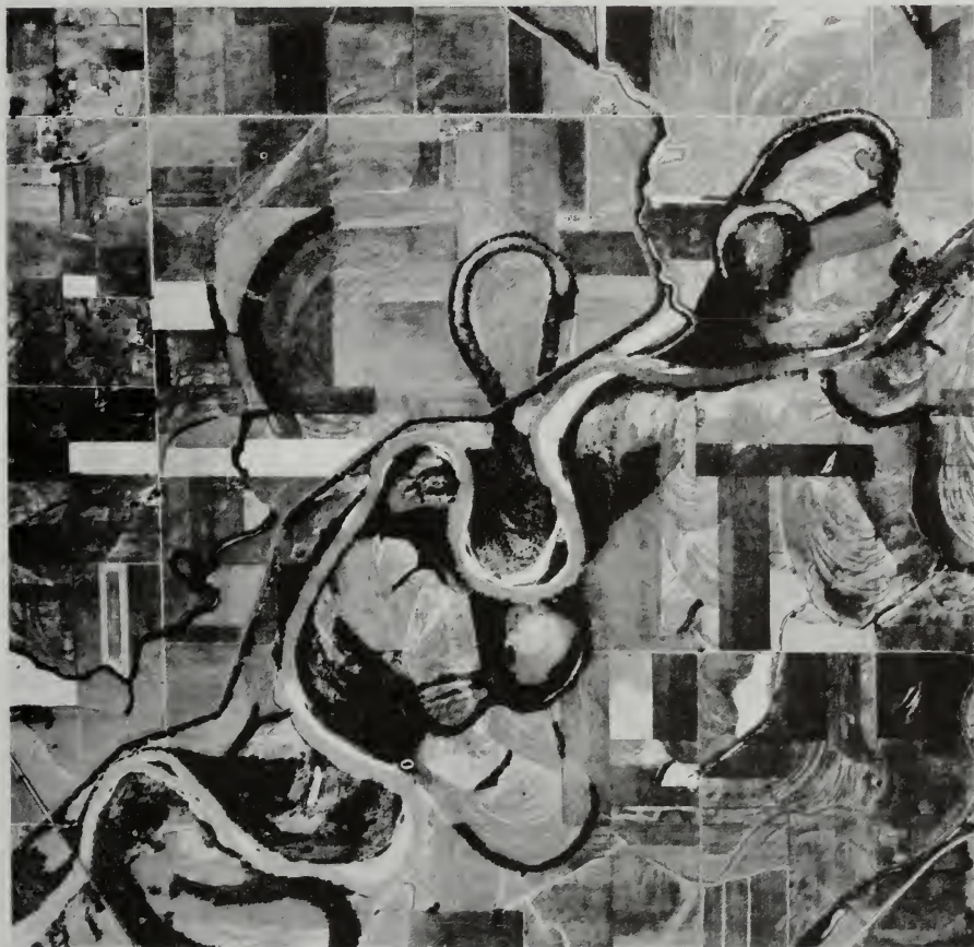
FIG. 7.3. Vertical photo of portion of White River Valley, Greene County, Indiana, showing details of a floodplain. Several meander cutoffs are shown, and point bar deposits are shown by the many light lines. (Production and Marketing Administration photo.)
