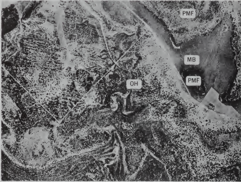
FIG. 21.10. Vertical photo of an area in San Saba County, Texas, which shows how outcrop belts of geologic formations are indicated by vegetation differences. PMF, Pennsylvanian Marble Falls limestone; MB, Mississippian Barnett shale; and OH, Ordovician Honeycut dolomite and limestone. Mesquite vegetation characterizes the areas of Barnett shale, whereas the areas of the Honeycut and Marble Falls formations have cedars, live oaks, and other trees. (Production and Marketing Administration photo.)
