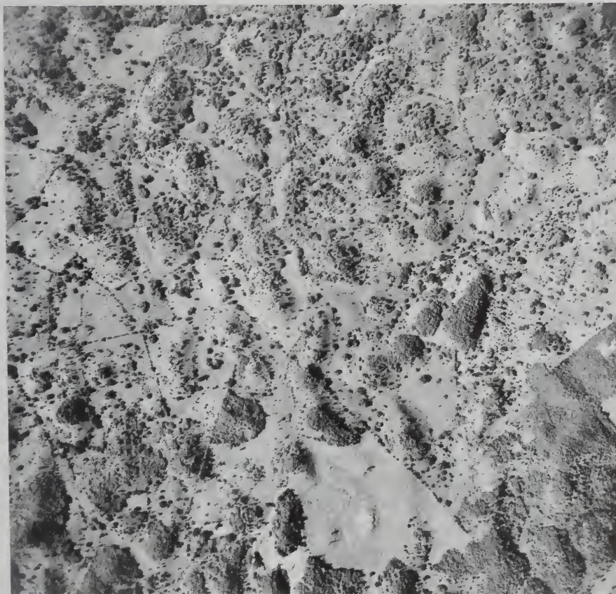
FIG. 22.5. Vertical photo of part of the Parish of St. Ann, Jamaica, showing the karst topography on which bauxite is found. Bauxite occupies the untimbered basins and sinkholes between residual limestone knobs. (Photo courtesy Reynolds Jamaica Mines, Ltd.)
