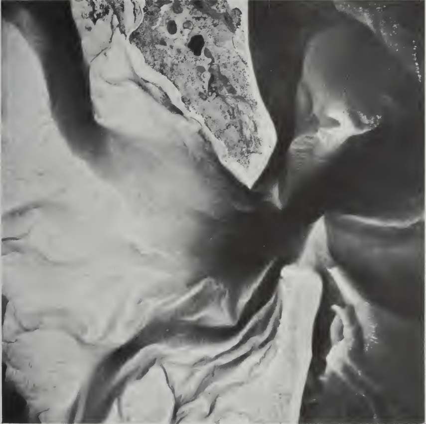
FIG. 18.6. Vertical photograph taken off the coast of Mozambique, Africa, showing troughs, bars, tidal channels, and other details of near-coastal submarine topography. (Courtesy Gulf Oil Corporation.)
