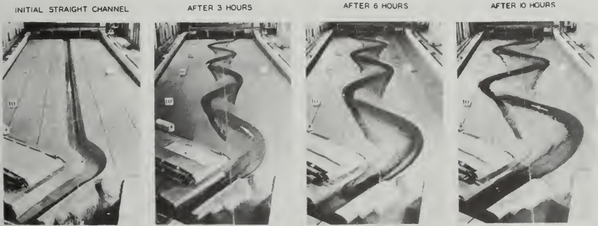
FIG. 1.1. A . Model of a typical bend in the Mississippi River in which simulated articulated concrete mattress-type revetment is being tested as part of a channel stabilization program. (Corps of Engineers photo.) B . Laboratory study of stream meandering. (Corps of Engineers photo.)
