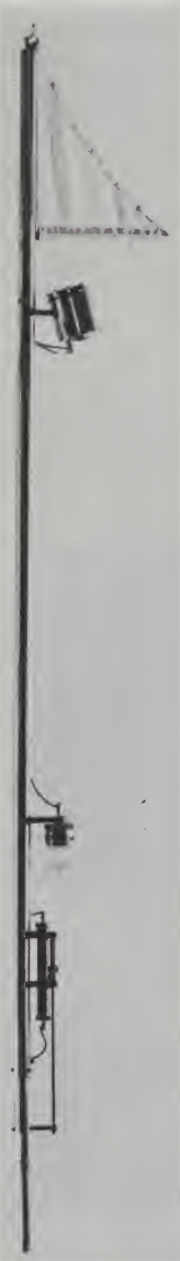
FIG. 18.2. The Ewing underwater camera. The sail at its top is to retard rotational movement; below the sail is the camera and below it the lamp housing; below the lamp housing is a battery case and part of the triggering mechanism; a coring tube and the remainder of the triggering mechanism are at the bottom. (Courtesy of Maurice Ewing.)
