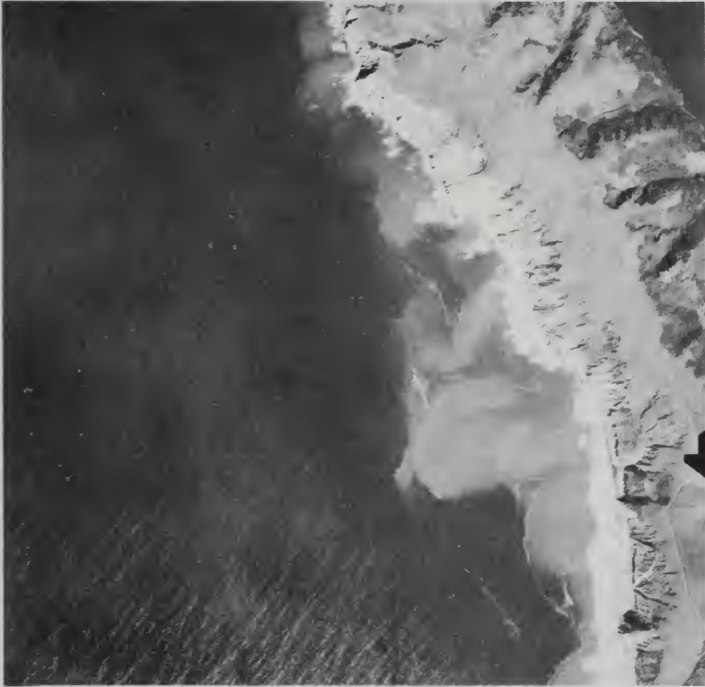
FIG. 17.2. Vertical photo, Marino County, California, showing rip currents extending seaward. (Production and Marketing Administration photo.)
