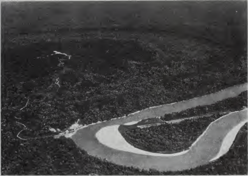
FIG. 21.11. The Ganzo Azul oil dome near Pucallpa, Peru, a domal structure in a tropical rain-forest area where no bedrock is exposed, but which is outlined by tonal differences in vegetation related to varying lithology. (Courtesy American Geographical Society.)
