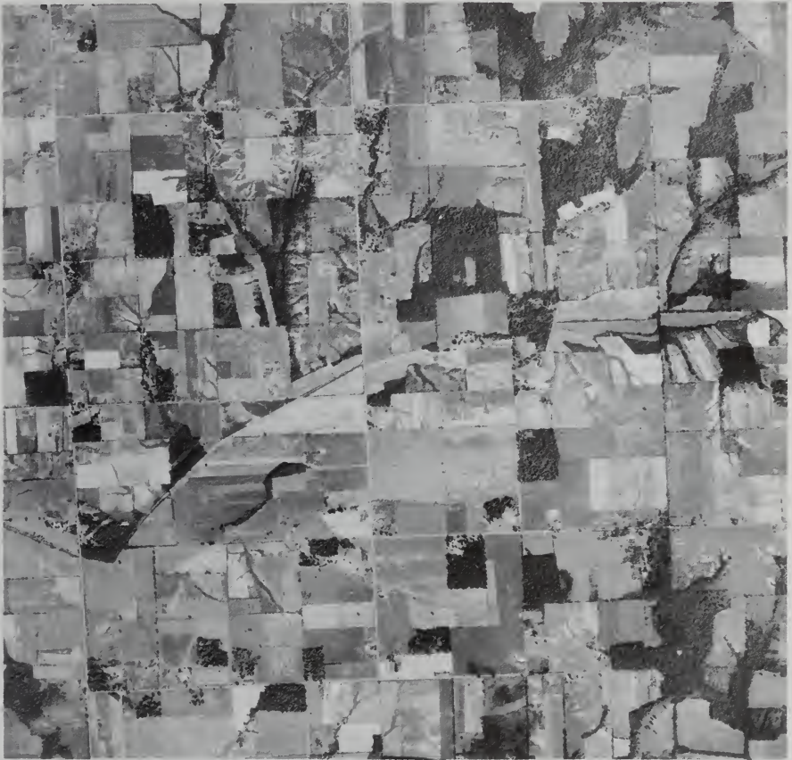
FIG. 21.9. Vertical photo of an area of Illinoian till plain in Scott County, Indiana. The lacy pattern along tributary stream is a diagnostic airphoto pattern of Illinoian till. (Production and Marketing Administration photo.)
