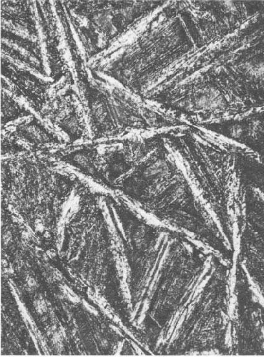
Figure 3.36 Spinifex texture in an Archean komatiite from the Barberton greenstone in South Africa ( \times 6 ). Radiating crystals are serpentine pseudomorphs after olivine.
