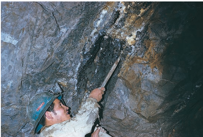
FIGURE 7.17 A wide vein that contains masses of sphalerite (dark), pyrite and chalcopyrite (both shiny yellow), as well as white quartz, in the Casapalca mine in Peru. It was mined for zinc and copper. Photo © Brian Skinner
