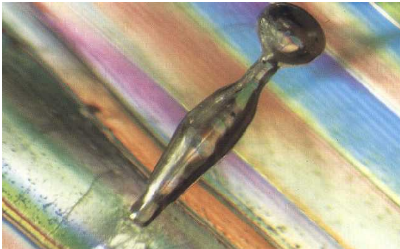
[PLATE 35] Bytownite feldspar from New Mexico (magnification 20 x; Gemological Institute of America). Photo by John Koivula using a Nikon SMZ-10 microscope and crossed polarizers to bring out the twin lamellae and carbon dioxide inclusion.
