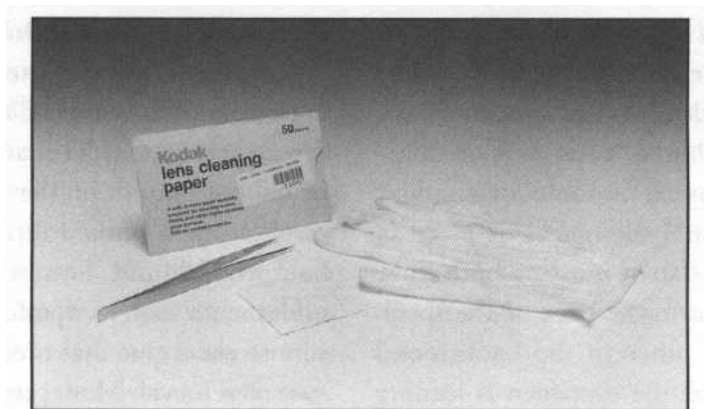
Figure 2-2 Items for handling and cleaning specimens. Left to right: tweezers, lens cleaning tissue, jewelry polishing cloth, and cotton glove.
