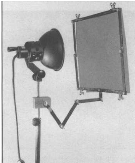
Figure A-6 Homemade gel/filter holder of 1/8 x 1/2 inch flat aluminum stock painted black. Joints are fastened with nuts, lock washers and bolts, or thumbscrews. Mounted to light stand with adapter block. (see Figure A-7)
