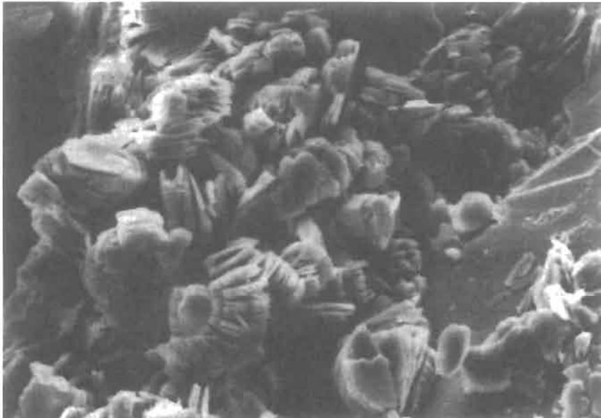
Figure 10.9. SEM microphotograph of pore-filling kaolinite plates. (Courtesy of Core Laboratories.)
