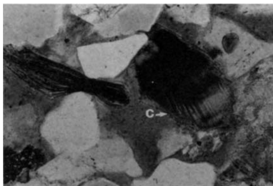
Fig. 2.22 A thin-section photomicrograph of a fine-grained micaceous sandstone from the Marnock Field, UK continental shelf. The porosity in the sample has been infilled with a resin. Most of the grains are quartz. The fibrous grain on the left is biotite (mica). All of the grains are coated with chlorite (C). The photograph was taken using a combination of cross-polarized light and a quarter-wavelength plate. Field of view 650\ \mu\text{m} \times 450\ \mu\text{m} . (Reproduced courtesy of BP.)
