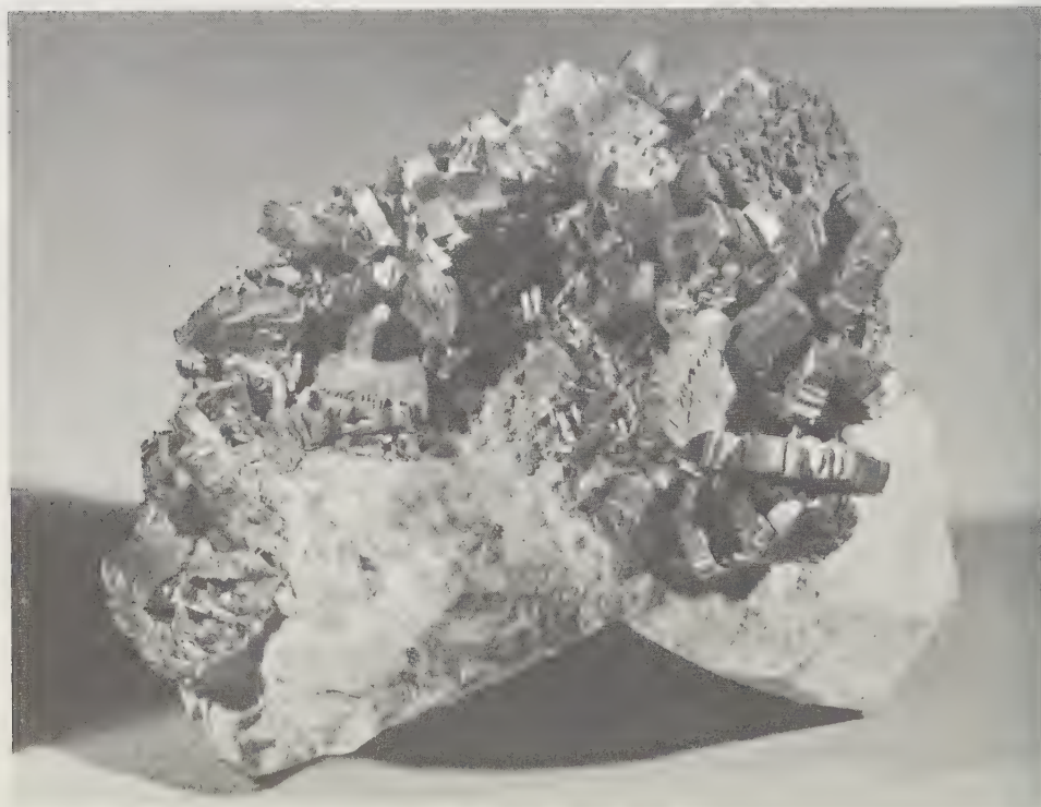
FIG. 132. Marcasite in cockscomb growths upon chert breccia fragment. Size 3\frac{1}{2} " by 3". From Joplin, Missouri. The sharp wedge-shaped terminations consist of a pair of e(101) faces, many of which are exposed because of repeated twinning which forms the fan-like sprays. The sides of the sprays are b(010) faces.
