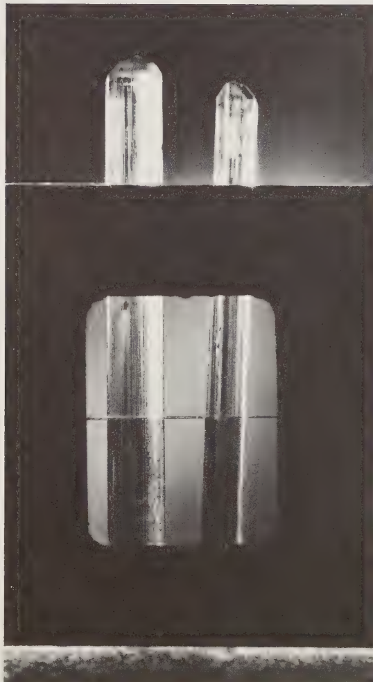
FIG. 100. An actual photograph of dichroism in tourmaline crystals. A small Eureka Polaroid sheet dichroscope has been placed before two slender pink crystals from the Himalaya Mine, San Diego County, California. Ordinary light is allowed to shine through the back. The segments of Polaroid are "crossed," the upper segment showing a very pale pink hue, but the lower showing a much darker pink, corresponding to the two dichroic colors observable in these crystals.
