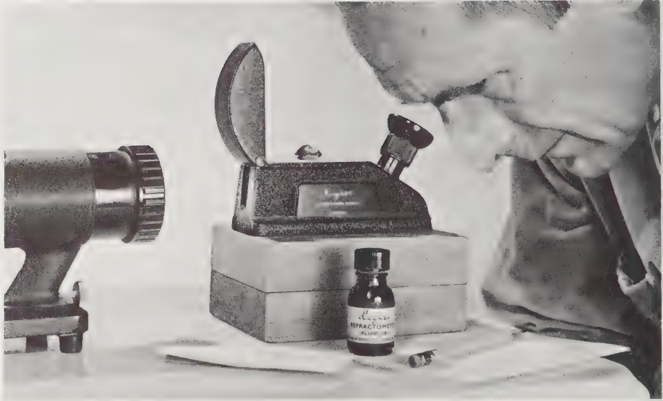
FIG. 104. The Rayner refractometer in use. The slide projector at the left shines a powerful beam of light into the refractometer window just beneath the raised hood. The light passes through a frosted glass screen and is reflected upward through a glass prism into the faceted gemstone seen resting upon the prism. Some is reflected downward through an additional optical system, and made to pass through a calibrated screen. Through the eyepiece one can read the refractive index directly on the screen. Note the small bottle of high index fluid in the foreground. Before the specimen is placed on the glass prism of the instrument, a small droplet of this fluid must first be applied to establish optical contact between the specimen and prism.
