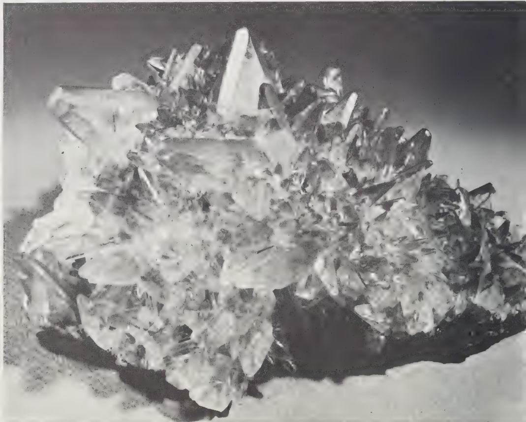
FIG. 176. Calcite crystals of scalenohedral habit, essentially colorless but partly coated by vivid red hematite. From Frizington, Cumberland, England. Size 5\frac{1}{2} " by 3\frac{1}{2} ".
