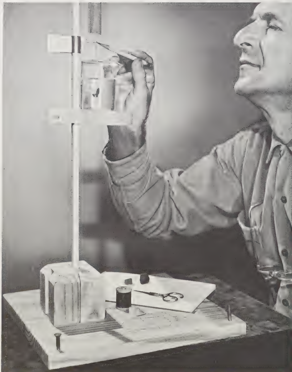
FIG. 86. Jolly balance in use. A specimen is suspended from thread at the lower end of the tension spring and is immersed in water for the weight-in-water reading. The author is checking the metal slider mark against the mark on the spring to see if marks match. The reading is taken from the strip of marked graph paper seen on the back side of the metal curtain rod.
