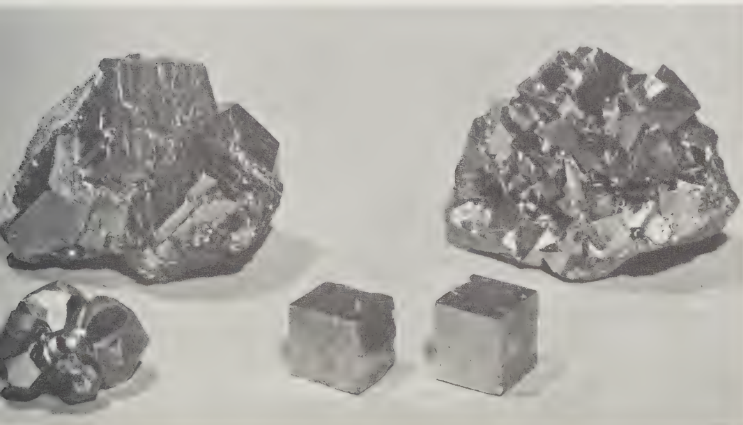
FIG. 129. Pyrite. Top left: modified pyritohedrons on matrix of specular hematite. Size 3½" by 3". Rio Marina, Elba, Italy. Top right: sharp octahedral crystals on massive pyrite from Morococha, Peru. Size 3½" by 2½". Bottom left: highly modified crystals in a cluster from Elba. Forms include cube, pyritohedron, octahedron and diploid. Size 1¾". Bottom center: simple cubes from Elba.
