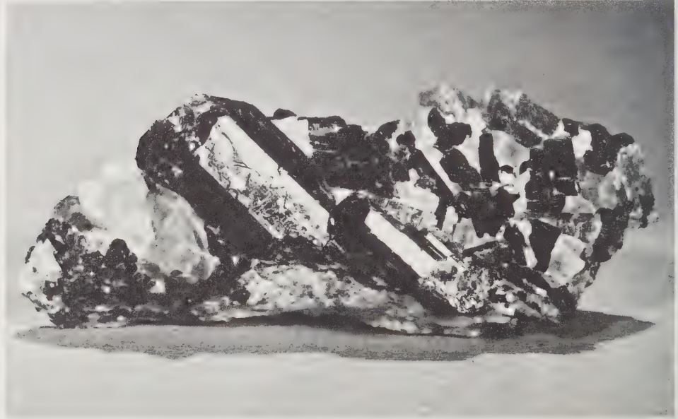
FIG. 278. Dark green diopside crystals in calcite with chalcopyrite, apatite and fluorite. Size 3\frac{1}{4} " by 1\frac{1}{2} ". From Huddersfield, Quebec. Crystals are rounded on edges, as if partly fused. Elongated along the c axes. Prism zone bounded by prism m[110] and pinacoids a[100] and b[010] .
