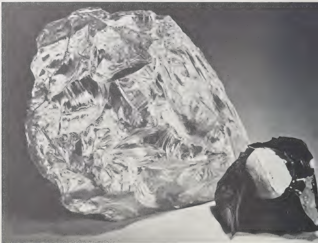
FIG. 77. Conchoidal fractures developed upon rock crystal quartz (left) and obsidian (right). The mass of quartz is cobbled from a much larger crystal and is virtually flawless. It measures about 7\frac{3}{4} " in diameter and originated from an unstated locality in Minas Gerais, Brazil. Conchoidal fractures are perfectly developed upon the obsidian specimen which comes from Coso Hot Springs area of Kern County, California. The latter specimen exposes a spherical inclusion of grayish-white cristobalite.
