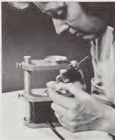
FIG. 101. Testing a thin cleavage flake of mica for a biaxial figure between the crossed polaroids of the Gemological Institute of America's polariscope. Light is provided from underneath by a small microscope substage lamp. The glass stirring rod ball-tip acts as a powerful but easily maneuvered magnifying glass to enlarge axial figures to the point where they can be clearly seen.
