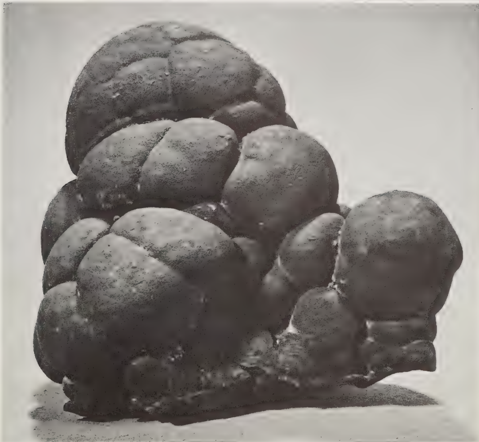
FIG. 153. Pyrolusite. Black reniform mass from surface workings in a manganese deposit in Sonora, Mexico. Size 4" by 4".
