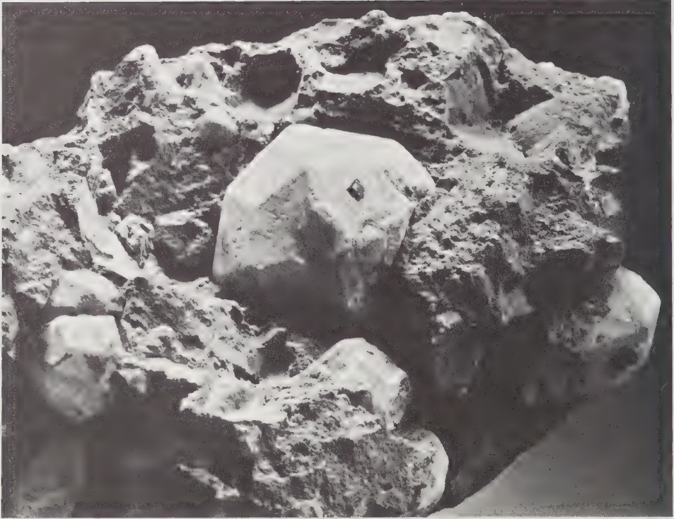
FIG. 252. Leucite trapezohedrons in pale gray volcanic tuff. From Ariccia, near Rome, Italy. Largest crystal 1" in diameter.
