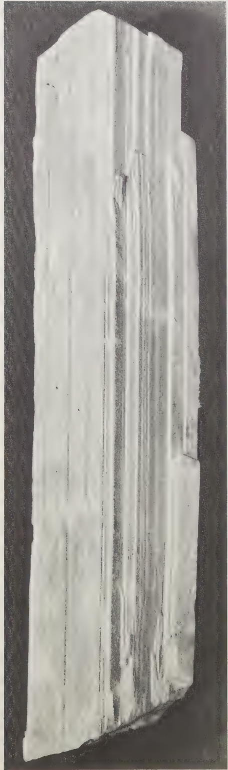
FIG. 157. Stibiconite replacing large stibnite crystal. Note how faithfully the typical striations of stibnite crystals are preserved. From Catorce, San Luis Potosi, Mexico. Size 6\frac{1}{4} ".
