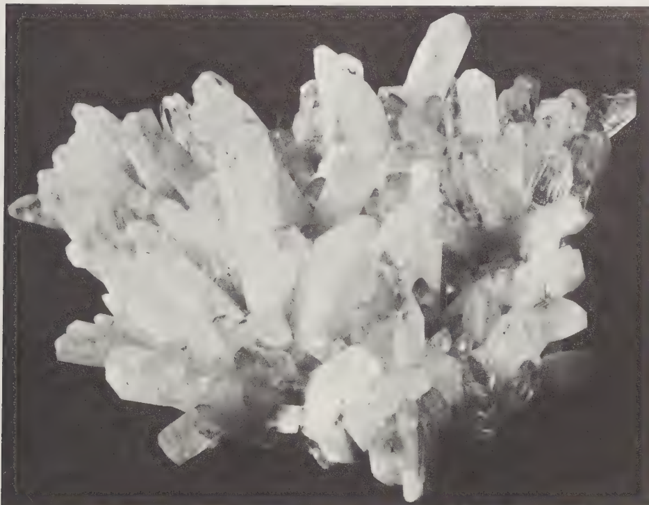
FIG. 251. Danburite group. Colorless to white crystals from Mina San Sebastian, Charcas, San Luis Potosi, Mexico. Size 4" by 3". Crystals elongated parallel to c axis and displaying forms shown in Figure 250.
