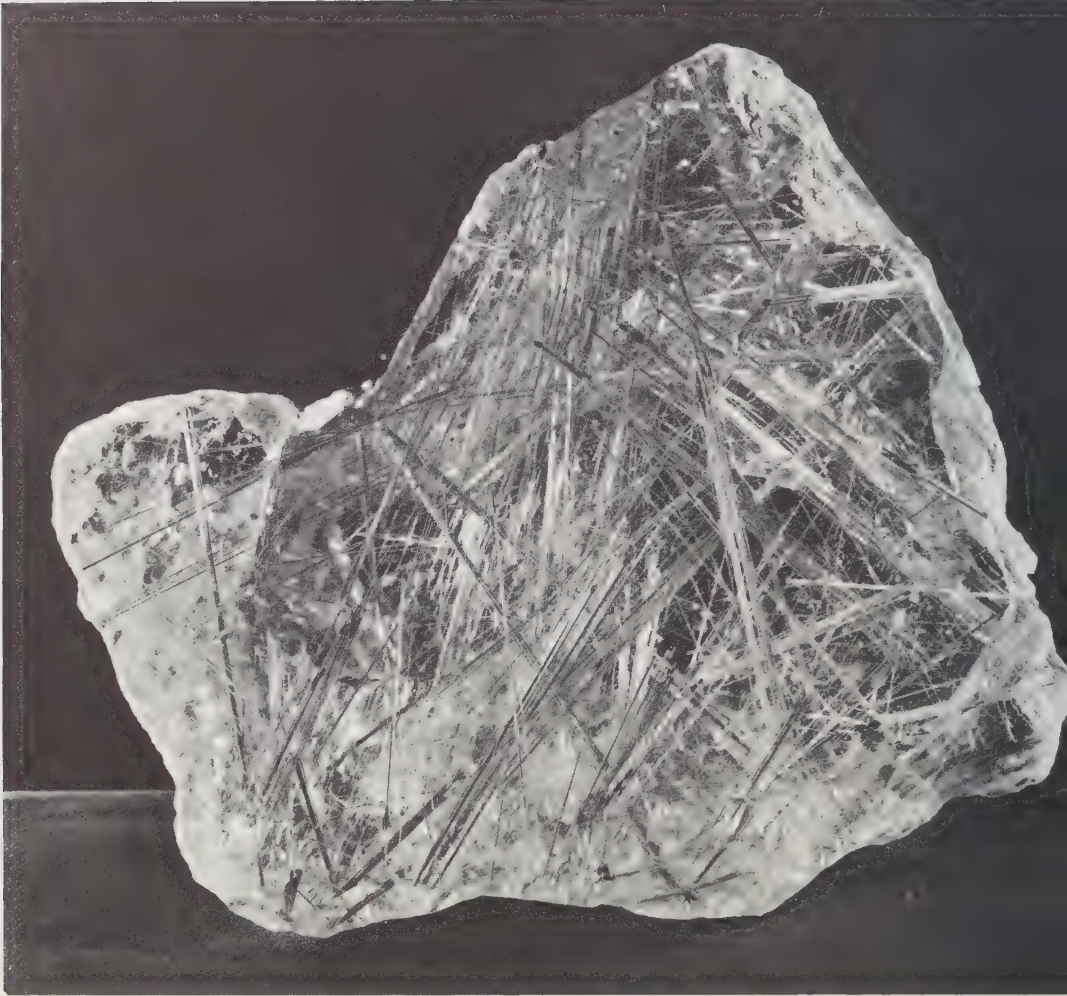
FIG. 32. Slender coppery-hued rutile needle crystals in clear rock crystal quartz. Such crystals grew in a cavity before the crystallization of the quartz and were enveloped later. Size of specimen 6" by 5". Front face polished. Minas Gerais, Brazil.
