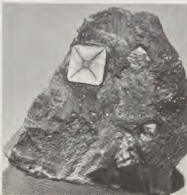
FIG. 309. Andalusite, variety chiastolite . Prismatic crystals enclosed in chlorite schist, from Chowchilla, Madera County, California. The large crystal at the upper left has been ground and polished to show the typical cross markings of this variety. Untouched fractured prisms appear at top right and lower right. Size 3\frac{1}{2} " by 3". Specimen in Elbert H. McMacken Collection, Ramona, California.
