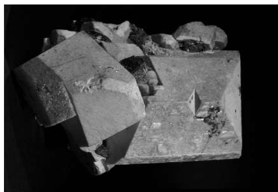
Fig. 19.21 Euhedral crystals of orthoclase from Wieza, Poland (width 95 mm) (courtesy A. Massanek).
