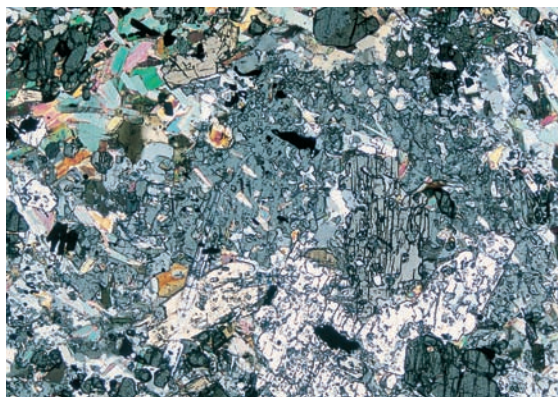
(d) Pelitic schist with all three aluminosilicates coexisting, from Cataeggio, Bergell Alps, Italy. A large porphyroblast of andalusite includes crystals of kyanite and a needle of sillimanite. Dark mineral is garnet, the crystal on the left side is staurolite. (Width 6 mm.)
