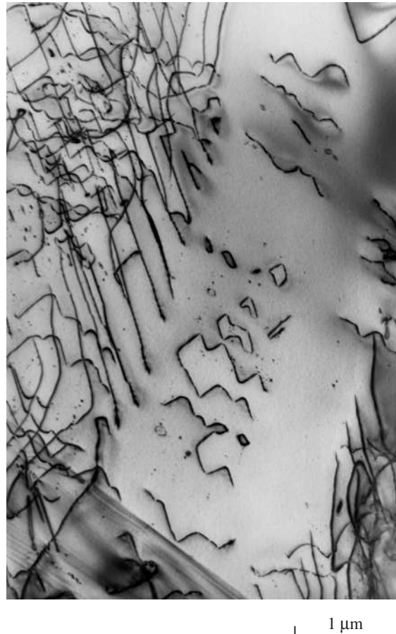
Fig. 6.10 TEM image of dislocations in experimentally deformed dolomite (courtesy D.J. Barber; see also Barber et al. , 1981).
