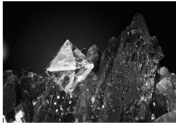
Fig. 5.8 Quartz from Westerwald (Germany), with hexagonal morphology reminiscent of its original formation as high-temperature hexagonal \beta -quartz. It is now trigonal (width 30 mm) (courtesy O. Medenbach).
