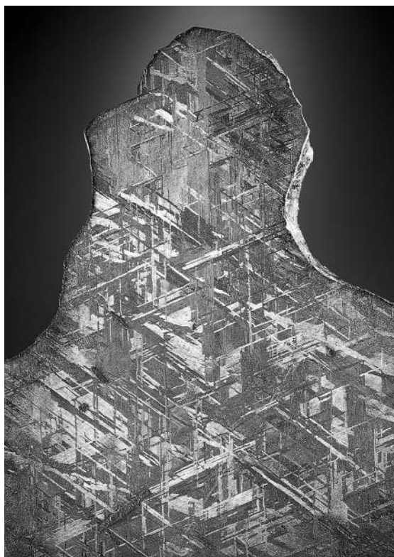
Fig. 20.6 Widmanstätten's pattern, an intergrowth of kamacite and taenite, observed in meteoritic iron. Gibeon meteorite, Namibia (width 80 mm) (courtesy O. Medenbach).
