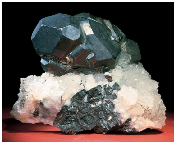
(a) Cube-octahedral galena from Freiberg, Germany (courtesy A. Massanek.) (Width 65 mm.)
