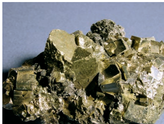
(c) Chalcopyrite from Morococha, Peru, with pyrite (cubes) and sphalerite (black) (photograph P. Gennaro). (Width 40 mm.)
