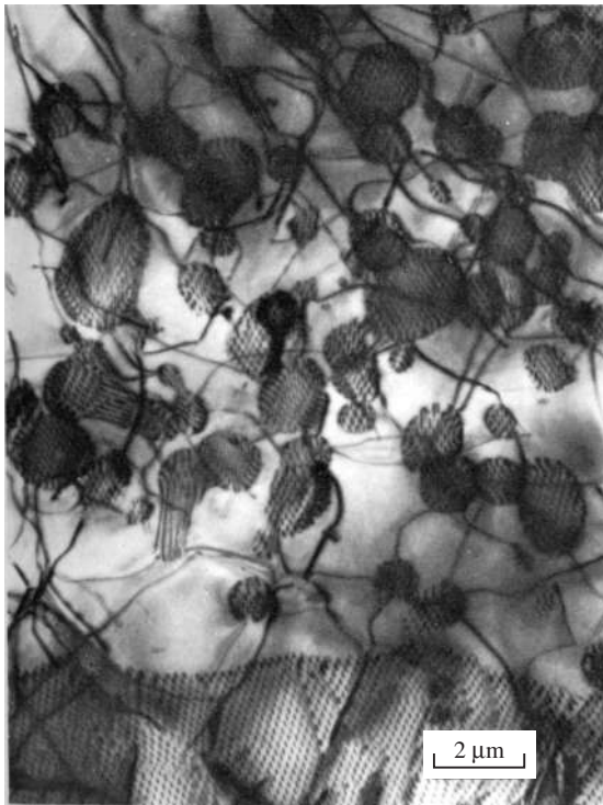
Fig. 6.13 TEM image showing small lenticular inclusions of hematite in ilmenite from Bancroft, Ontario, with misfit dislocations decorating the boundary between hematite and ilmenite regions. The larger dark lines are normal dislocations in ilmenite (from Lally et al. , 1976).
