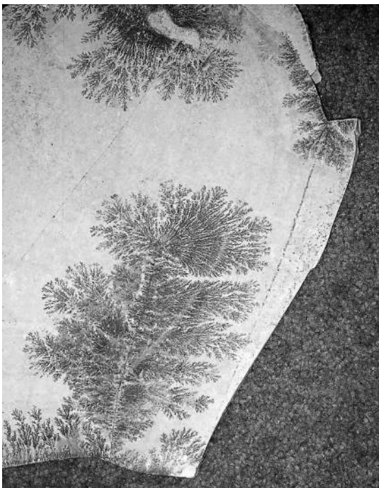
Fig. 5.10 Dendritic growth of manganese oxides ( \text{MnO}_2 ) on bedding planes of Solnhofen limestone (Germany). Growth initiates from fractures (width 55 mm) (courtesy E.H. Wenk).
