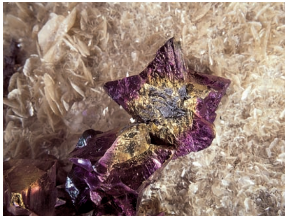
(d) Chalcopyrite with typical oxidation colors on siderite from Wilroth, Westerwald, Germany (courtesy O. Medenbach). (Width 36 mm.)
