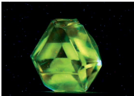
(b) Synthetic diamond imaged when exposed to a high intensity synchrotron X-ray beam, producing yellow optical luminescence and corresponding reflections (courtesy A. Freund, see also Hozzowaska et al. , 2001). (Diameter 10 mm.)
