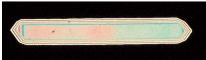
(d) Interference colors observed on a quartz prism. In the microscope the c -axis of the crystal was at 45^\circ (NW-SE). Crossed polarizers.
