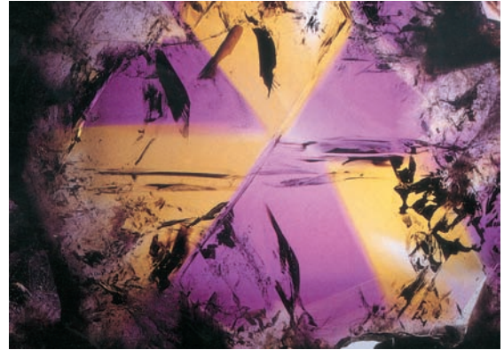
(d) Sector zoning in the quartz variety ametrine from the Anahi mine in Bolivia, with purple sectors of amethyst (Fe-poor, yellow citrine (Fe-rich). Displayed is a section cut through the tip of a crystal (courtesy M. Weibel). (Width 40 mm.)
