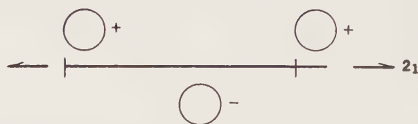
2-fold screw axis parallel to b
