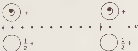
Glide plane with glide component parallel to c ; plane parallel to (100)
