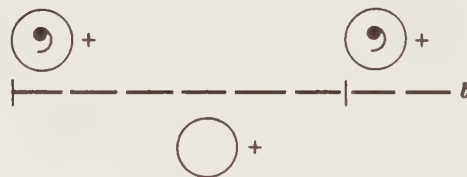
Glide plane with glide component parallel to b ; plane parallel to (100)
