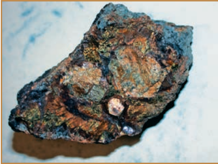
Chalcopyrite is a copper iron sulfide mineral that crystallizes in the tetragonal system. Chalcopyrite is one of the most important copper ores. (Photo courtesy of Nature's Images)
