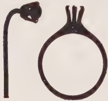
FIG. 472.—X-ray photograph of lead-glass imitation (pin) and of diamond (ring).
