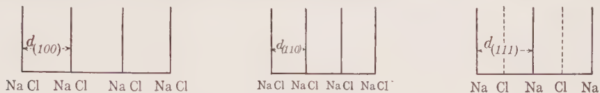
FIG. 430.—Relative distances between successive layers of atoms in halite (NaCl) parallel to faces of the cube (100), rhombic dodecahedron (110), and octahedron (111), respectively.
