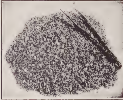
FIG. 482.—Bortz suitable for diamond drills.
