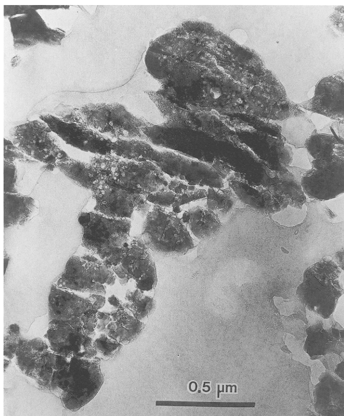
Fig. 9. Transmission electron micrograph of an ultrathin section of chondritic IDP L2011K7 embedded in epoxy (gray background) showing fusion of subspherical (carbon-free) ferromagnesio-aluminosilica (very low \text{Al}_2\text{O}_3 ) units with ultrafine-grained Mg, Fe-olivines and pyroxenes and iron oxides. The shattered appearance is an artifact of ultramicrotome sectioning
