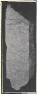
FIG. 648.—Orthoclase showing rectangular cleavage.
