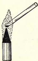
FIG. 392.— Heating in closed tube.
