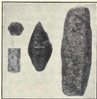
FIG. 490.—Corundum crystals—tabular, prismatic, pyramidal, long prismatic.
