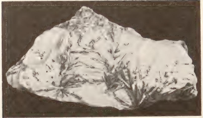
Fig. 66. The radiate aggregates of antimonite crystals in a quartz vein. (Half the size)
