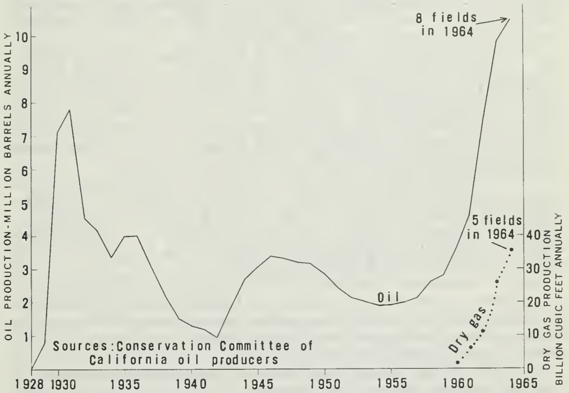
FIGURE 59. Offshore oil and dry gas production in Ventura sedimentary basin, California.
