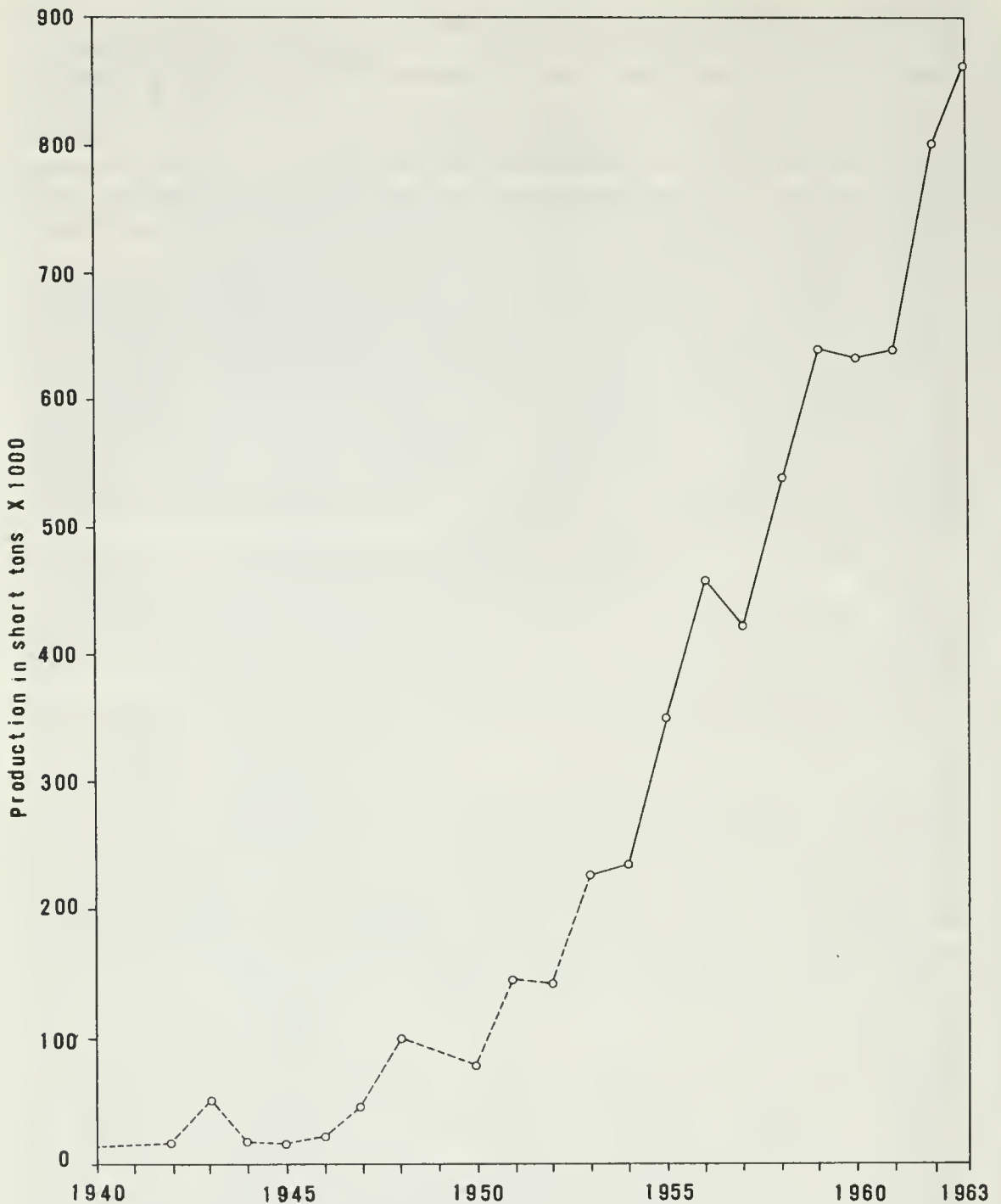
FIGURE 71. Annual production of expanded shale aggregate in California (figures prior to 1953 are approximate due to incomplete statistics).
