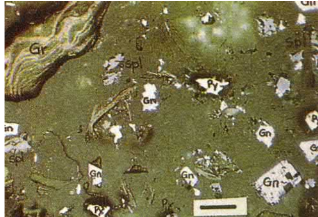
FIGURE 13.8 Final milling completes the liberation of free sphalerite, galena, pyrite, graphite, and gangues, ready for froth flotation or any suitable process.
