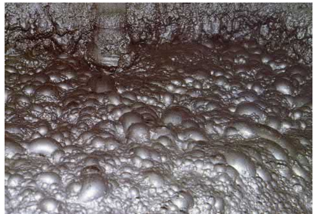
FIGURE 13.36 Formation of mineralized froth (lead concentrate) from an active flotation cell and that subsequently moves to lead cleaner, and concentrate stockpile.
