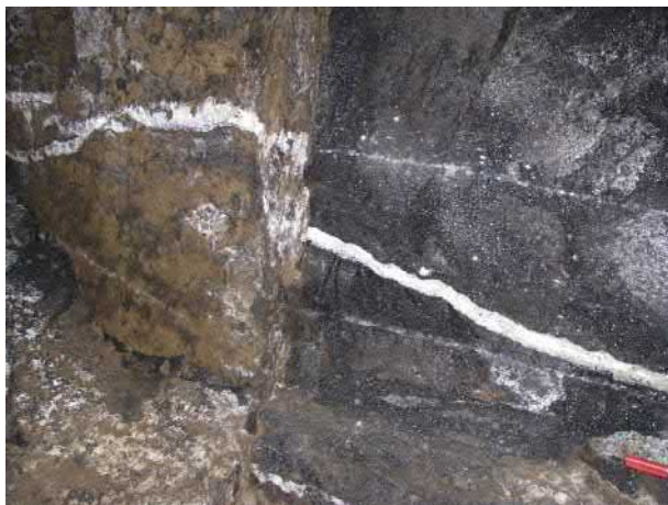
FIGURE 2.4 Massive chromite lode depicting sharp faulted contact with barren ultramafic rock, Kathpal underground mine, Sukinda belt, India.
