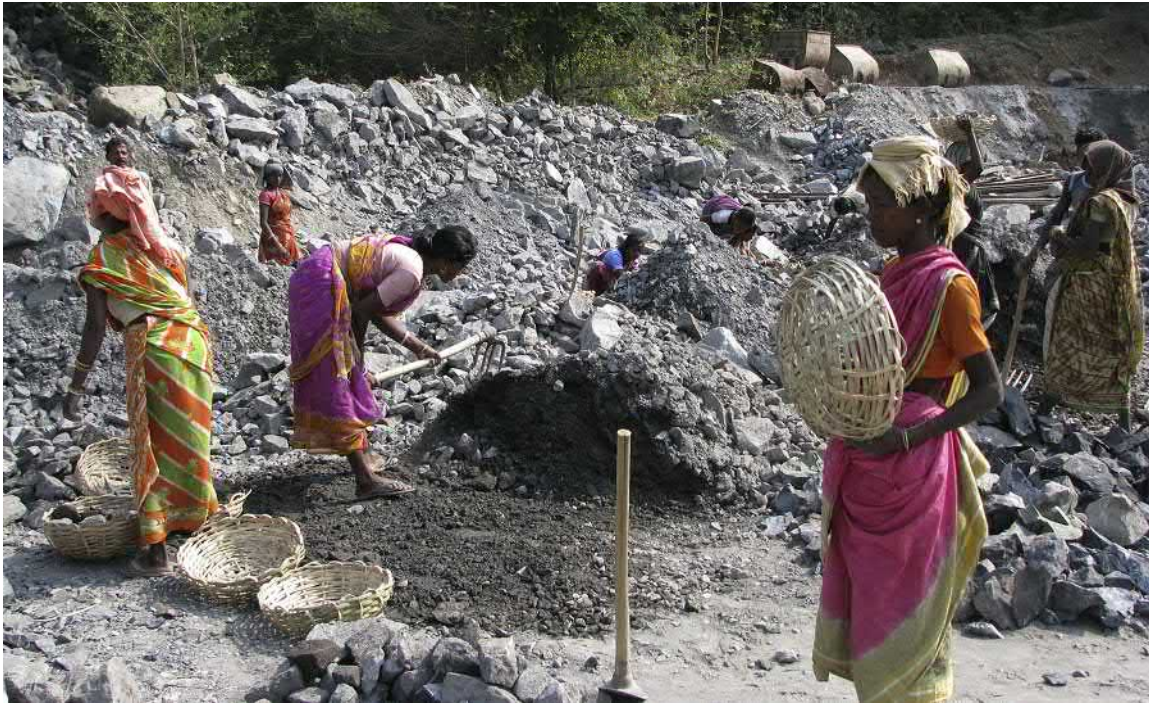
FIGURE 13.26 Hand sorting and commercial sizing by manual works at low cost in small-scale mining operation at Nausahi chromite mine, India.
