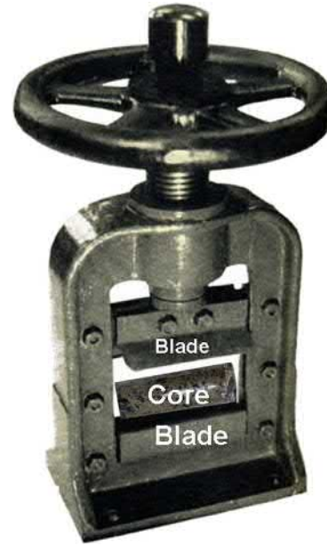
FIGURE 7.26 Semimechanical core splitter used at Khetri copper mine during the 1970s.
