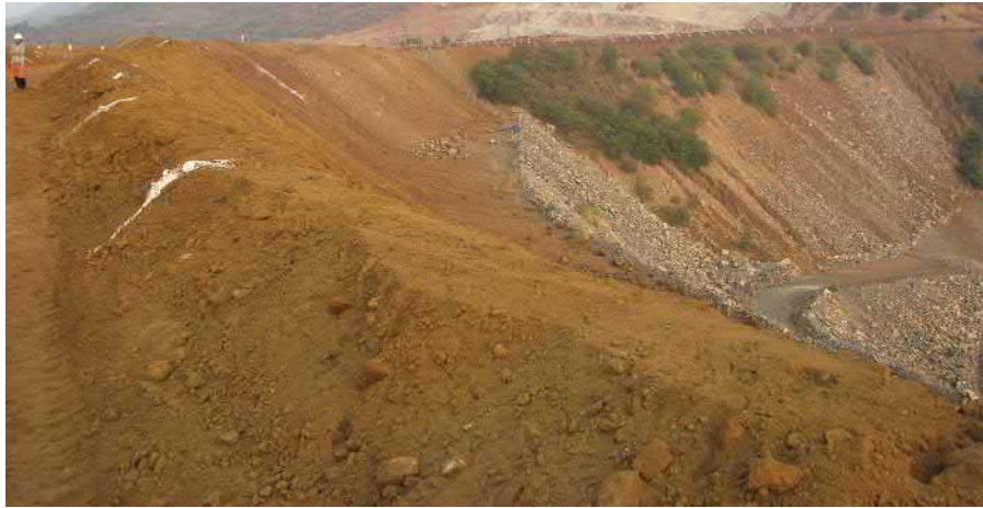
FIGURE 5.5 The older ultramafics have been extensively weathered to form laterite (yellow and red limonite) at the top of Sukinda intrusion. The nickel-bearing laterite has complex metallurgy for economic recovery and is stacked separately for future technology update.
