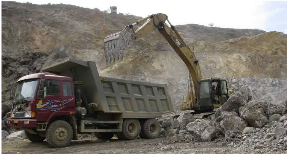
FIGURE 12.40 Hydraulic large shovel mucking and loading and 85-t Haulpac dumper at Jhamarkotra rock phosphate open pit mine, Rajasthan, India (December 2008).
