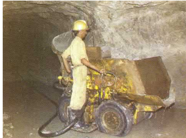
FIGURE 12.36 Compressed air-driven four-wheel drive Cavo loaders on four extra rubber-molded tires with 1\text{ m}^3 capacity are useful in small-scale underground mine transportation.
