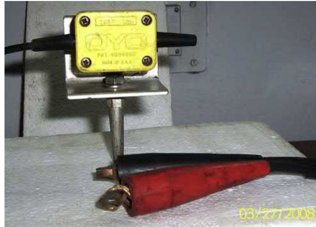
FIGURE 6.8 A three-component vertical 14 Hz “geophone” device for detection and recording of seismic reflection and refraction from subsurface interface.
