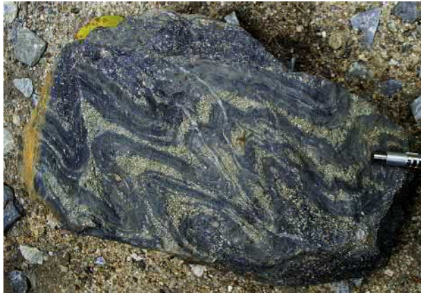
FIGURE 2.3 Stratiform pyrite-zinc-lead mineralization folded with mineral concentration at crests presenting saddle reef structure, Rajpura-Dariba deposit, India.
