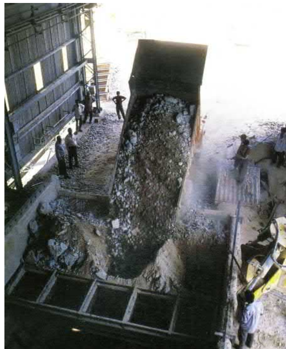
FIGURE 13.18 Run-of-mine ore is transported to a beneficiation plant and uploaded on a grizzly separator for preventive screening before feeding to a primary crusher.
