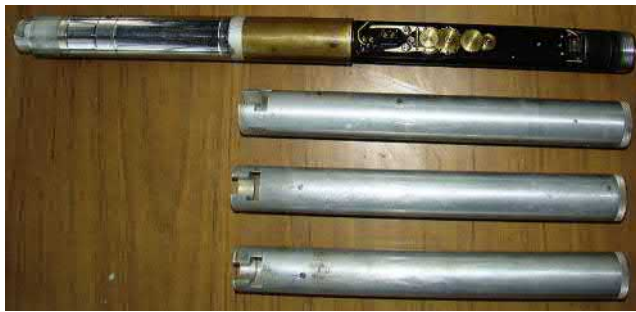
FIGURE 7.16 Borehole survey by reflex multishot camera is ideal for measuring both angle and azimuth with highest precision for holes at a number of depths at one lowering—a total borehole survey solution.
