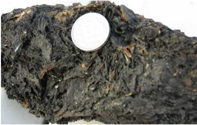
FIGURE 5.7 The dark chocolate color, crust radiate structure, and diamond mesh cellular box work of a unique gossans formation above Rajpura-Dariba deposit indicate the presence of galena and tetrahedrite underneath.
