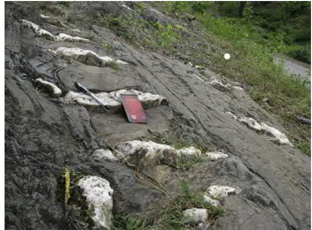
FIGURE 2.11 Quartz-filled ladder vein structure in compact dolomite mass at the footwall of main lodes within greywacke rocks, Zawar group of mines, India.
