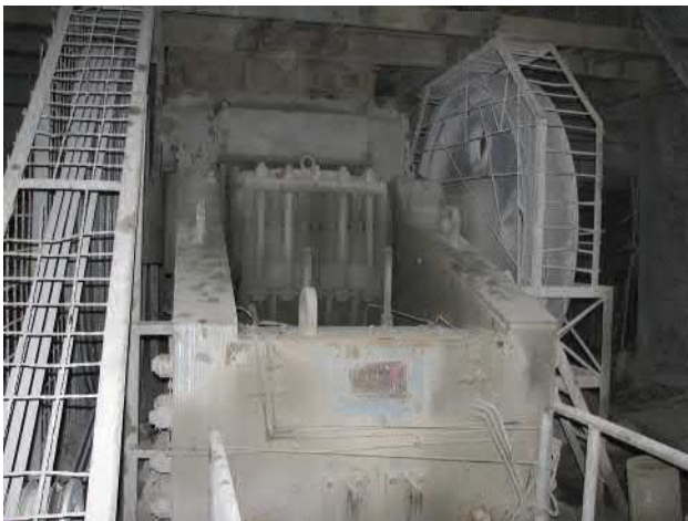
FIGURE 13.10 Medium-sized jaw crusher in operation in underground mine for crushing run-of-mine (ROM) ore before transferring to the surface.
