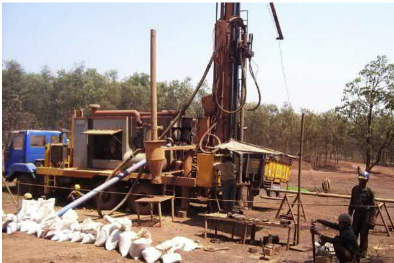
FIGURE 7.13 Reverse circulation drilling in operation and sample collection for iron ore deposits.
