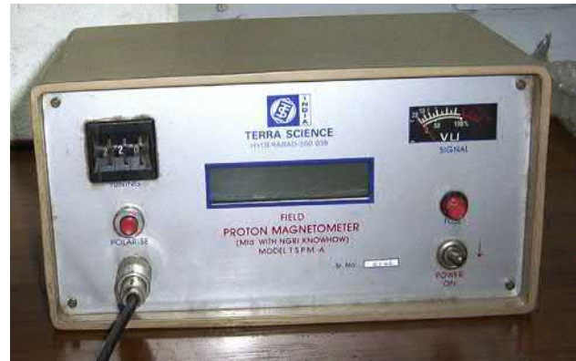
FIGURE 6.13 User-friendly proton magnetometer device compatible to high-end processing with precision.
