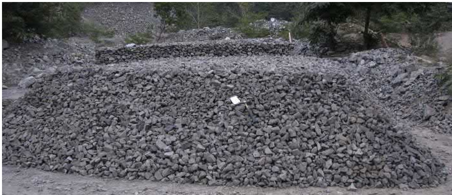
FIGURE 13.2 Screen-sorted chromite ore stockpiles of different specifications for direct sale and transportation to a ferrochrome plant.
