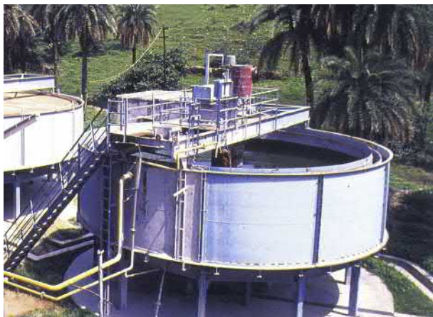
FIGURE 13.48 A view of a thickener with a rake mechanism in the first phase of dewatering of concentrate by sedimentation or gravity settling of solids.
