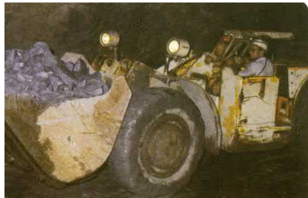
FIGURE 12.37 Diesel/compressed air-driven 1.5\text{ m}^3 load-haul-dump machine transporting the broken ore from working stopes to loading points.
