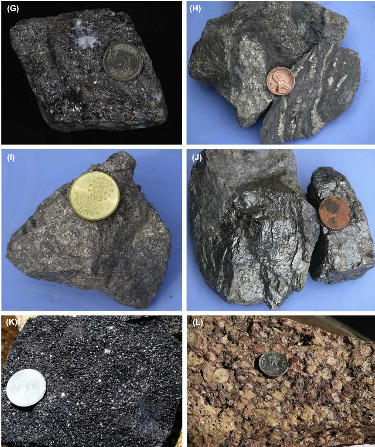
FIGURE 1.2, cont'd (G) brown sphalerite (Zawar, India), (H) stratiform pyrite in graphite schist (Rajpura-Dariba, India), (I) massive pyrrhotite (Sindesar-Khurd, India), (J) wolframite (Degana, India), (K) crystalline chromite (Sukinda, India), (L) pisolite structure in bauxite (Bagru Hill, Jharkhand, India)
