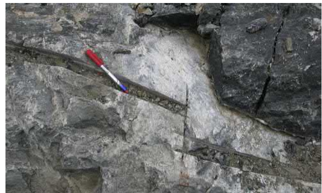
FIGURE 7.24 Channel sample cut by pneumatic drill machine for exploration of platinum-group elements at open pit bench face, Boula-Nausahi chromite mine, Orissa, India.
