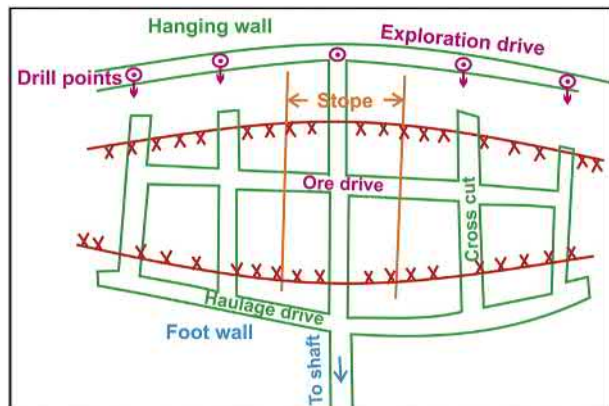
FIGURE 12.13 Schematic level diagram showing the various drives, cross-cuts, and mining stopes and their purposes.
