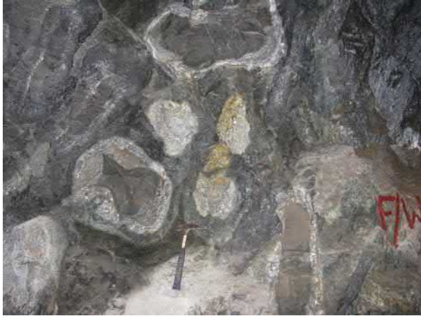
FIGURE 2.7 Irregular fragmented chromite (black with white rims) in matrix of Pt–Pd-bearing gabbro from the tectonic breccia zone, Boula-Nausahi underground mine, Orissa, India.
