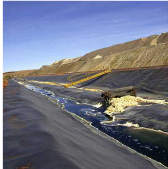
FIGURE 13.25 Copper heap leaching at Whim Creek, Philbara, Australia (Halдар, 2013).
