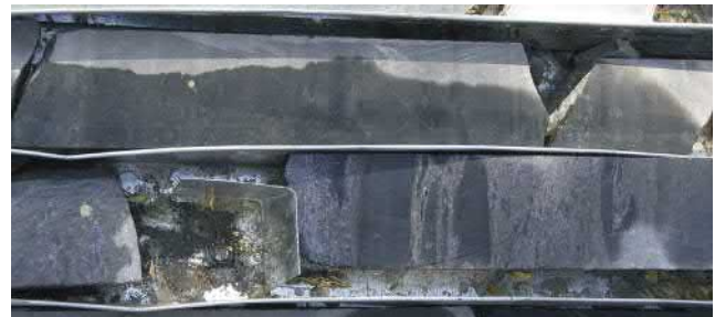
FIGURE 7.28 Stratiform sulfide drill core split into two identical halves by electric core cutter.
