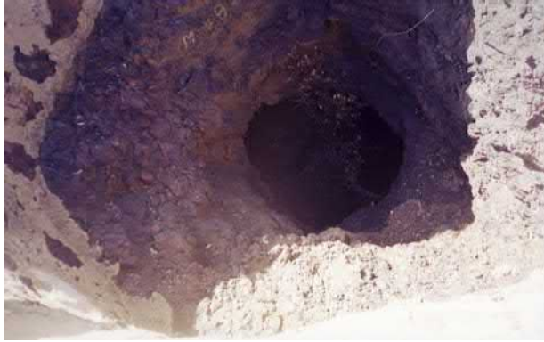
FIGURE 4.1 Ancient entry system to underground mine at shallow depth of orebody without any plunge during the 3rd–2nd millennium BC at Khetri copper belt, Rajasthan, India.
