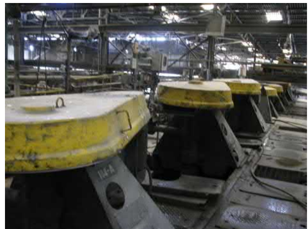
FIGURE 13.38 A typical bank of flotation cells in an operating circuit.
