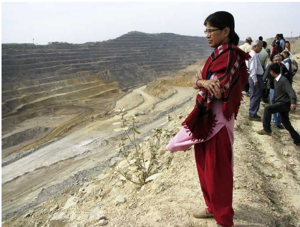
FIGURE 15.33 Entire stretch of A and D block at Jhamarkotra phosphate deposit has been mined for a vertical height of 400 m, and has reached the ultimate open pit mine bottom. A group of geoscientists assembled on a mine visit.
