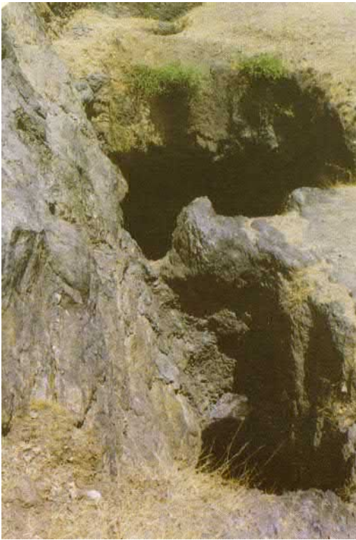
FIGURE 4.2 Ancient entry system to underground mine at greater depth with orebody plunge to northeast at Rajpura-Dariba copper-zinc-lead-silver mine, India.
