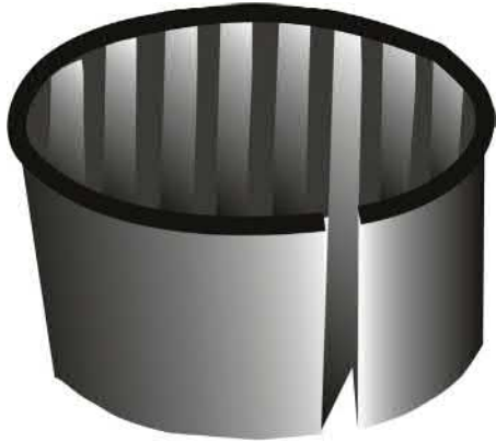
FIGURE 7.9 Standard spring-type core lifter that protects the core from slipping into the hole and regrinding.
