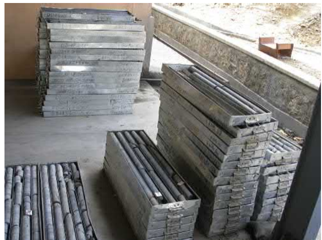
FIGURE 7.17 Standard wooden, plastic, and metallic (aluminum) core boxes essential for drill core preservation.
