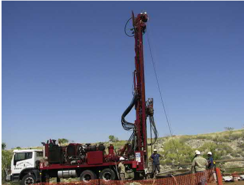
FIGURE 7.6 Truck-mounted diamond drill rig in operation for base metal exploration in Australia. The device is capable of drilling 50–100 m a day.
