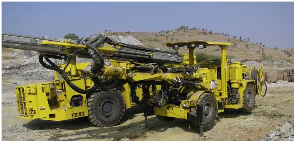
FIGURE 12.31 Single boom jumbo drill with basket diesel-powered articulated chassis with permanent four-wheel drive.
