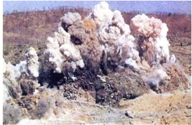
FIGURE 14.6 Open pit mine blasting of rock phosphate, India, generates toxic/nontoxic gases harmful to any living entity. The effect is controlled by better quality explosives, blasting between shift intervals, and nonexposure of miners to gas.
