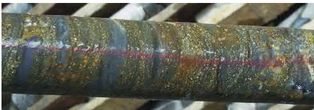
FIGURE 7.10 Standard drill core showing stratiform sphalerite and galena in calc-silicate host rock with the red pencil line marked for splitting into two near-identical halves at Rajpura-Dariba Mine, India.
