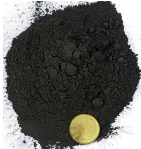
FIGURE 13.40 Dry lead concentrate with grade up to 65% Pb is achieved based on feed quality.
