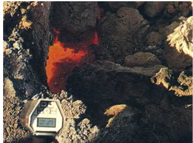
FIGURE 14.4 Coal mine fire is a common phenomenon in open pot and underground mines due to the burning of natural gases and temperature recorded by infrared gun at Jharia coalfields, India.
