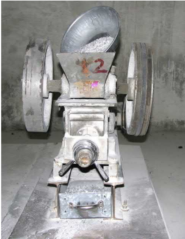
FIGURE 7.33 Sample grinding by a laboratory-scale small roll crusher.
