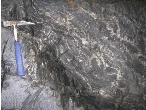
FIGURE 2.12 Stock work formed by stratification and stringers of sphalerite, galena, and pyrite hosted by carbonaceous calc-silicate rock at Sindsar-Khurd orebody, India.
