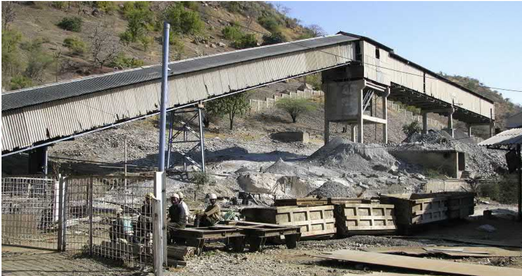
FIGURE 13.3 Close conveyor system (top) transporting run-of-mine (ROM) ore automatically unloaded from shaft cage to ore bin, and interim stockpiles (right) with chutes (bottom) for autofeeding to the mineral process plant.
