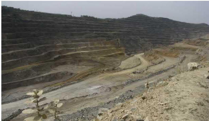
FIGURE 12.6 View of Jhamarkotra rock phosphate mine with haulage road and series of overburden benches. The mine is planned to be 7 km long, 700 m wide, and 280 m with an ultimate open pit limit of 2 Mt ore and 16 Mt overburden waste per annum capacity (December 2008).
