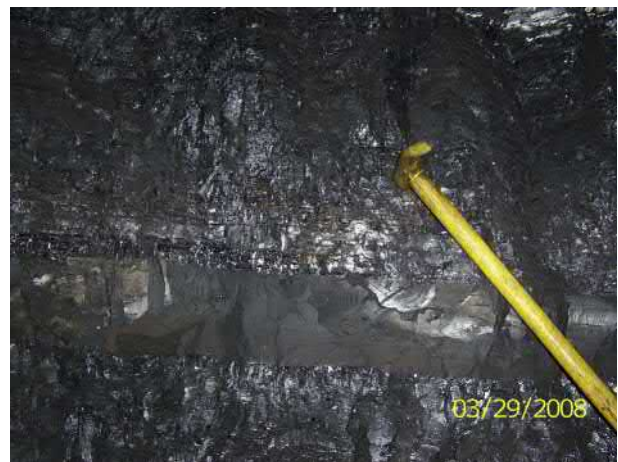
FIGURE 2.14 Alternate bands of coal (shining black color) and shale (brownish-gray), Belatan mine, Jharia coalfield, India.
