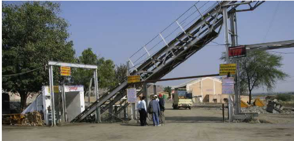
FIGURE 12.8 Mine entry systems by incline at a moderately steep angle of \sim 30 degrees to reach the orebody at the shortest distance, primarily preferred during exploration to confirm ore characteristics and sample for beneficiation test works.
