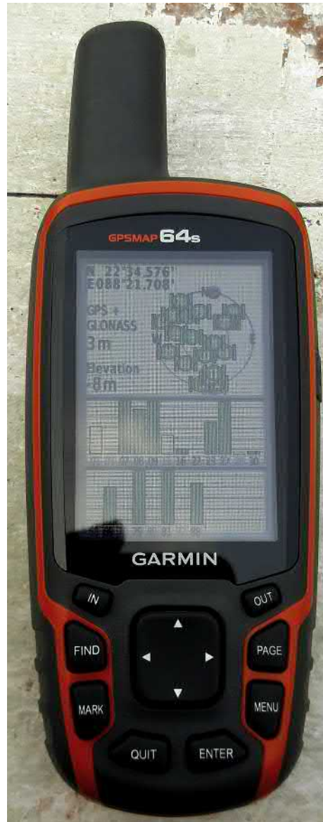
FIGURE 3.14 Hand-held Geographical Positioning System (GARMIN GPSMAP 64s) capable of measuring 3D coordinate system and trace the traverse path, rock contacts, structural features, and many more. Courtesy Prof. Sayad Rahaman.
