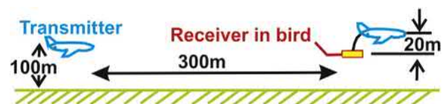
FIGURE 6.19 Schematic diagram showing electromagnetic aerial survey employing two airplanes.
