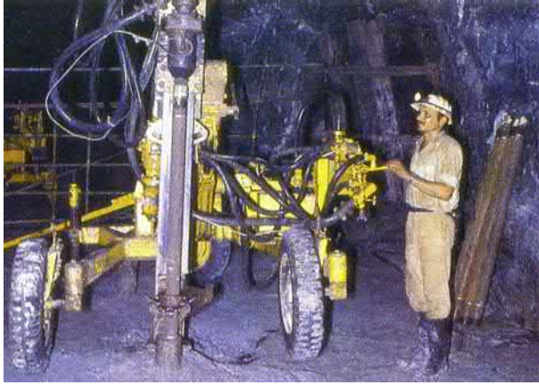
FIGURE 12.33 Tire-mounted down-the-hole hammer drill rigs in operation for drilling 60 m vertical height of vertical retreat mining stopes at Rajpura-Dariba mine during the 1990s.
