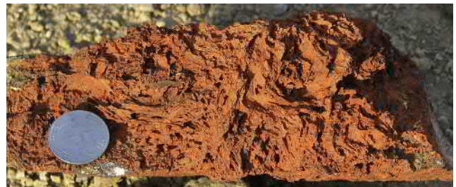
FIGURE 5.6 The yellow-brown color, cellular box work, and sponge structure of a unique gossans formation above Rajpura-Dariba zinc-lead-copper-silver deposit indicate the presence of sphalerite underneath.
