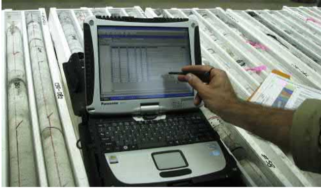
FIGURE 7.19 Tough book—a high-tech internet interfaced data-sharing drill core logger used at Lennard Shelf zinc deposit, Australia.
