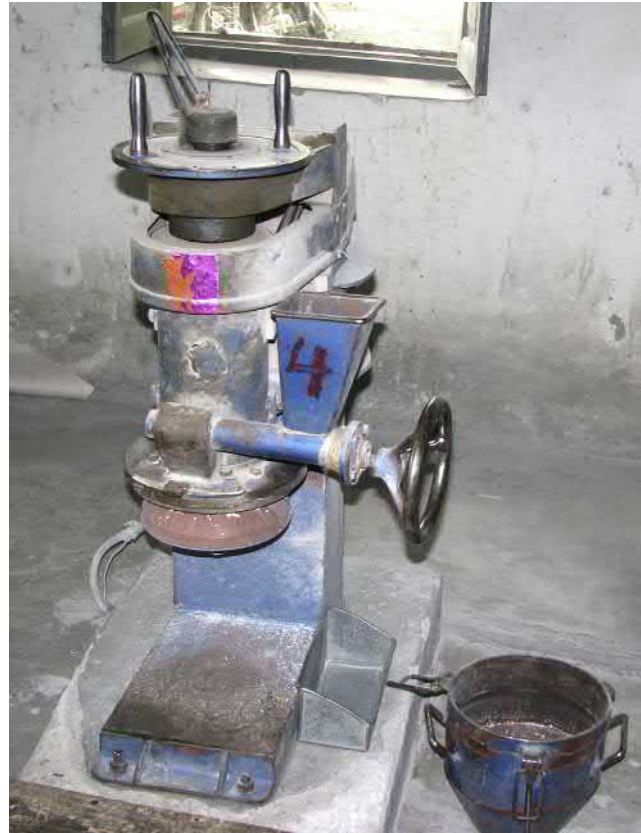
FIGURE 7.34 Sample size reductions by a laboratory-scale disc, ball, or rod pulverizer.
