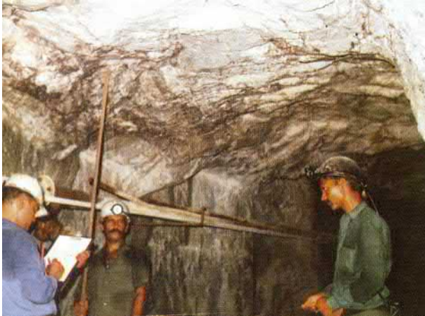
FIGURE 4.13 Scan line underground mapping of cross-cut at Balaria Mine, India.
