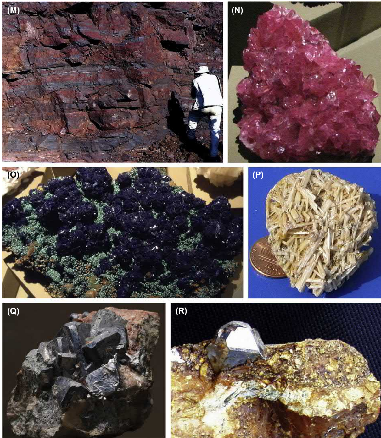
FIGURE 1.2, cont'd (M) hematite (steel gray) and jasper (red) (India), (N) rhodochrosite crystals with brilliant rose red color from South Africa, (O) azurite with distinct azure blue color is an excellent exploration guide, (P) cerussite or "white lead ore" (Megan, Germany), (Q) nickel-skutterudite (Schoenberg, Germany), (R) sperrylite crystal (~8 mm across) on weathered chalcopyrite mat (Broken Hammer deposit, Wallbridge Mining Co. Ltd., Sudbury Camp, Canada) (Dr. Tom Evans)
