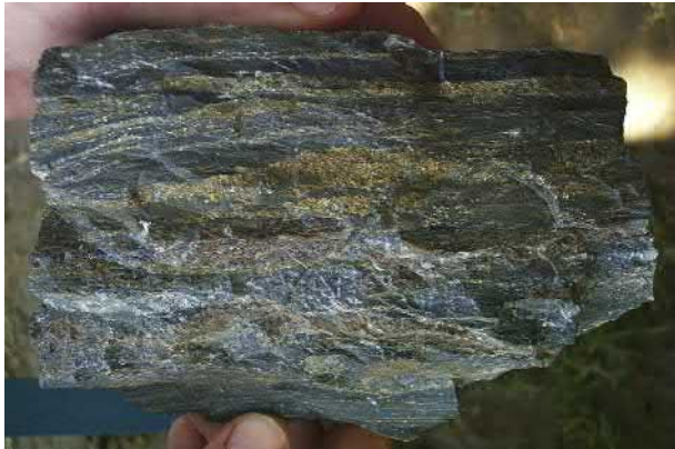
FIGURE 2.13 Stratiform sphalerite (honey-brown) mineralization in calc-silicate (bluish-gray) host rock at Rajpura-Dariba deposit, India.
