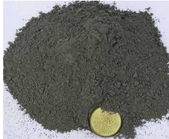
FIGURE 13.39 Dry zinc-lead ore grinded to 68% of -74 \mu m particle size to yield the highest liberation of ore and gangue minerals.
