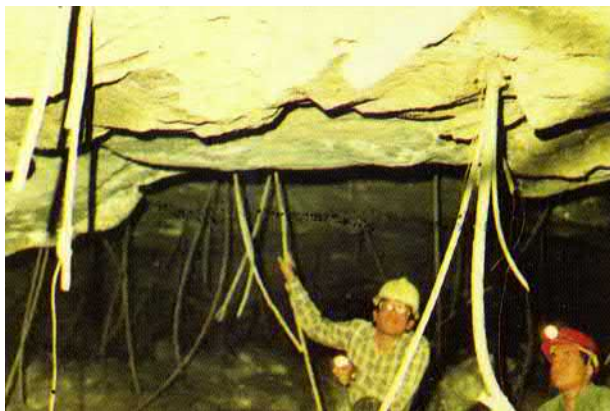
FIGURE 12.42 Cable bolting is suitable to bind large rock masses for extended periods and is adopted as an appropriate support system in bad ground.
