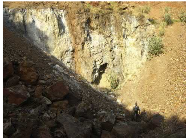
FIGURE 5.11 Part of the unique gossans collapsed in the eastern part of the hill during active underground mining operation leaving fresh exposure. Photo January 2010.
