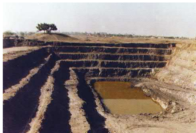
FIGURE 10.7 A surface pit was opened at the end of exploration, estimation, and project formulation to generate large volumes of representative samples for pilot plant metallurgical tests, and bench blast-hole sampling to compare with estimated block grades.
