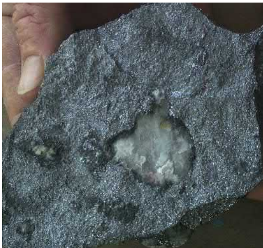
FIGURE 2.21 Massive fine-grained crystalline galena (shining gray color) and remnants of partially replaced quartz vein (white) at Rajpura-Dariba underground mine, India. The excessive fine grain size or over-grinding hinders better recovery. Courtesy: Prof. Martin Hale.
