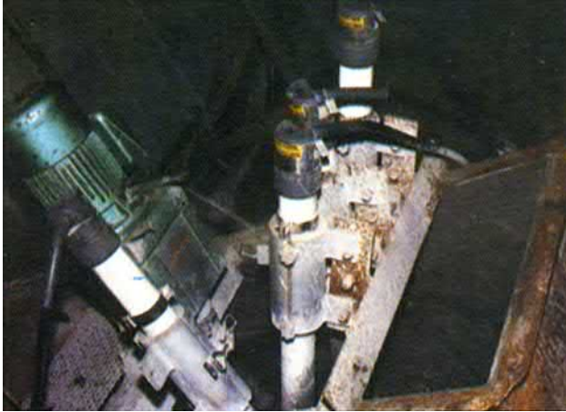
FIGURE 13.5 Mill sampling system by in-stream analyzer. The probe is installed in the slurry stream of feed (conditioner) and reject (tailing) for continuous sensing of metal grades and simultaneous digital process control of reagents.
