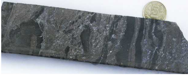
FIGURE 2.20 Massive sphalerite (iron-brown) and galena (shining) in carbonaceous calc-silicate host rock sedimentary exhalative deposition at Sindesar-Khurd SEDEX type in India.
