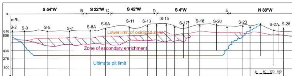
FIGURE 15.6 Composite longitudinal section along Malanjkhanda copper orebody showing the surface drilling interval and ultimate open pit bottom.
