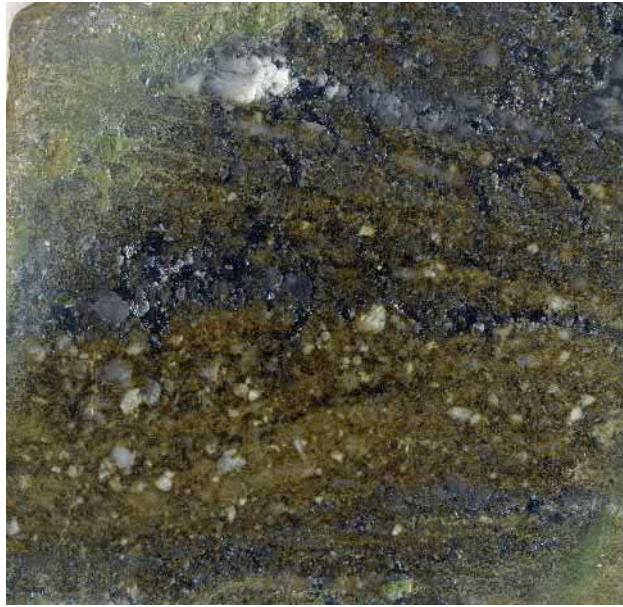
FIGURE 13.6 Camera image of polished surface of rich run-of-mine (ROM) ore showing yellow-brown sphalerite, gray-black galena, and gangue minerals (white calcite, dolomite, and quartz crystals).
