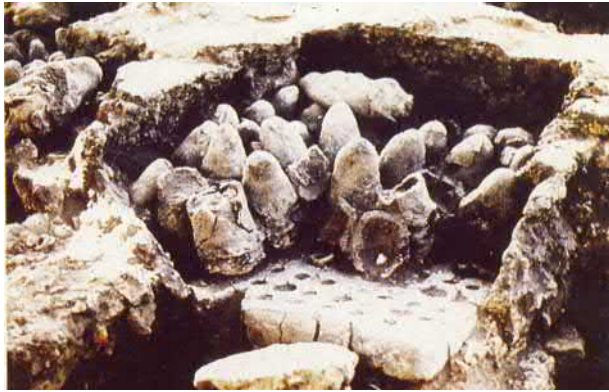
FIGURE 4.5 Ancient smelting furnace unearthed with 6 \times 6 numbers of retorts placed in an inverted position for distillation of zinc by a heating and condensation process at Zawar Mines, India, during 2180 \pm 35 years from today.
