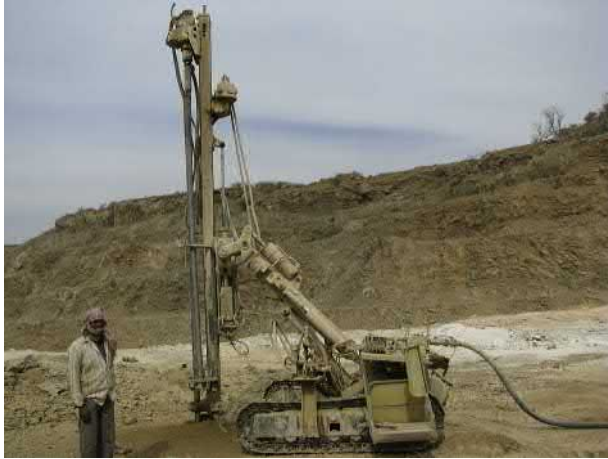
FIGURE 15.32 Robust crawler chain-mounted wagon drill in operation at Jhamarkotra rock phosphate mine, which drills at a 5–10 m bench height and is easy to move to hole sites.
