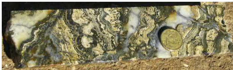
FIGURE 2.19 Sphalerite (yellow) and galena (black) mineralization in calcite (white) bands indicating different fluid phase events, Lennard Shelf MVT deposit, Western Australia.
