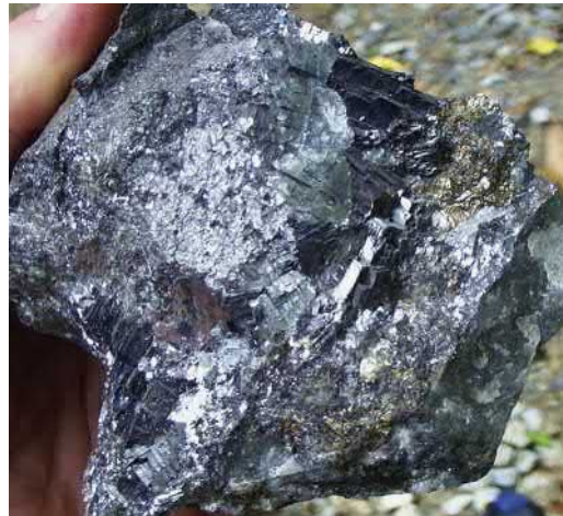
FIGURE 2.23 Coarse-grained galena crystal (shining gray color) with small patches of chalcopyrite (yellow) from SEDEX type of sulfide mineralization at Rajpura-Dariba underground mine, India. The sample is easiest to identify and unique in all respects. Courtesy: Prof. Martin Hale.
