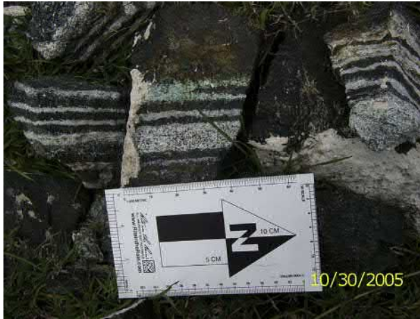
FIGURE 2.15 Layers of chromite (black) and Pt–Pd-bearing gabbro (white), Sittampundi Igneous Complex, Tamil Nadu, India.
