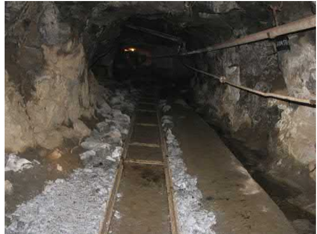
FIGURE 12.14 View of a main cross-cut starting from the central main shaft to the orebody at Boula-Nausahi chromite deposit, main production haulage (December 2009).
