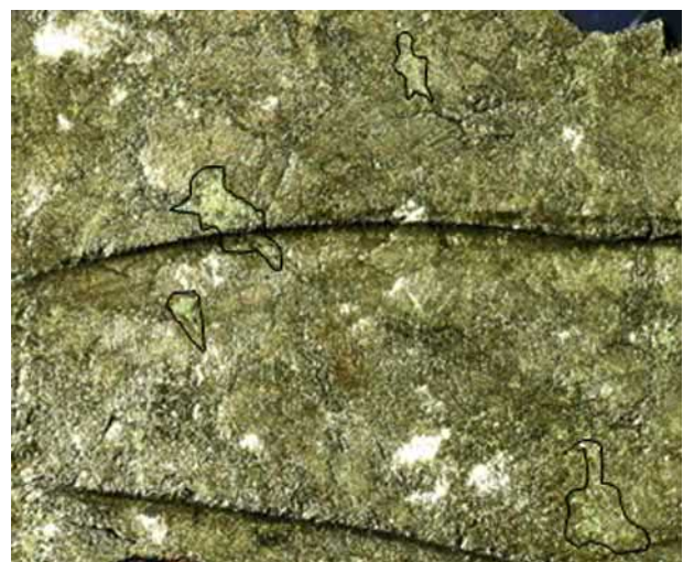
FIGURE 15.16 The nickel bearing massive pyrrhotite, and patches (black irregular boundary) of pentlandite \{(Fe, Ni)_8S_9\} are inter grown from the Trill “offset inclusion quartz dyke” associated with the Sudbury Complex, Canada. The other nickel mineral millerite (NiS) occurs as micro level inters grown type. Credit: Tom Evans.
