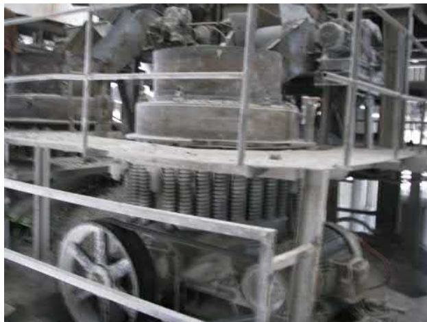
FIGURE 13.13 A working cone crusher in a mineral process plant operation, performing both secondary and tertiary crushing functions.
