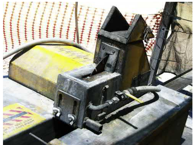
FIGURE 7.27 Fully mechanized electric core cutter used at Lennard Shelf zinc deposit, Australia.
