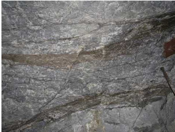
FIGURE 2.9 Sheeted veins and fine stringers of sphalerite in dolomite host rock at Zawar deposit, India.
