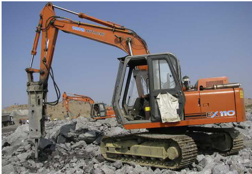
FIGURE 12.34 Crawler-mounted (continuous tracks) hydraulic hammer-type rock breaker in operation to break large-sized stones of run-of-mine ore at Sindesar-Khurd mine, Rajasthan, India.
