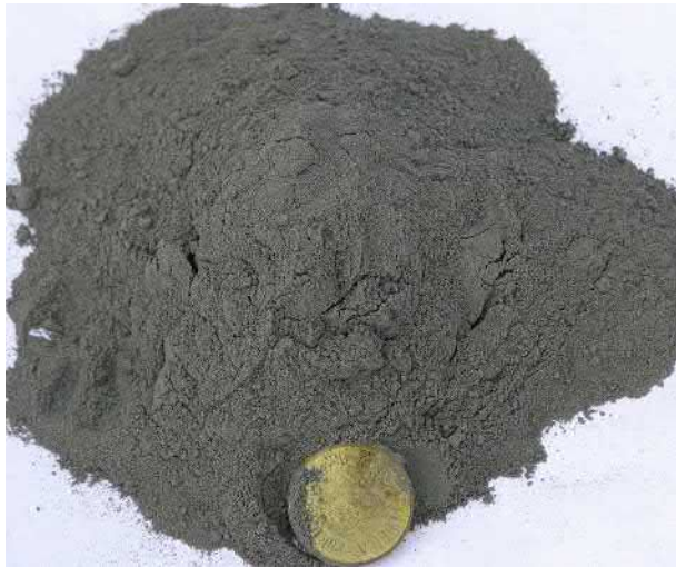
FIGURE 13.42 Dry tailing from a Zn-Pb process plant with grade around 0.20% Pb; 0.50%–1.00% Zn is lost based on feed quality.
