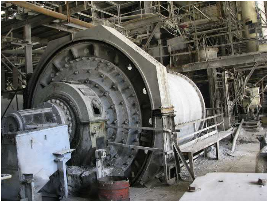
FIGURE 13.17 Standard grinding ball mill plays a significant role in completing the liberation of ore and gangue minerals. It is in operation at Zawar Mine, India.
