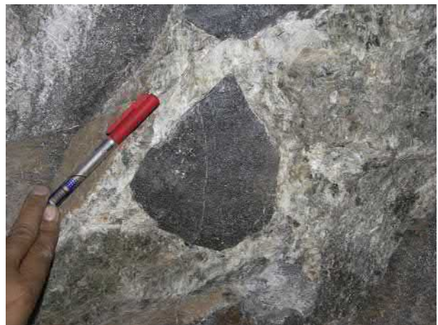
FIGURE 2.6 Pt-Pd-bearing magma (greasy white color gabbro) around sharp-angle chromite (black) from the tectonic breccia zone, Boula-Nausahi underground mine, Orissa, India.
