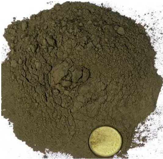
FIGURE 13.41 Dry zinc concentrate with grade up to 55% Zn is achieved based on feed quality.
