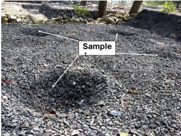
FIGURE 7.22 Stack sampling of chromite mine production ore at Sukinda belt, India.
