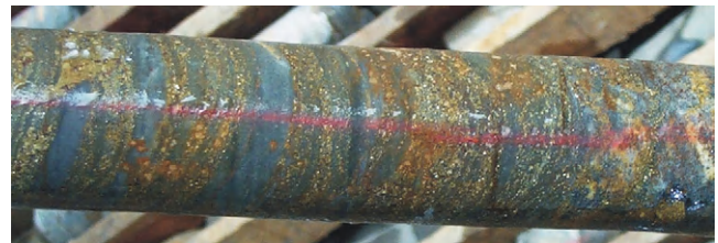
FIGURE 7.10 Standard drill core showing stratiform sphalerite, galena in calc-silicate host rock with red pencil line marked for splitting into two near-identical halves at Rajpura-Dariba Mine, India.
