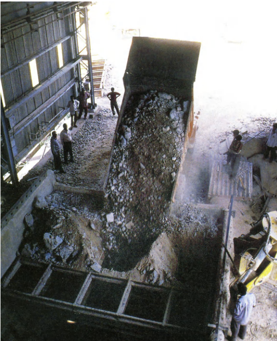
FIGURE 12.18 ROM ore is transported to beneficiation plant and uploaded on Grizzly separator for preventive screening before feeding to primary crusher.
