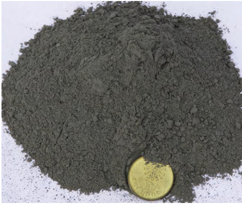
FIGURE 12.41 Zinc-lead ore grinded to 68% of -74\ \mu\text{m} particle size to yield highest liberation of ore and gangue minerals.
