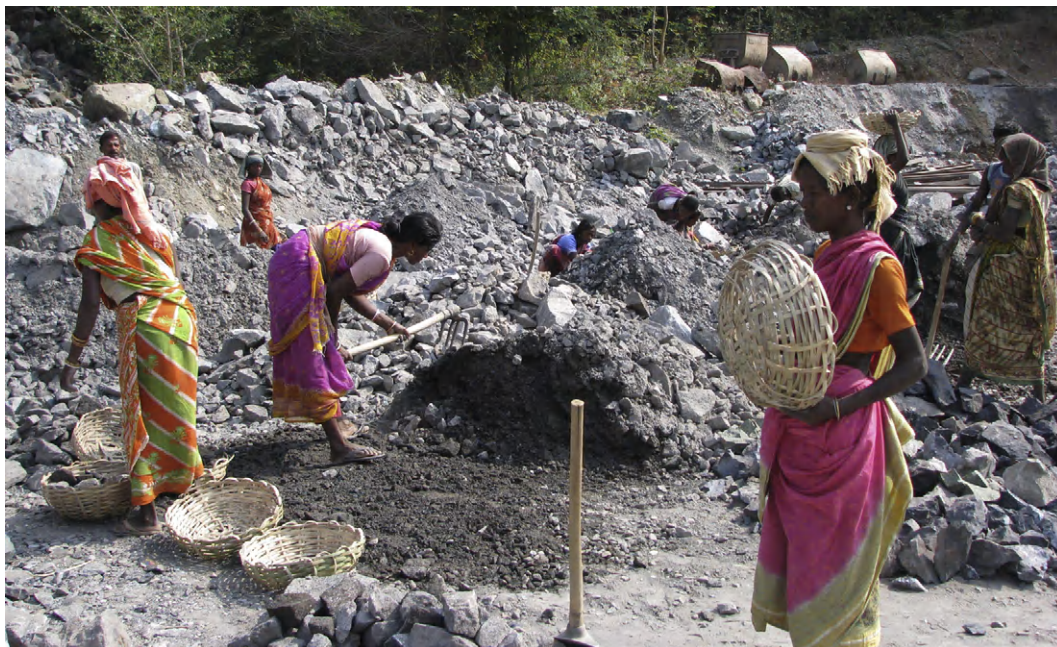
FIGURE 12.26 Hand sorting and commercial sizing by manual works at low cost in small-scale mining operation at Nausahi chromite mine, India.
