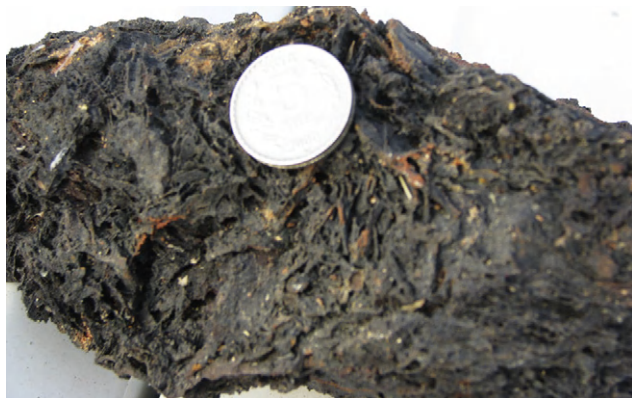
FIGURE 4.5 The dark chocolate color, crust radiate structure and diamond mesh cellular box work of unique gossans formation above Rajpura-Dariba deposit indicate presence of galena and tetrahedrite underneath.
