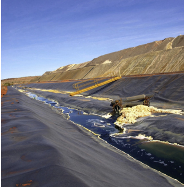
FIGURE 12.25 Copper heap-leaching at Whim Creek, Philbara, Australia (Credit: Dr Tim Sugden, Venturix Resources Limited, Australia).
