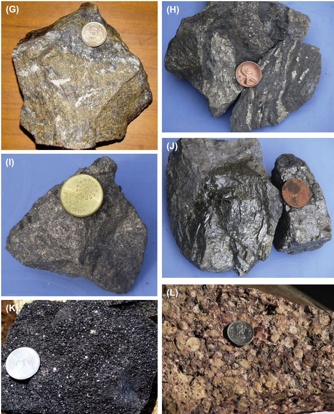
FIGURE 1.3 G-L Common ore minerals: (G) honey yellow sphalerite, (Rajpura-Dariba, credit: V. K. Jhanjhri), (H) stratiform pyrite in graphite schist (Rajpura-Dariba), (I) massive pyrrhotite (Sindesar Khurd), (J) wolframite (Degana mine, India), (K) crystalline chromite (Sukinda, India), (L) pisolitic structure in bauxite (Bagru Hill, Jharkhand, India).
