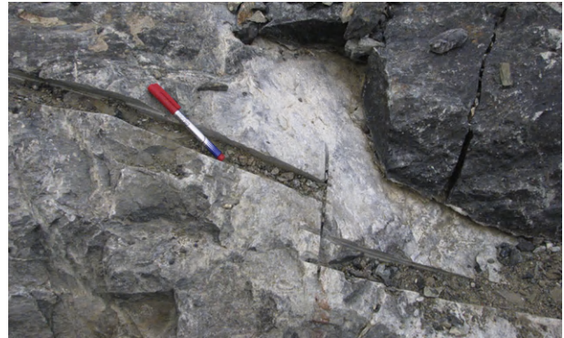
FIGURE 7.24 Channel sample cut by pneumatic cutter for exploration of platinum group of elements at open pit bench face, Boula-Nausahi chromite mine, Orissa, India.
