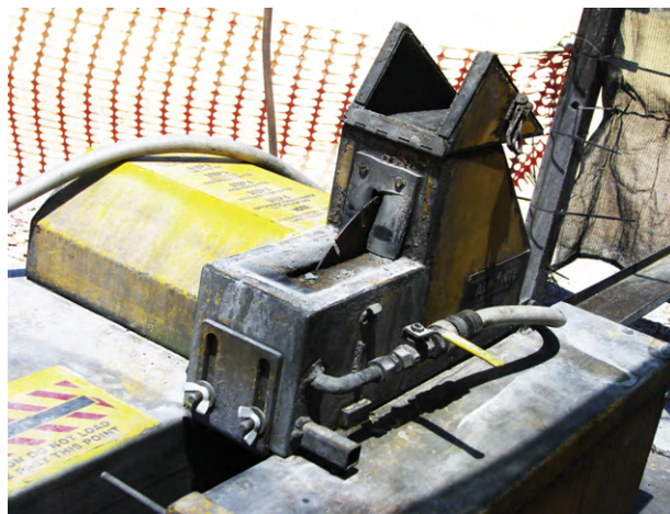
FIGURE 7.27 Fully mechanized electric core cutter being used at Lennard Shelf Exploration Camp, Australia.
