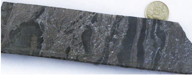
FIGURE 2.16 Massive sphalerite (iron brown) and galena (shining) in carbonaceous calc-silicate host rock sedimentary exhalative deposition at Sindesar Khurd SEDEX type in India.
