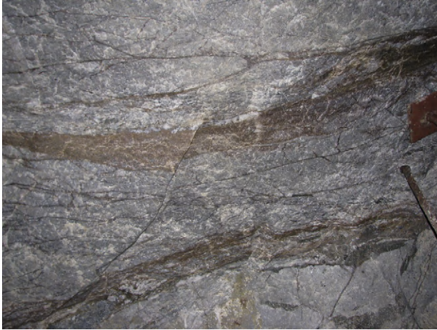
FIGURE 2.8 Sheeted veins and fine stringers of sphalerite in dolomite host rock at Zawar deposit, India.
