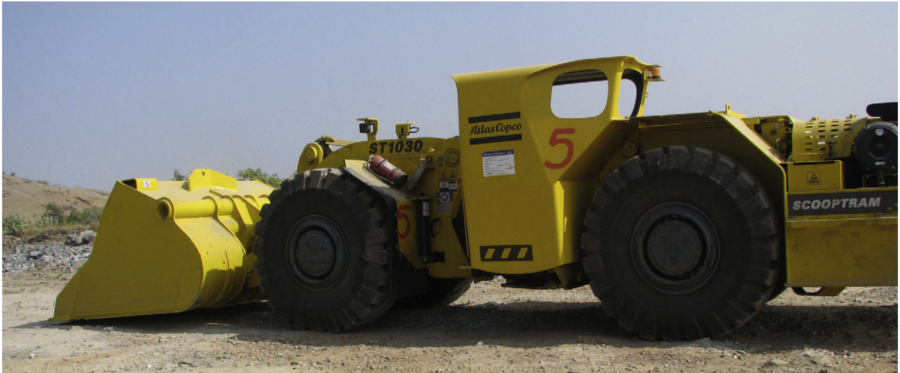
FIGURE 11.38 Electric-powered radio remote control operation of 2.7 m 3 capacity.
