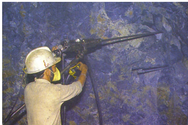
FIGURE 7.3 Jackhammer drilling in rich sulfide mineralization for multipurpose use as underground mine face development and sample source for ore continuity and grade control.
