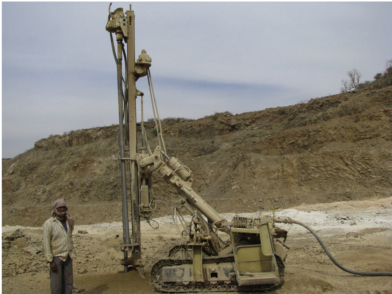
FIGURE 11.29 Robust crawler chain-mounted Wagon drill in operation at Jhamarkotra rock-phosphate mine to drill 5-10 m bench height and easy movement to hole sites.
