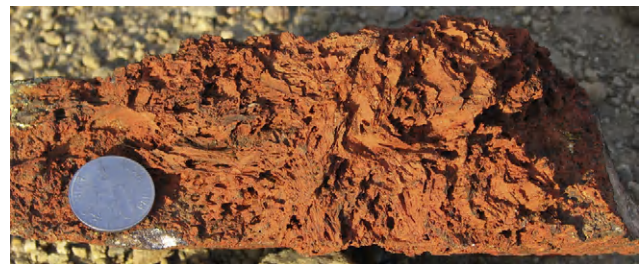
FIGURE 4.4 The yellow-brown color, cellular box work and sponge structure of unique gossans formation above Rajpura-Dariba zinc-lead-copper-silver deposit indicate presence of sphalerite underneath.
