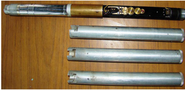
FIGURE 7.16 Borehole survey by reflex multishot camera competent to measure both angle and azimuth with highest precision for several depth of hole at one lowering—a total borehole survey solution (Credit: Vinod Jhanjari).
