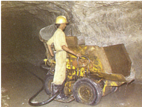
FIGURE 11.36 Compressed air-driven four-wheel drive “CAVO loaders” on four extra rubber molded tires with 1 m 3 capacity are useful in small-scale underground mine transportation.
