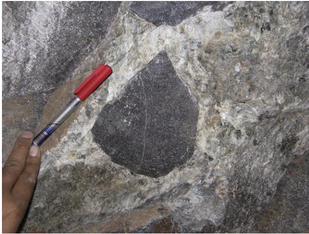
FIGURE 2.11 Stock work of Pt-Pd-bearing magma (greasy white color gabbro) around sharp-angle chromite (black) from the tectonic breccia zone, Boula-Nausahi underground mine, Orissa, India.
