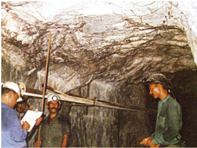
FIGURE 3.12 Scan line underground mapping of crosscut at Balaria mine, India.
