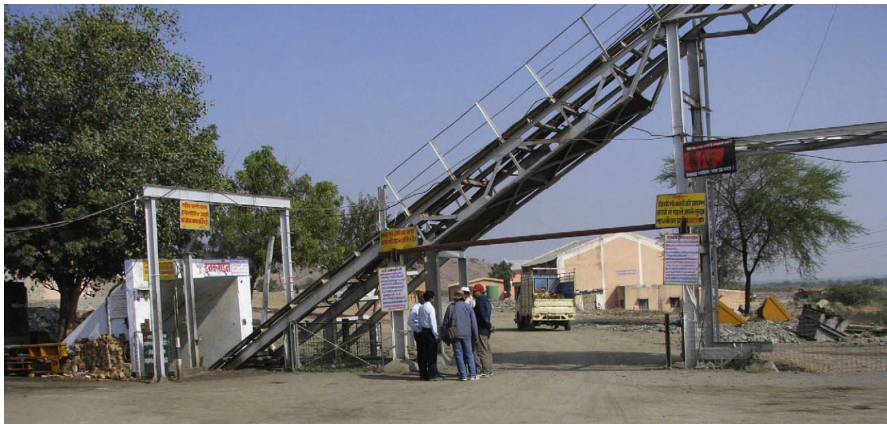
FIGURE 11.8 Mine entry systems by incline at a moderately steep angle \sim 30^\circ to reach the orebody at shortest distance, primarily preferred during exploration to confirm ore characteristics and sample for beneficiation test works at Sindesar Khurd Project, India.
