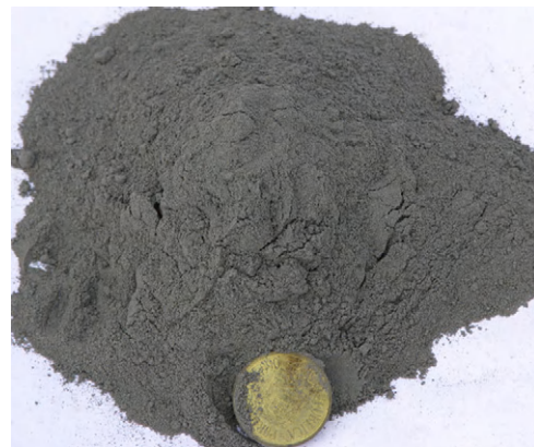
FIGURE 12.44 Tailing from Zn-Pb process plant with grade around 0.20% Pb and 0.50-1.00% Zn is lost based on feed quality.
