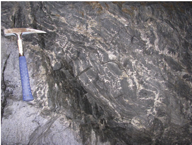
FIGURE 2.9 Stratification and stringers of sphalerite, galena and pyrite hosted by carbonaceous calc-silicate rock at Sindesar Khurd orebody, India.
