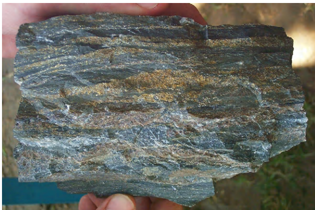
FIGURE 2.12 Stratiform sphalerite (honey brown) mineralization in calc-silicate (bluish gray) host rock at Rajpura-Dariba deposit, India.
