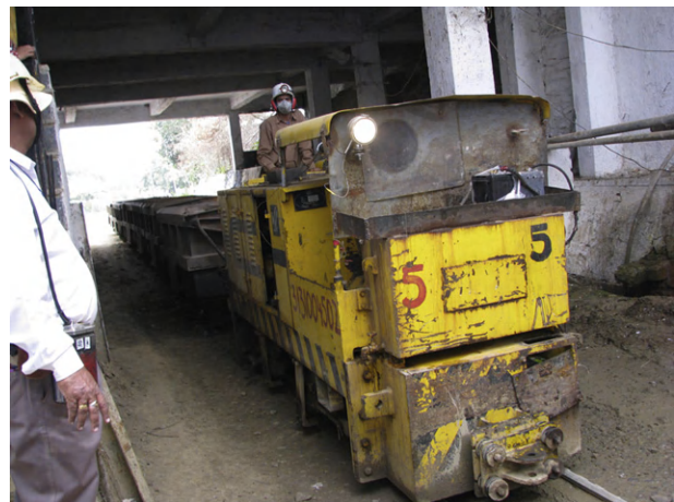
FIGURE 7.30 Car sample in underground mine by collecting handful of ore randomly from moving mine cars.
