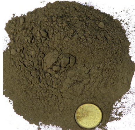
FIGURE 12.43 Zinc concentrate with grade up to 55% Zn is achieved based on feed quality.
