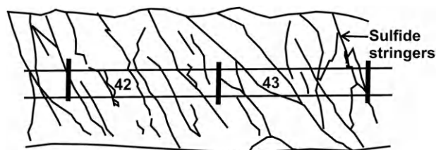
FIGURE 7.23 Schematic presentation of channel sampling of mineral exposure at surface and underground mine crosscut wall at 1 m interval.
