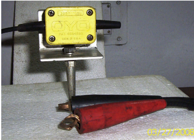
FIGURE 5.8 A three-component vertical 14-Hz “geophone” device for detection and recording of seismic reflection and refraction from subsurface interface.
