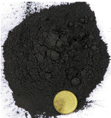
FIGURE 12.42 Lead concentrate with grade up to 65% Pb is achieved based on feed quality.
