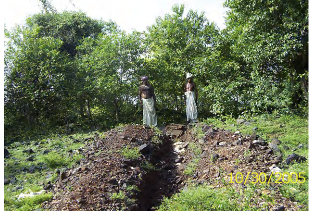
FIGURE 7.21 Trench sampling for platinum group of elements and chromite during Reconnaissance survey at Sitampundi layered igneous complex, Tamil Nadu, India.
