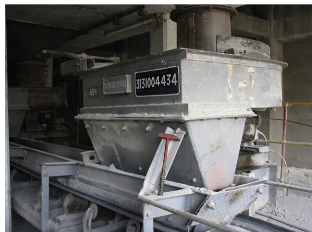
FIGURE 12.16 Close circuit transfer of oversize material from secondary crusher collected in ore bin (top) and auto-transfer to tertiary crusher by conveyer belt (bottom).
