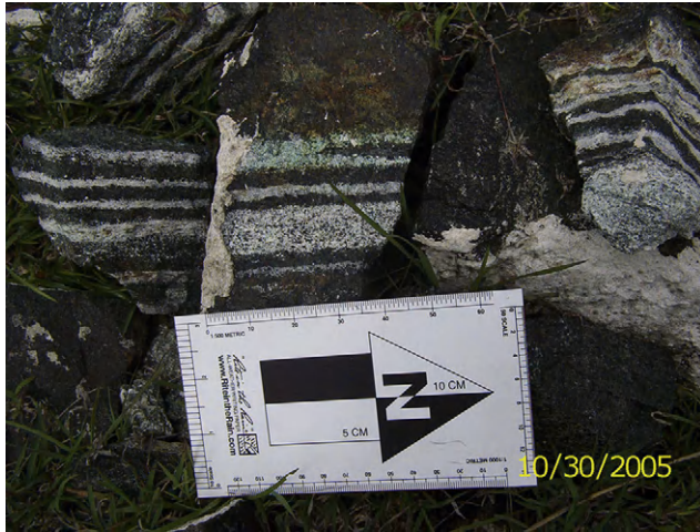
FIGURE 2.14 Layers of chromite (black) and Pt-Pd-bearing gabbro (white), Sittampundi Igneous Complex, Tamil Nadu, India.
