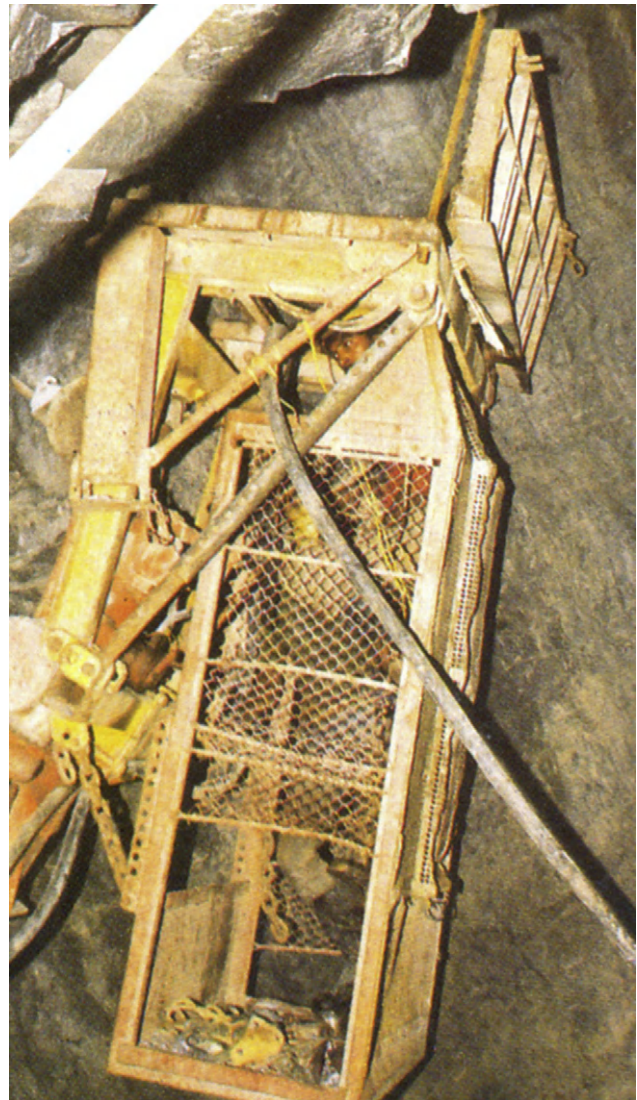
FIGURE 11.12 Alimak raise climbers are often in use for vertical or inclined excavation to join between levels and sublevels.
