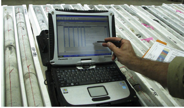
FIGURE 7.19 “Tough book”—a high-tech Internet interfaced data sharing drill core logger used at Lennard Shelf Exploration Camp, Australia.
