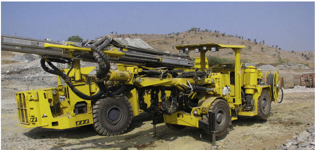
FIGURE 11.31 Single boom drill jumbo with basket diesel-powered articulated chassis and permanent four-wheel drive.
