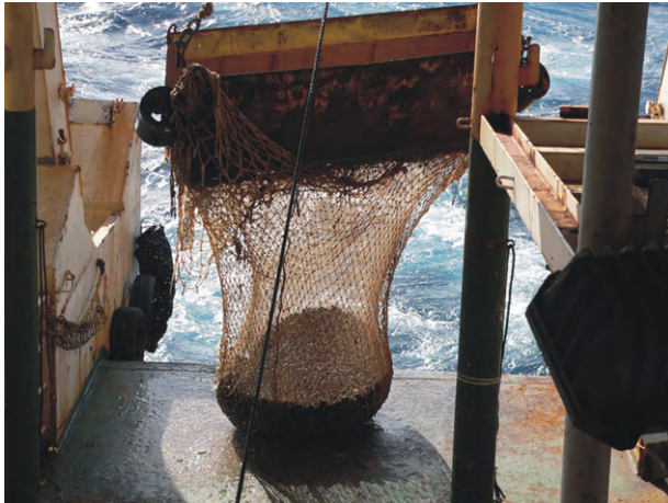
FIGURE 7.31 Bucket-in-pipe poly-metallic nodule sample lifting system collected from deep ocean floor (Credit: Arpita De).
