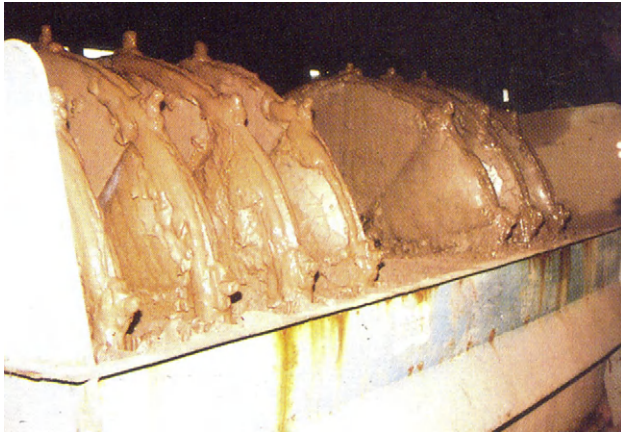
FIGURE 12.51 A view of disc filter in the second phase of dewatering of concentrate.
