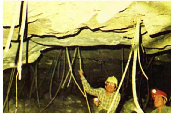
FIGURE 11.41 Cable bolting is suitable to bind large rock masses for extended period and adopted as appropriate support system in bad ground.
