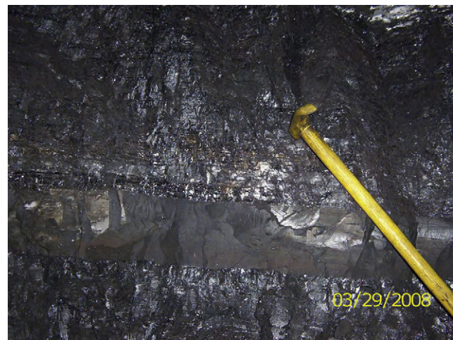
FIGURE 2.13 Alternate bands of coal (shining black) and shale (brownish gray), Belatan mine, Jharia coalfield, India.
