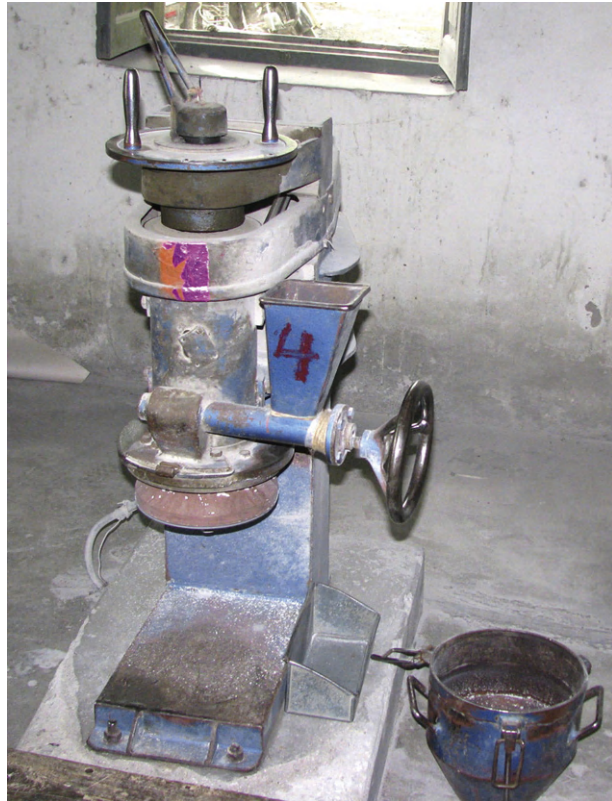
FIGURE 7.34 Sample size reductions by laboratory scale disc, ball or rod pulverizer.
