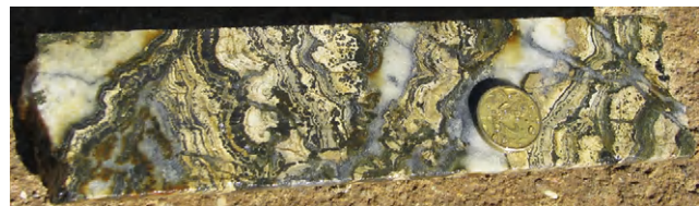
FIGURE 2.15 Sphalerite (yellow) and galena (black) mineralization in calcite (white) bands indicating different fluid phase events, Lennard Shelf MVT deposit, Western Australia.
