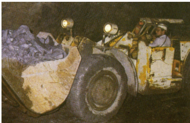
FIGURE 11.37 Diesel/compressed air-driven 1.5 m 3 LHD transporting the broken ore from working stopes to loading points.
