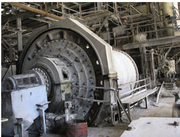
FIGURE 12.17 Standard grinding ball mill plays significant role to complete the liberation of ore and gangue minerals. It is in operation at Zawar Mine, India.
