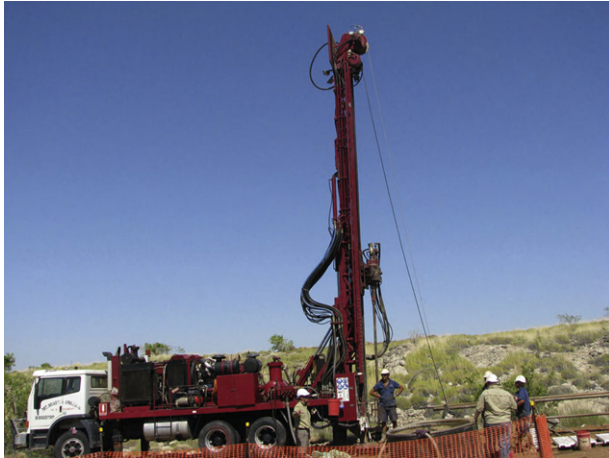
FIGURE 7.6 Truck-mounted diamond drill rig in operation for base metal exploration in Australia and capable of drilling 50-100 m a day.
