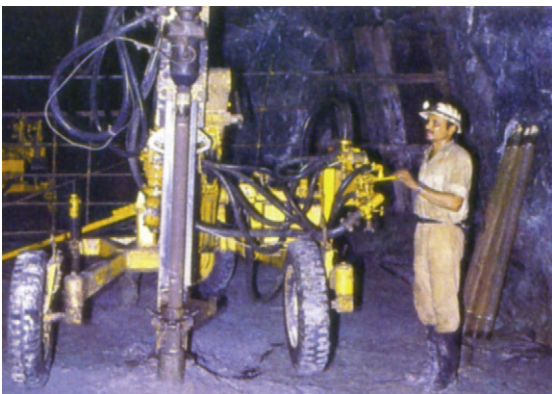
FIGURE 11.33 Tire-mounted DTH hammer drill rigs in operation for drilling 60 m vertical height of VRM stopes at Rajpura-Dariba mine during 1990s.
