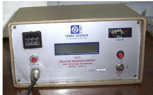
FIGURE 5.13 User-friendly proton magnetometer device compatible to high-end processing with precision.
