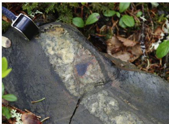
FIGURE 5.4.15 Uraninite grain 15 mm across within a dolomite–calc-silicate vein with thin biotite selvage enveloped by albite-rich alteration of metabasalt.
