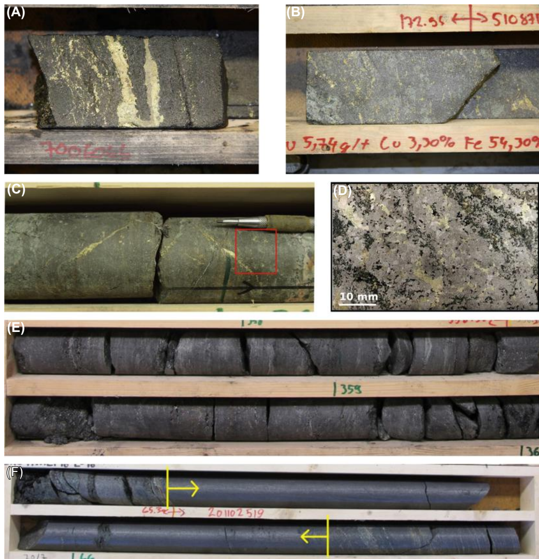
FIGURE 6.9 Different styles of oxide and sulfide occurrences in the Hannukainen deposit.
