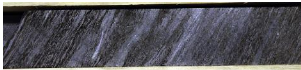
FIGURE 5.4.5 Metabasalt with strong foliation defined by biotite-amphibole-rich zones (dark) and lighter albitic alteration bands at South Rompas.
