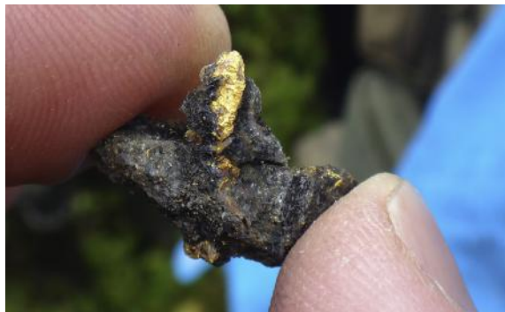
FIGURE 5.4.12 A small vein of gold within dolomite and fine dark amphibole.
