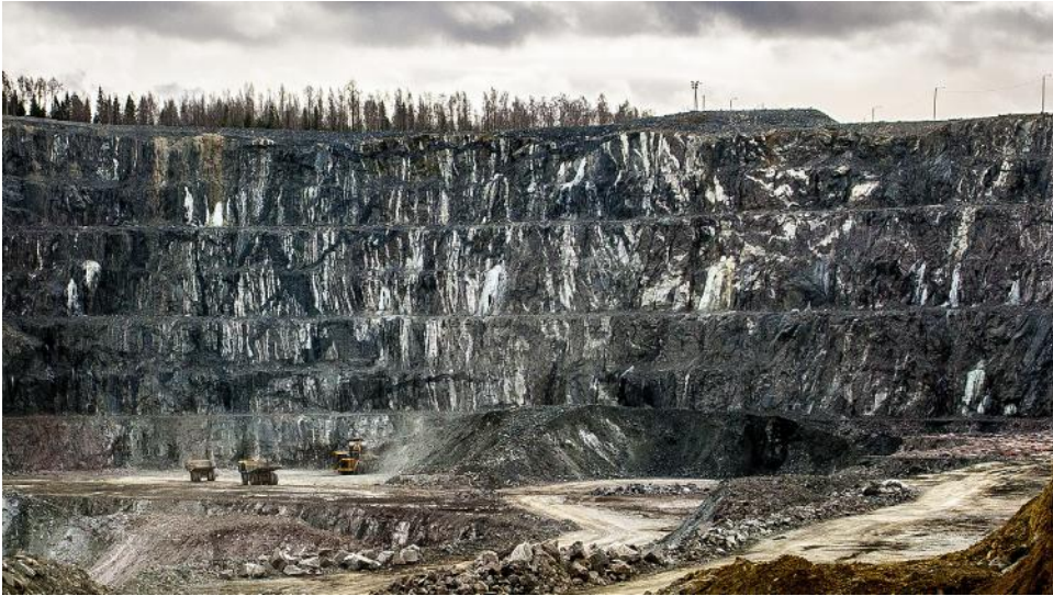
FIGURE 4.3.2 Photograph from the south wall of the main pit showing alternating glimmerite-rich and carbonatite-rich bands of the central portion of the main ore zone.
