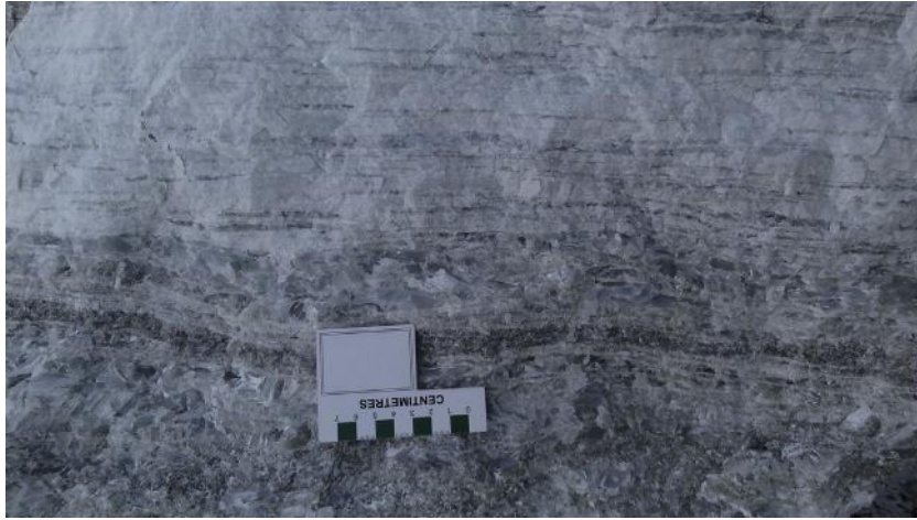
FIGURE 9.5.7 The main ore type of wollastonite consisting of sets of calc-silicate bands (wollastonite, diopside \pm quartz).
