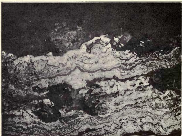
FIG. 160.—Photograph of branch vein on 1,000-foot level, El Oro Mining and Railway Company, showing pronounced banding by sulphides; vein three feet wide contains 9\frac{1}{2} ounces gold and 165 ounces silver per ton. Open cavity in middle.
