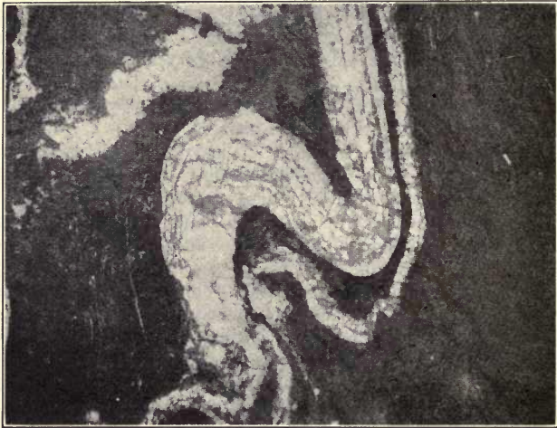
FIG. 202.—Folded quartz vein in slate, Mexican mine, Goldenville, Nova Scotia. After T. A. Rickard.
