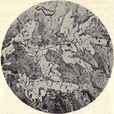
FIG. 53.—Feathery geocronite ( 5\text{PbS}\cdot\text{Sb}_2\text{S}_3 ) (white) replacing galena. Tintic, Utah. Magnified 24 diameters.
