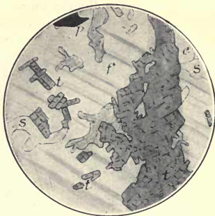
FIG. 59.—Replacement veinlet of tourmaline in fresh andesine grain. Keystone mine, Meadow Lake, Nevada County, Cal. t , Tourmaline; f , andesine; e , epidote; s , sericite. Magnified 50 diameters.
