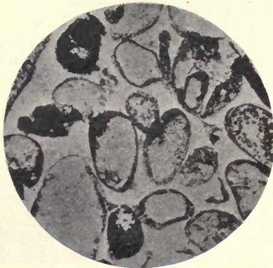
FIG. 123.—Ferruginous chert with greenalite granules, in part replaced by ferric oxide (black). Magnified 40 diameters. After C. K. Leith.
