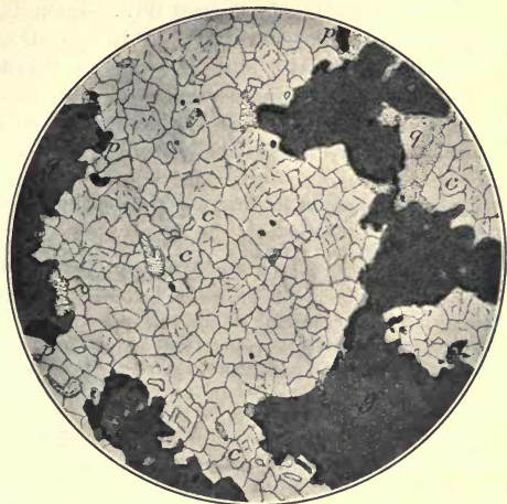
FIG. 63.—Galena, replacing crystalline dolomite. Elkhorn mine, Montana. g , Galena; p , pyrite; c , calcite grains of limestone; q , secondary quartz. Magnified 15 diameters.
