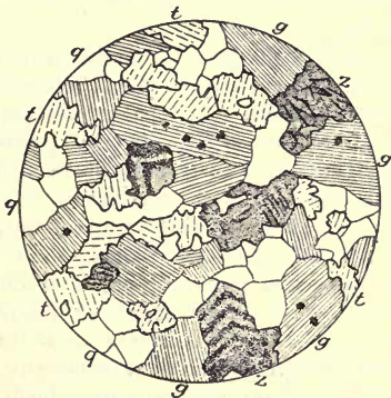
FIG. 226.—Thin section of greisen from Banka, derived from granite. g , Lithium mica; q , quartz; z , cassiterite; t , topaz; stippled spots in mica consist of zircon and rutile, surrounded by pleochroic rings. Magnified 45 diameters. After R. Beck.
