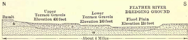
FIG. 78.—Diagrammatic section across Feather River below Oroville, California. a , Bed-rock; b , Ione formation; c , tuffs of Oroville.
