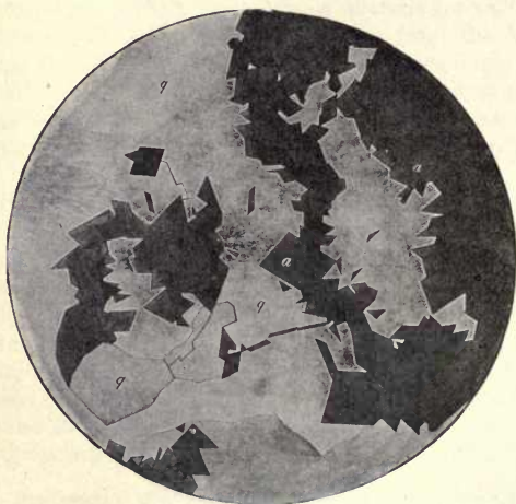
FIG. 146.—Intergrowth of quartz ( q ) and adularia ( a ), Fraction vein, Tonopah, Nevada. Magnified 38 diameters. After J. E. Spurr, U. S. Geol. Survey.
