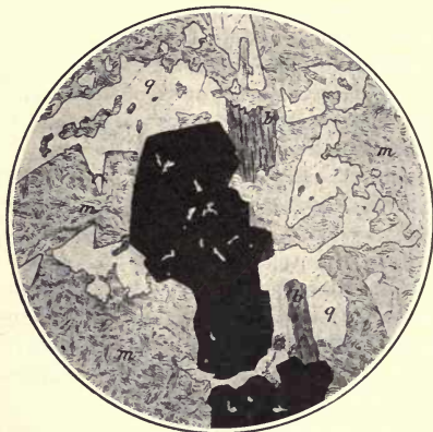
FIG. 184.—Altered granodiorite, Bellefontain mine, Nevada City, California. m , Fine aggregate of sericite with some calcite and quartz, replacing orthoclase and andesine; b , original biotite altered to sericite; q , original quartz; black, pyrite with included sericite. Magnified 15 diameters.
