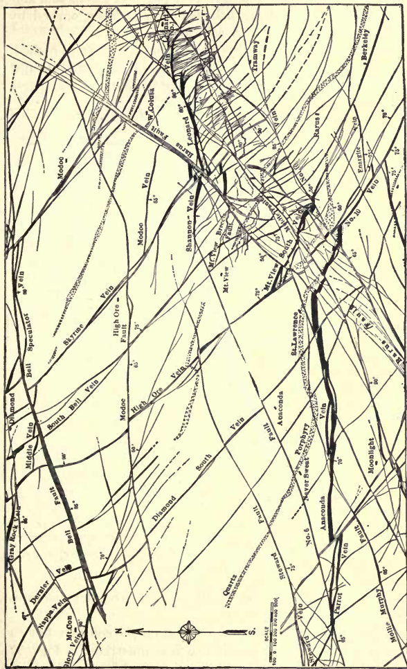
Fig. 46.—Horizontal section of part of Butte district, Montana, on level about 1,500 feet below surface. After Reno Sales.
