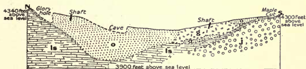
FIG. 255.—Generalized section of Brooklyn ore-body, Phoenix, B. C. o , ore-body; ls , limestone; g , gangue; j , jasperoid. Scale 400 feet = 1 inch.
