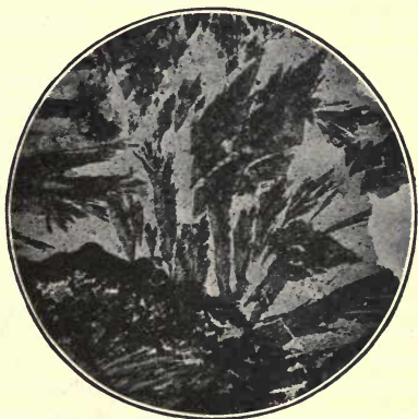
FIG. 273.—Photomicrograph of thin section showing azurite crystals replacing kaolin, Clifton, Arizona. Magnified 15 diameters.
