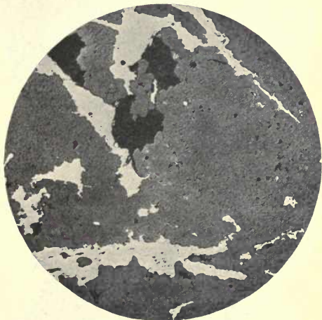
FIG. 52.—Replacement veinlets of galena (white) in cryptocrystalline quartz (dark gray) with vugs (black). Tintic, Utah. Magnified 11 diameters.
