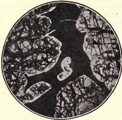
FIG. 264.—Thin section of olivine corroded by pyrrhotite and chalcopyrite East Union, Maine. Magnified 15 diameters. After E. S. Bastin.
