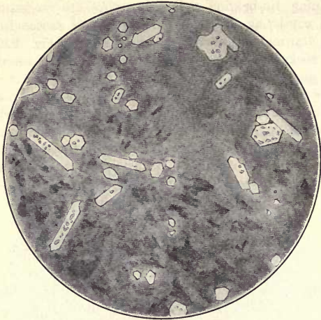
FIG. 57.—Incipient silicification of limestone. Aspen, Colo. White areas represent quartz crystals with small inclusions of limestone. Magnified 30 diameters.
