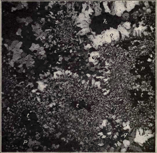
FIG. 183.—Photomicrograph of silicified dacite, Goldfield, Nevada, showing quartz of varying grain. p , Pyrite; t , famatinite; q , quartz; h , vug. Magnified 40 diameters. After F. L. Ransome, U. S. Geol. Survey .
