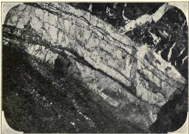
FIG. 191.—Argonaut vein in slate country rock, Amador County, California, at 650-foot level. Photograph by O. H. Packer. ¶
