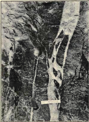
FIG. 219.—Photograph of vein of arsenides with inclusions of greywacke, Cobalt district. After W. L. Whitehead.
