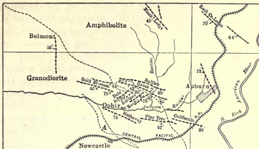
FIG. 188.—Map of principal vein systems near Ophir and Auburn, California. A, Small area of amphibolite. Scale 1 inch = 2.7 miles.
