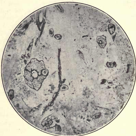
FIG. 6.—Section of chalcedonic spring deposits, from De Lamar, Idaho, showing vegetable remains. Magnified 35 diameters. Ordinary light.
