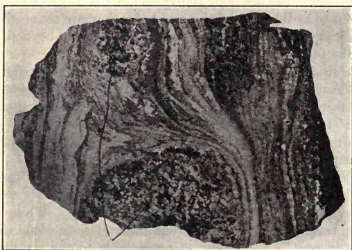
FIG. 225.—Nodules of barite and calcite (A) in banded sulphide ore from Rammelsberg, Germany. After Lindgren and Irving.
