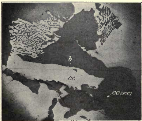
FIG. 272.—Intergrowth of bornite ( b ) and chalcocite ( cc ), Wall mine, Virgilina, North Carolina. cc (sec) , Secondary chalcocite. Magnified 50 diameters. After L. C. Graton and J. Murdoch.
