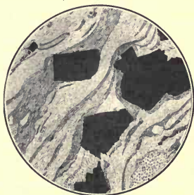
FIG. 144.—Crystals of galena developing in shaly dolomite. Black, galena; shaded and stippled, shaly dolomite; white, quartz. Magnified about 10 diameters. After E. R. Buckley.
