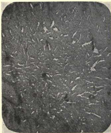
FIG. 283.—Photomicrograph of polished section showing residual galena (light) in anglesite (dark). Magnified 420 diameters.
