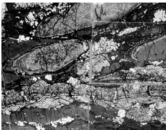
Figure 1: Collage of reflected light photographs of the polymictic Ni-Mo sulfide ore bed of Tianshan, near Zunyi, Guizhou. Widths of field approximately 2 mm. Note compositional variation of consisting of varying proportions of a layered C/MoS 2 phase (MoSC), iron and nickel sulfides, apatite, and organic matter. The light gray horizontal wavy band that extends through the middle of the photograph in the lower left-hand corner of the figure consists almost entirely of the new mixed layer (MoSC) that was first described by Kao et al. (2001). The presence of about 50 mole % carbon MoSC indicates that MoSC is not jordisite as is commonly supposed. Width of field = 2 mm.
