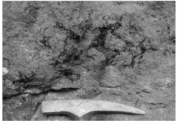
Figure 2: Bitumen (black) fills the fissures of basalt (grey). Field photo of the Sujiaqing copper deposit in NE Yunnan.
