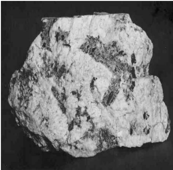
Figure 2: Coarse grained tourmaline in pegmatite sample from Vavdos. Irregular development of tourmaline (black) and associated quartz (grey) in a matrix of feldspar (white) and quartz. Bar scale = 2 cm.
