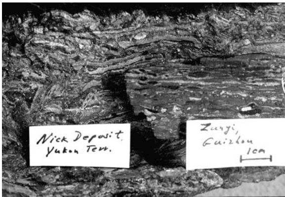
Figure 2: Cambrian-age Ni-Mo sulfide ore from Tianshan, near Zunyi, Guizhou sitting on a sample of Devonian-age mineralized Ni sulfide from the Nick deposit, Yukon.
