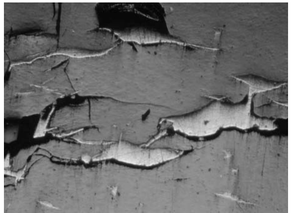
Figure 3: Native copper (white) fills the fissure of bitumen (grey). Polished section; plane polarized light; 0.6×0.4 mm. Sample taken from the Dadi copper deposit, NE Yunnan.
