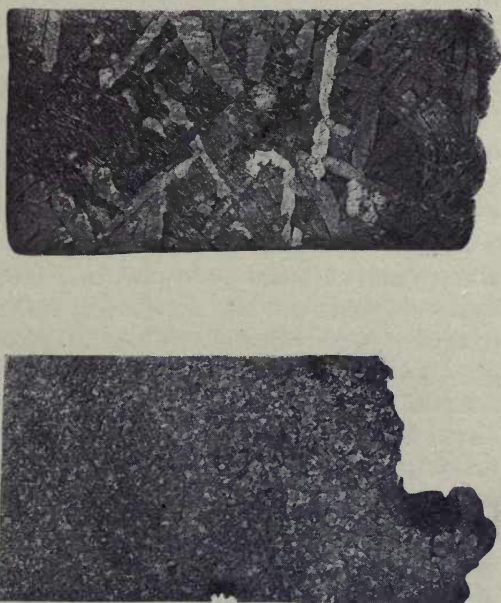
FIG. 43.—Effect of heating a section of the Toluca meteorite for 7 hours at 950^{\circ}\text{C} . Upper figure, before heating. Lower figure, after heating. The heating destroyed the lamellar structure and produced an appearance like that of some ataxites. After Berwerth.
