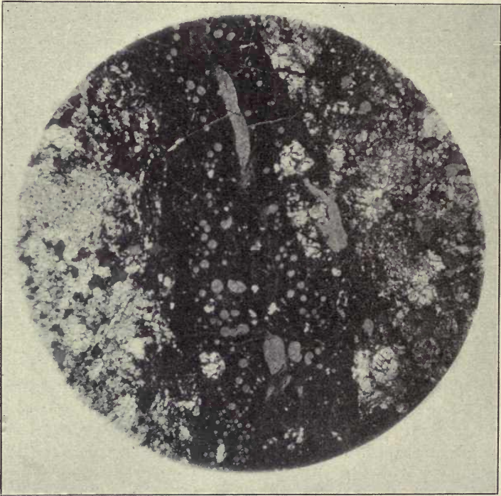
FIG. 34.— Cross section of a vein of one of the Mocs meteorites. The vein mass appears as a broad black band through the center. It is in part intermixed with the adjoining ground mass and in part has well-defined walls. The gray spots are lumps and spheres of nickel-iron illuminated by reflected light. The branching of some of these into clefts, one of which is still open, is of interest. \times 20 . After Tschermak.
