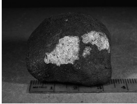
Figure 2.7 An individual specimen with fusion crust of the Chelyabinsk meteorite fall. (A black-and-white version of this figure will appear in some formats. For the colour version, please refer to the plate section.)
