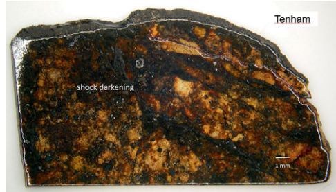
Figure 5.2 Phenomenon of "silicate darkening" a.k.a. "shock darkening" observed in the Tenham L6 ordinary chondrite. Reflected light.
