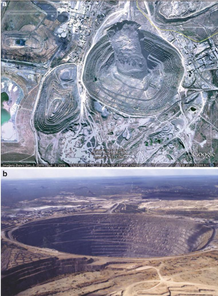
**Fig. 3.18** Two views of the Palabora open pit – a major Cu-rich multi-element deposit hosted in an alkali intrusion in South Africa
