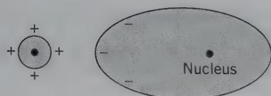
FIG. 3.10 Polarization effect of a small, highly charged cation on a large anion.
