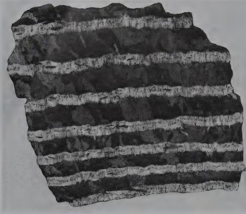
FIG. 19.54 Veins of chrysotile asbestos in serpentine. Thetford, Quebec, Canada.
