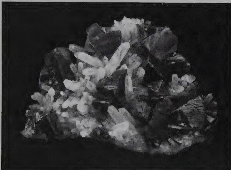
*Chalcopyrite,  $Cu_5FeS_4$ , as disphenoid crystals that are tetrahedral in aspect. The white crystals are quartz,  $SiO_2$ , with well-developed prisms and terminating rhombohedrons. (From St. Agnes, Cornwall, England (Harvard Mineralogical Museum.)*
