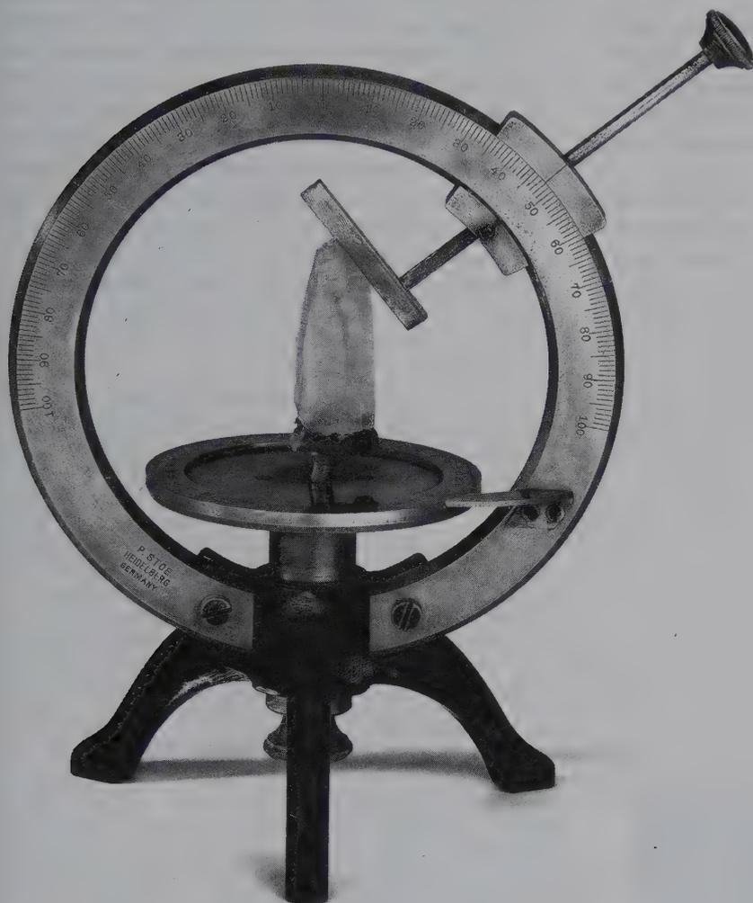
*Antique, two-circle contact goniometer based on the 1896 design of Victor Goldschmidt. The horizontal circle allows for the measurement of  $\phi$  angles, and the vertical circle of  $\rho$  angles. The crystal is quartz.*
