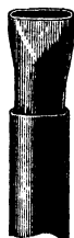
FIG. 2. The other end should then be cemented into the blowpipe by means of sealing-wax. This kind of mouthpiece, when inserted between the lips, displaces them but slightly from their customary position, and causes very little fatigue.
