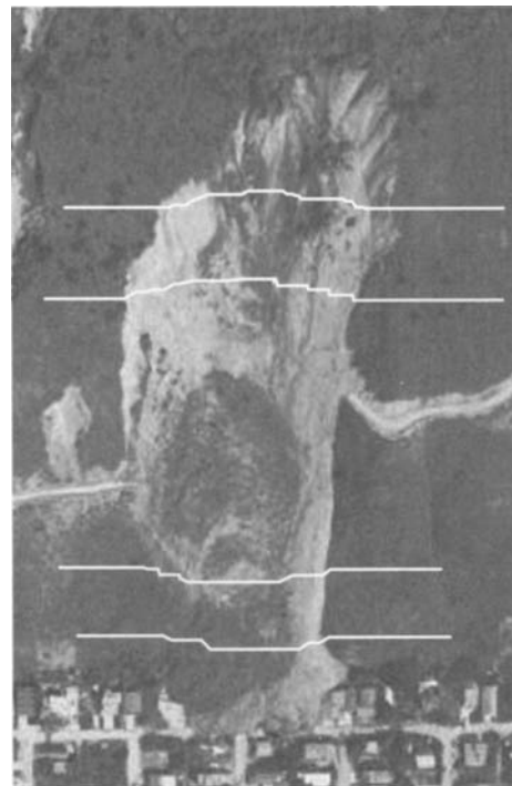
FIGURE 8.5 Contours that cross landslides, as shown on vertical photos, bend to follow concave part of slope in the upper scarp area of the slide. Contours in the lower part of a landslide will be convex and irregular over hummocky terrain. La Conchita, California, 1995; Same site as in Figure 8.4. Photograph courtesy of Pacific Aerial Surveys, http://www.geog.ucsb.edu/~jeff/projects/la_conchita/1995/95_slideshots.html
