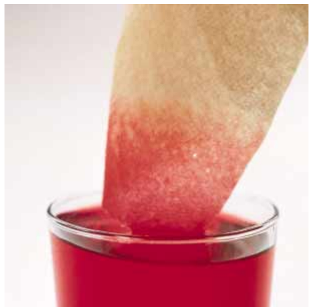
Figure 15-3 Capillary action pulls water upward from the water table just as it does in this paper towel dipped into dyed water.
