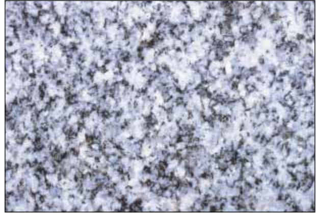
Figure 1–2 This granite rock is composed of different minerals, primarily quartz, feldspar, and hornblende. The mineral grains are a few millimeters in diameter.
