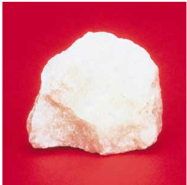
Figure 8–2 Metamorphism has destroyed the fossiliferous texture of the limestone in Figure 8–1 and replaced it with the large, interlocking calcite grains of marble.
