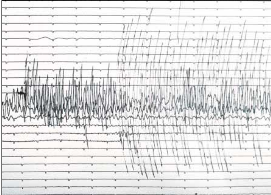
Figure 10-11 This seismogram records north-south ground movements during the October 1989 Loma Prieta earthquake. (Russell D. Curtis/USGS)
