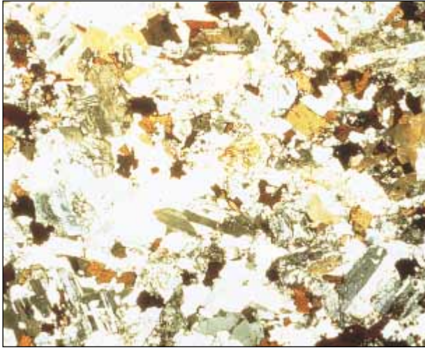
Figure 3-7 A photomicrograph of a thin slice of granite. When crystals grow simultaneously, they commonly interlock and show no characteristic habit. To make this photo, a thin slice of granite was cut with a diamond saw, glued to a microscope slide, and ground to a thickness of 0.02 millimeters. Most minerals are transparent when such thin slices are viewed through a microscope.
