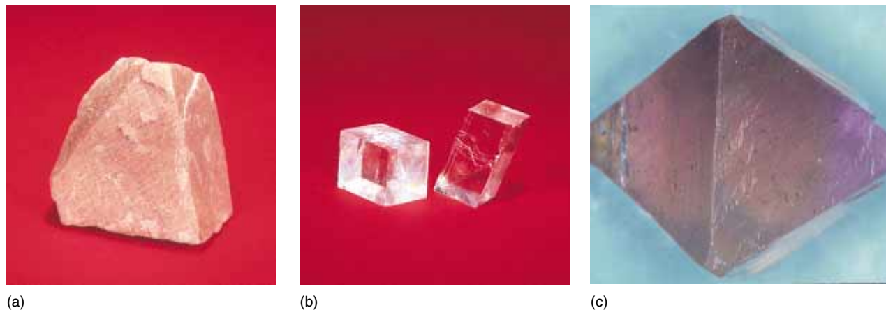
Figure 3-9 Some minerals have more than one cleavage plane. (a) Feldspar has two cleavages intersecting at right angles. (b) Calcite has three cleavage planes. (c) Fluorite has four cleavage planes. (Arthur R. Hill, Visuals Unlimited)
