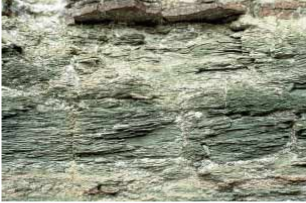
Figure 8-3 Shale is a very fine-grained sedimentary rock, containing clay, quartz, and feldspar.
