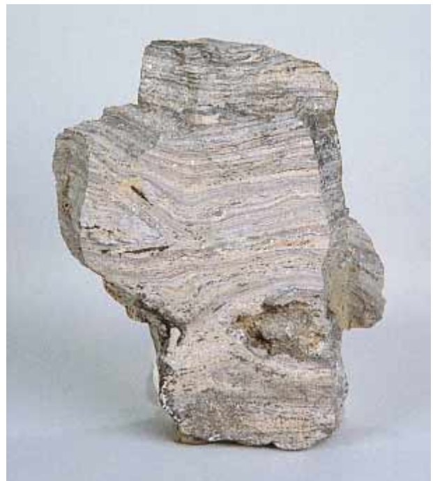
Figure 5–23 This welded tuff formed when an ash flow became hot enough to melt and flow as a plastic mass. The streaky texture formed when rock fragments similar to those in Figure 5–22 melted and smeared out as the rock flowed. (Geoffrey Sutton)
