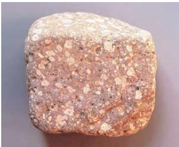
Figure 4-13 Porphyry is an igneous rock containing large crystals embedded in a fine-grained matrix. This rock is rhyolite porphyry with large pink feldspar phenocrysts.
