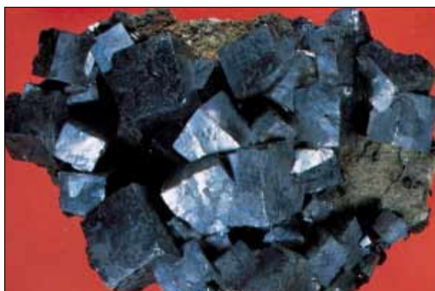
Figure 3–14 Galena is the most important ore of lead and commonly contains silver. (Ward’s Natural Science Establishment, Inc.)
