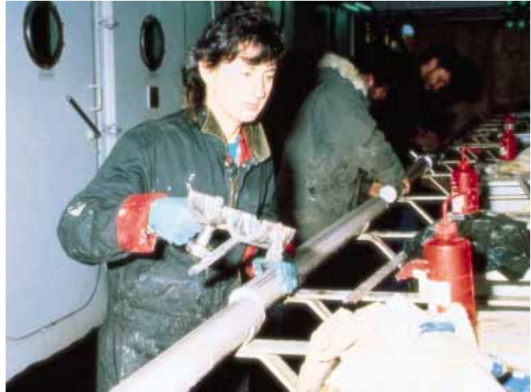
Figure 11-1 An oceanographer extracts sediment from a core retrieved from the sea floor. (Ocean Drilling Program, Texas A&M University)
