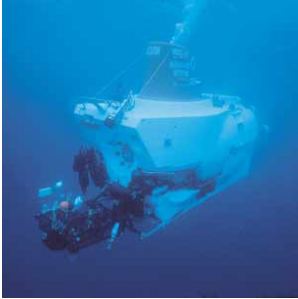
Figure 11-2 Alvin is a research submarine capable of diving to the sea floor. Scientists on board control robot arms to collect sea-floor rocks and sediment. (Rod Catanach, Woods Hole Oceanographic Institution)
