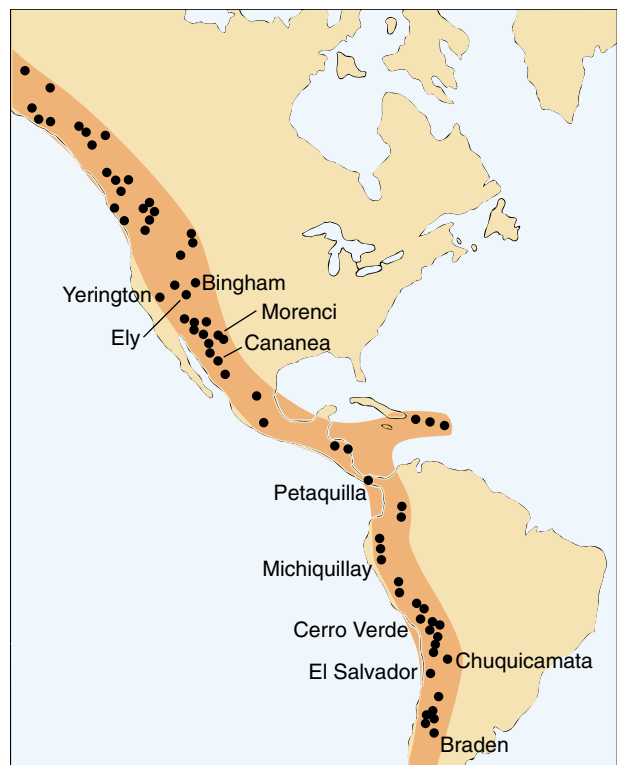
Figure 19-5 Porphyry copper deposits in the Western Hemisphere lie along modern or ancient tectonic plate boundaries.
