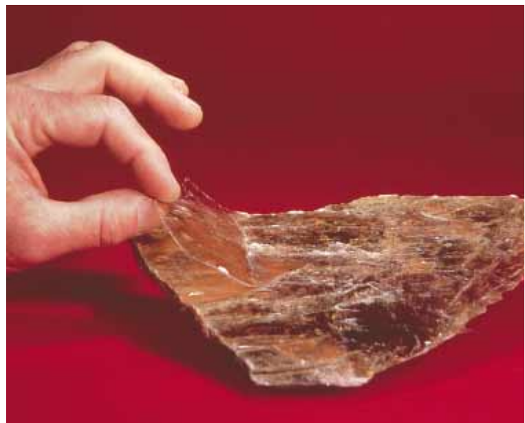
Figure 3-8 Cleavage in mica. This large crystal is the variety of mica called muscovite. (Geoffrey Sutton)
