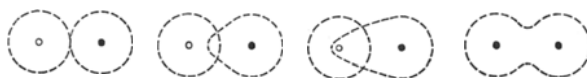
Fig. 157. Transition from ionic- to covalent bonding through polarization. (After K. FAJANS from Hedvall)
