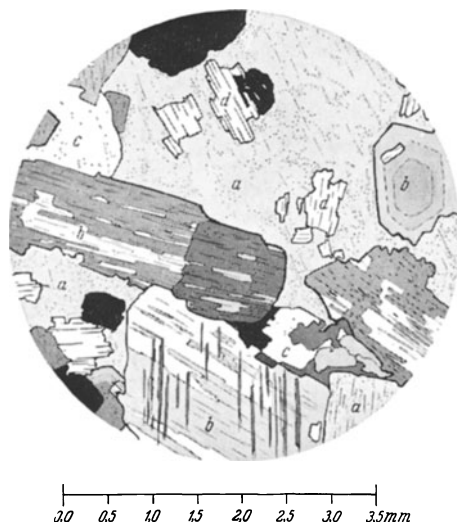
Fig. 313. Equigranular structure. Granite (La Ginnea, Genoa), between crossed nicols. a orthoclase, large somewhat cloudy crystals showing twinning; b plagioclase, large crystals with narrow twin lamellae and one zoned crystal; c quartz, clear, "pincher" shaped between feldspars; d mica, small crystals showing cleavage; one crystal intergrowth in zoned plagioclase
