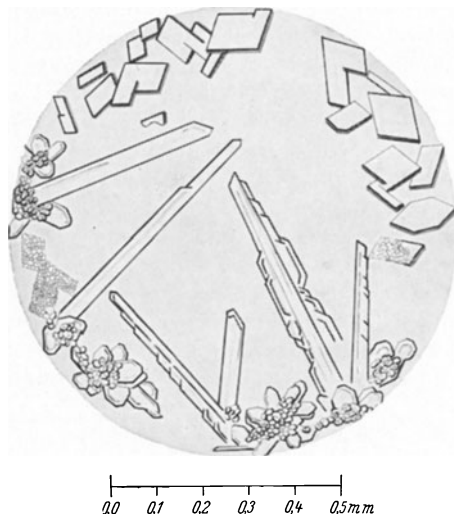
Fig. 290. \text{KNO}_3 crystallization by evaporation under the microscope. The first-formed rhombohedral crystals are transformed upon contact with the later forming orthorhombic needles (middle right). In their vicinity the rhombohedra are dissolved (left above)
