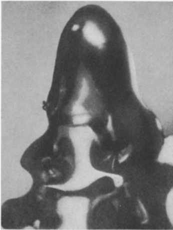
Fig. 279. Point of a copper dendrite ( \times 350 ). (After GRAF)
