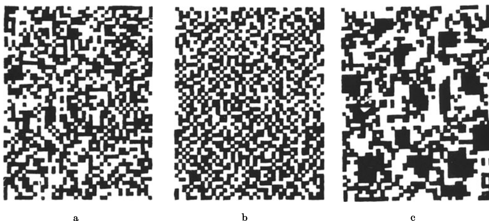
Fig. 180 a—c. Distribution of black and white squares, (a) statistical (random), (b) Deviation from random toward chess board pattern, (c) deviation toward segregation of larger black and white domains. (From LAVES)
