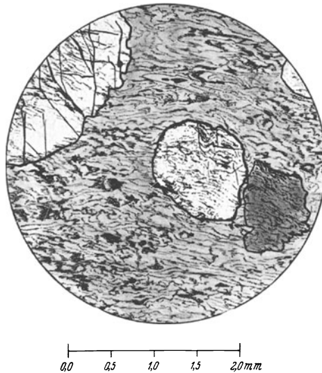
Fig. 374. Porphyroblasts in garnet-sericite schist. Pebble from the Mareiter Bach at Bozen. Two large garnets (bright) and mica crystal (dark) in a groundmass of quartz, sericite and carbonaceous matter. Schistosity of groundmass preserved within large crystals
