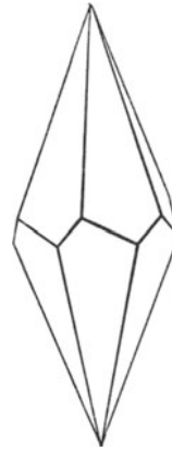
Fig. 85. Left-handed hexagonal trapezohedron
