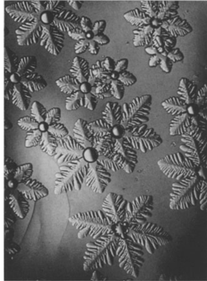
Fig. 280. Tyndall figures in ice. Picture taken parallel to hexagonal axis of the crystal. (After BASS and MAGUN)
