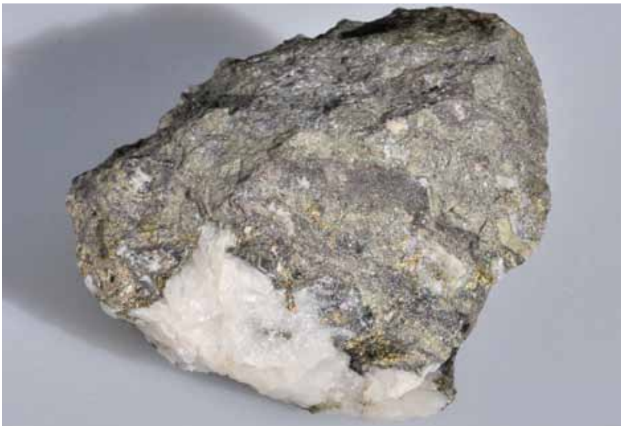
Figure 5.2 A more complex paragenesis From the same area of North Wales as Fig. 5.1, this hand-specimen of quartz and intergrown sulphides belongs to a completely different generation of veining. Chalcopyrite, pyrite, sphalerite and galena are all visible to the naked eye but their relationships to one another are not discernible because they are so finely intergrown. Together, these specimens demonstrate two important things: firstly that mineralized districts commonly contain more than one generation of mineralization, and secondly that sectioning and examination of mineral assemblages using a petrological microscope is essential if the mineralogist is to get the full picture.
