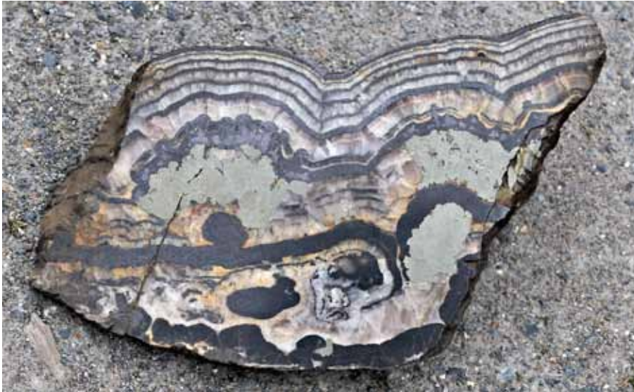
Figure 5.1 A straightforward paragenesis Large (30 cm wide) specimen of coarse-grained vein mineralization from North Wales. Sphalerite and calcite occur in repeated bands from the vein wall (bottom) to its central cavity (top); some of the bands also contain marcasite and galena. The order in which the minerals were deposited can plainly be seen.
