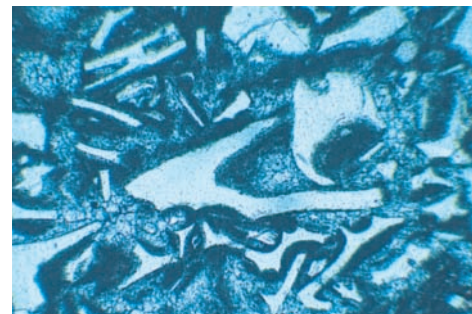
f Microscopic view of a fragmental texture. The colorless, angular objects are pieces of volcanic glass measuring up to 2 mm.
