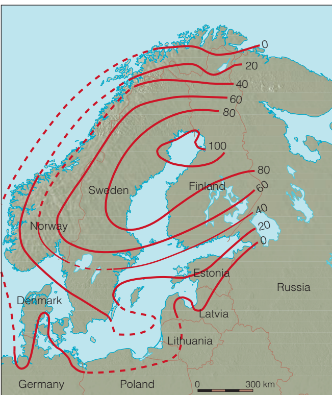
c Isostatic rebound in Scandinavia. The lines show rates of uplift in centimeters per century.
