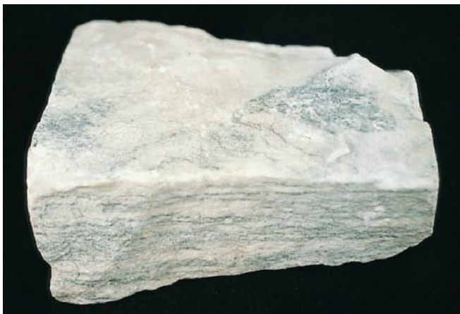
c Rock gypsum. When deeply buried, gypsum ( \text{CaSO}_4 \cdot 2\text{H}_2\text{O} ) loses its water and is converted to anhydrite ( \text{CaSO}_4 ).
