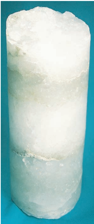
a This cylindrical core of rock salt was taken from an oil well in Michigan.
