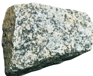
b Slower cooling in plutons yields a phaneritic or coarse grained texture.
