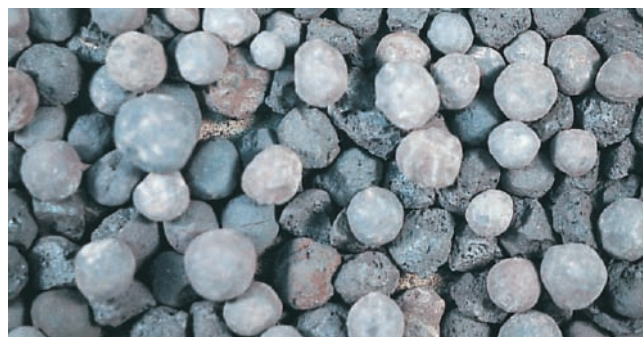
b The Iron ore is refined and shaped into pellets containing about 65% iron. The pellets are about 1 cm across.
