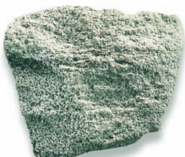
c Pumice is glassy and vesicular; its density is so low that it floats.
