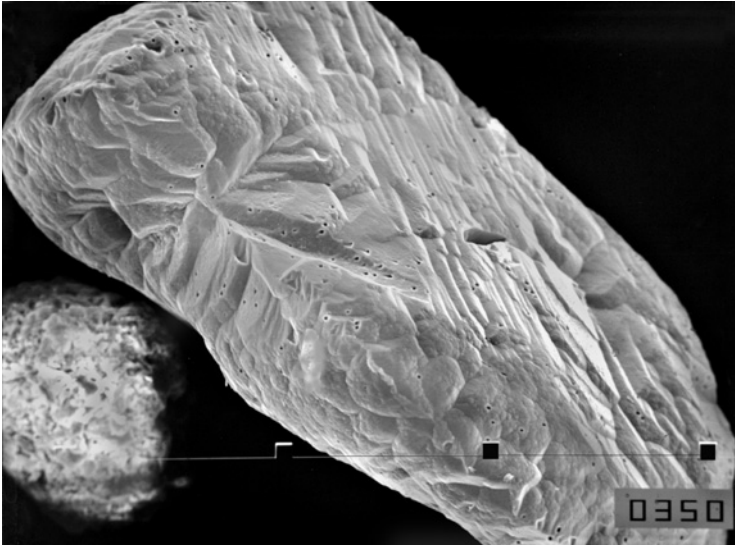
Fig. 3. Etch pits superimposed on imbricate wedge marks (inherited from diagenetically altered Palaeozoic sandstones in the source area of the glacial deposits) on garnet from agricultural soil at the Michigan State University Kellogg Biological Station. Scale marks are 100 \mu\text{m} apart.
