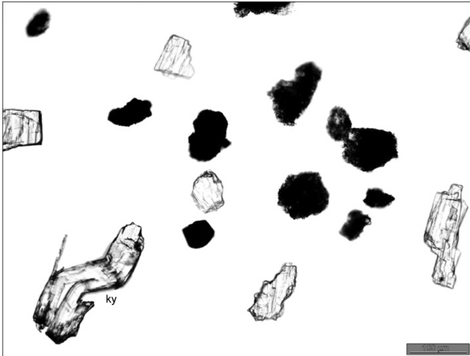
Fig. 9. Grain mount of a high-temperature fired specimen containing neo-formed calcite crystals and a bent, etched kyanite (ky) grain.
