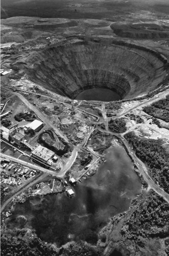
Kimberlite pipe outside of Mirney, Russia. Diamonds are formed in the Earth's mantle and brought up to the surface in the volcanic rock called kimberlite. Kimberlites form pipe-shaped intrusions, and diamond miners dig vertically downward, following the pipe into the Earth. (Sergei Karpukhin, Reuters/Landov)
