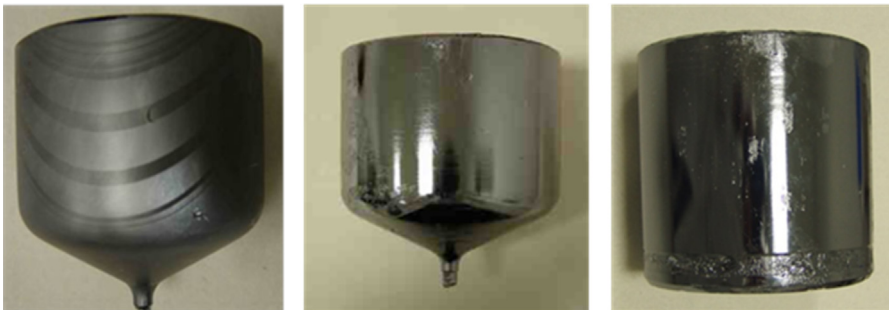
FIGURE 9.8 Heavily twinned 4-inch liquid encapsulation vertical gradient freezing (LEVGF) IP crystal and twin-free crystals grown in a standard and a flat bottom crucible, respectively.
