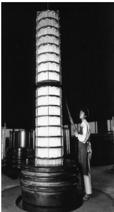
FIGURE 14.2 Production of quartz crystals in the world's largest autoclave. Photograph courtesy S. Taki, Japan [3].
