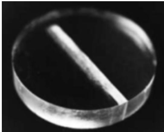
FIGURE 26.18 Cracking of a GSO test specimen observed in a thermal stress test. From Ref. [49] with permission of Tech Science Press.
