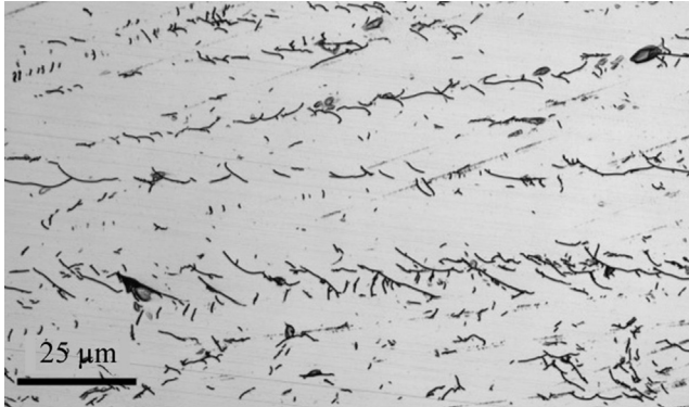
FIGURE 18.12 Optical microscope image of an etched, beveled wafer surface after fixed abrasive sawing. The microcracks are aligned along the wire motion direction.
