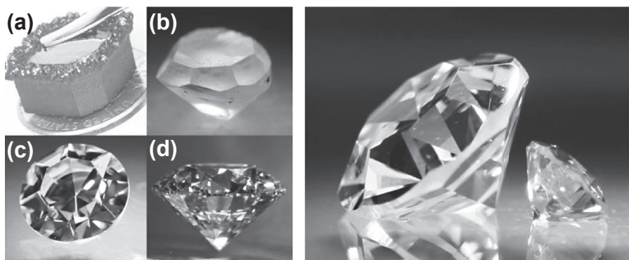
FIGURE 17.17 The picture on the right shows a 2.4-carat single-crystal CVD diamond compared with 0.25-carat CVD diamond. On the left, example of the evolution of CVD diamond single crystal starting with crystal 13.5-carat block (a) to the 2.3-carat cut gem anvil (d). Reprinted with permission from Ref. [187]. Copyright 2012, Wiley-VCH Verlag GmbH & Co. KGaA.
