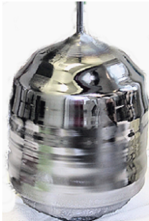
FIGURE 3.4 The 160-mm diameter GaAs grown by the modified vapour pressure–controlled (VCz) inside the diving bell using As vapor pressure control. After Neubert et al. [23] with permission of Elsevier.
