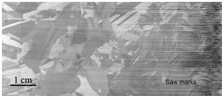
FIGURE 18.8 Part of an as-sawn silicon wafer surface showing saw marks.
