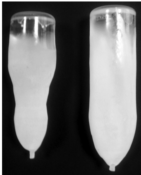
FIGURE 19.20 Two 40-mm diameter sapphire crystals grown by the Verneuil process, with (right) and without (left) efficient process control. The white aspect is due to a nitride layer that appears on the boule surface, due to air reaction at a temperature lower than the melting point.
