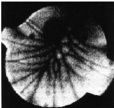
FIGURE 22.15 Spoke patterns observed on the \text{LiNbO}_3 melt surface without the crystal. (From Ref. [52].)
