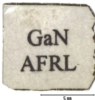
FIGURE 15.21 A transparent GaN crystal grown under ammono-basic conditions. (Reprinted from Ref. [90] with permission.)
