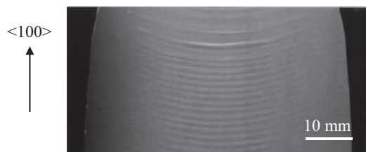
FIGURE 2.14 X-ray topography of a longitudinal section of a silicon Cz crystal grown under the influence of a cusp magnetic field. The nonuniform incorporation of dopants causes the occurrence of growth striations displaying the shape of the solid–liquid interface. Reprinted from Ref. [85] with permission from Elsevier.
