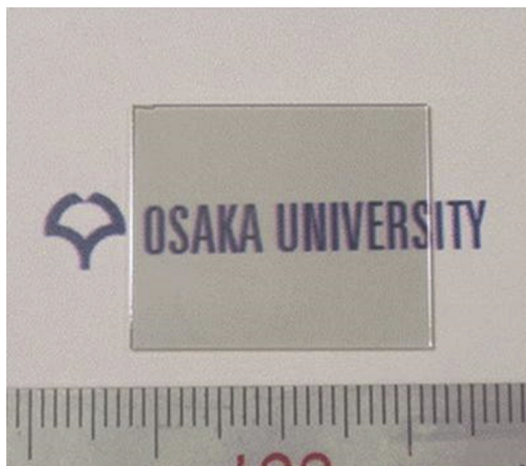
FIGURE 13.20 Photograph of the GaN crystal grown by the Na flux LPE method on HVPE-GaN seed crystals. Both sides of the crystal were polished to the thickness of 750\ \mu\text{m} to remove the seed crystals.
