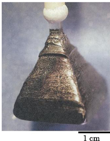
FIGURE 30.23 As grown 1-inch-class size NdBCO single crystal produced by continuous pulling for 67 h from \text{Ba}_3\text{Cu}_5\text{O}_8 solvent melt in the \text{Nd}_2\text{O}_3 crucible in the air atmosphere. Its size is 24 \times 24 \text{ mm}^2 in the ab -plane and 21 mm in the c -axis direction [128]. © 1997 The Japan Society of Applied Physics.
