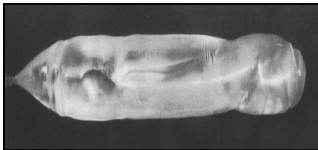
FIGURE 4.23 CWO crystal grown by CZ method.
