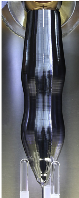
FIGURE 7.12 Image of the grown Avogadro crystal using regulation. The image was taken by Turschner at the Leibniz Institute for Crystal Growth (IKZ).
