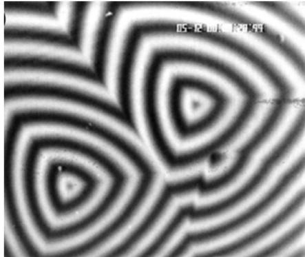
FIGURE 24.12 Michelson two-beam interferogram from spiral hillocks of  $\text{Ba}(\text{NO}_3)_2$  growing in solution.
