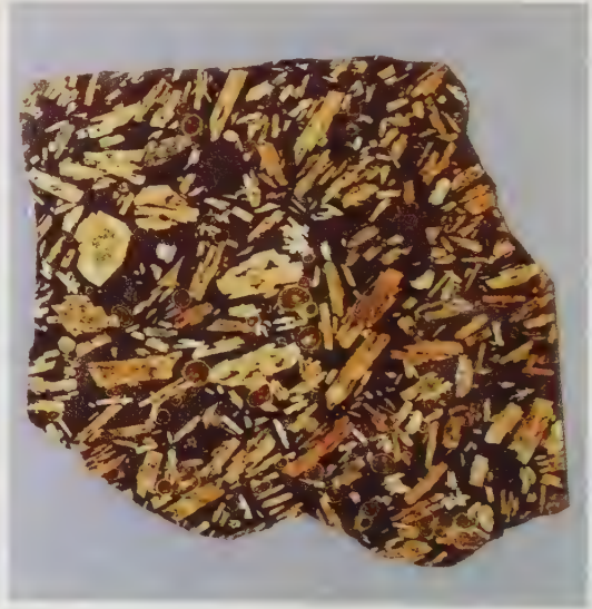
Amygdaloidal Porphyritic Lava. Copper River near Terrace, B.C. Contains pink feldspar crystals and green epidote filled vesicles.
