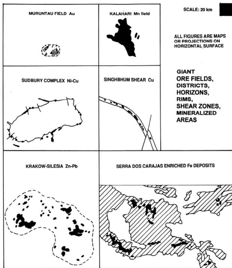
Figure 2.2c. Configuration, "footprint" and internal complexity of "giants": ore fields, districts, horizons, shears
