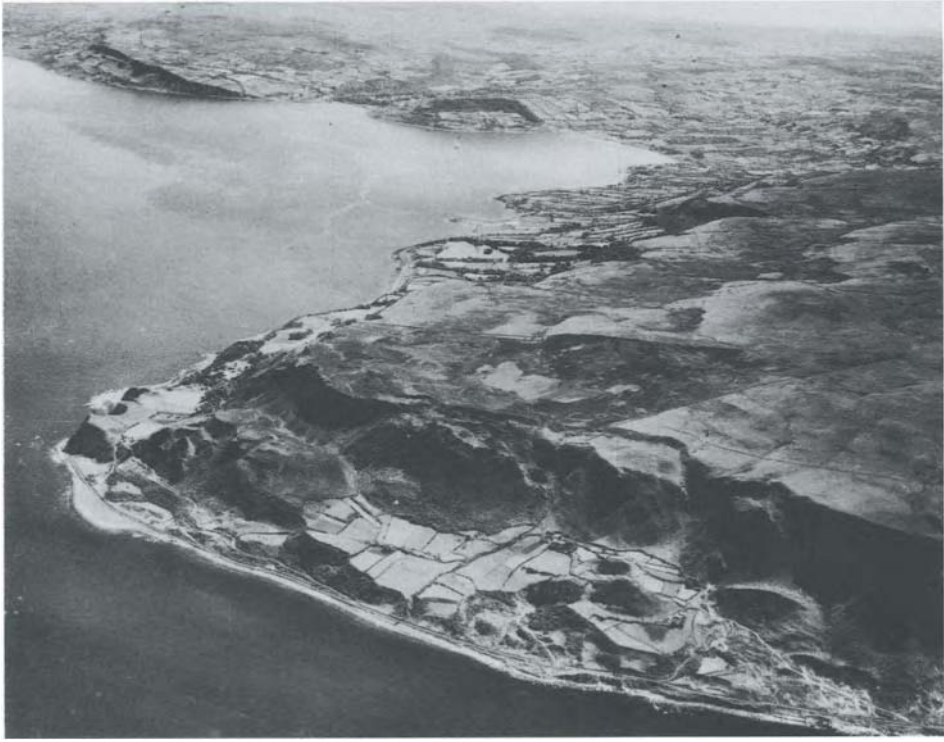
Fig.11.5. Aerial view of Garron Point, Co.Antrim, showing multiple rotational landslips, with vertical displacements of up to 125m, below the plateau surface at about 300m O.D. Some of the blocks have prominent steep seaward faces and back-tilted upper surfaces, while others have been degraded by weathering and their outlines obscured by aprons of block scree (Photo: Aerofilms Ltd )
