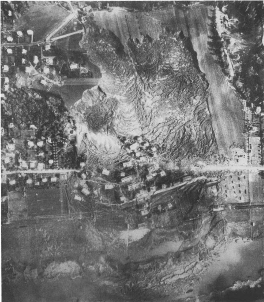
Fig.19.4. The Surte slide. Note the bulge into the river (lower) and the disturbed road and railway. The clay crust has been broken into separate narrow blocks, indicating the movement in the soft clay below (photo from Caldenius and Lundström, 1956).
