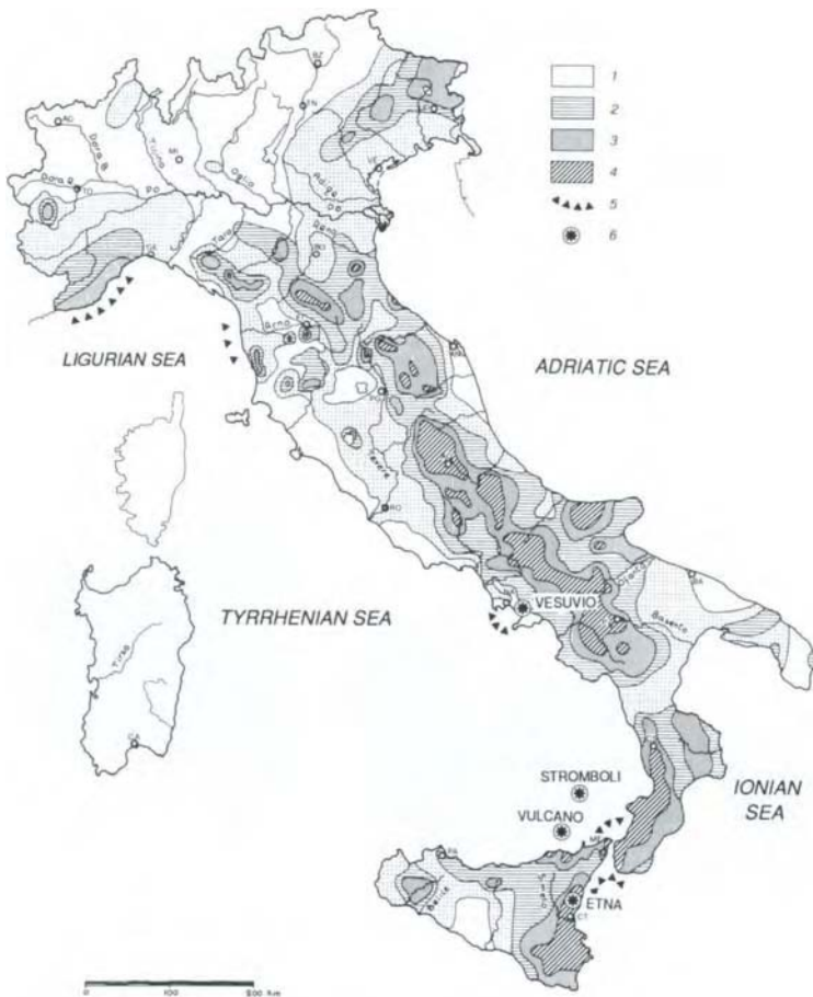
Fig.12.3. Seismic and volcanic activity in Italy, showing areas of maximum earthquake intensity on the Mercalli scale: 1: \leq VII; 2: VIII; 3: IX; 4: \geq X; 5: coastlines most likely to be affected by tsunamis; 6: active volcanoes
