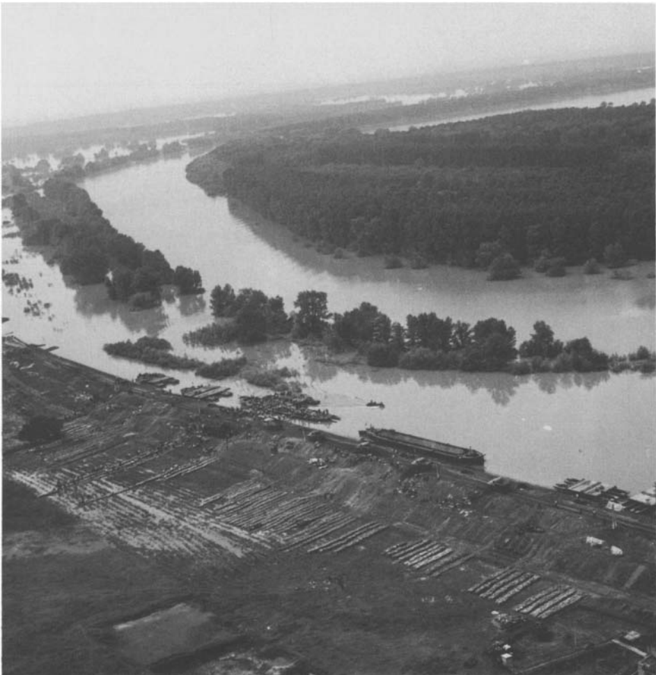
Fig.10.2. Bankfull discharge on the Tisza river in May 1970, caused by the damming effect of tributaries (photo: Water Management Documentation Aerial Photography Service)
