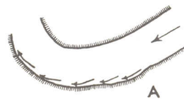
Diagram showing the place of greatest erosion on the bend of a river.
