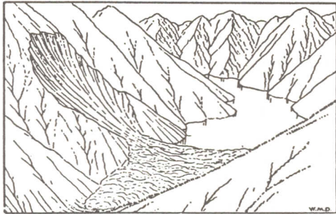
Ideal sketch showing how a landslide may dam up a mountain valley to form a lake. Silt, sand, and gravels deposited in and on the edge of this lake will cover the stream gravels in its bottom. (After Davis, State Mineralogist's Report XXIX .)
