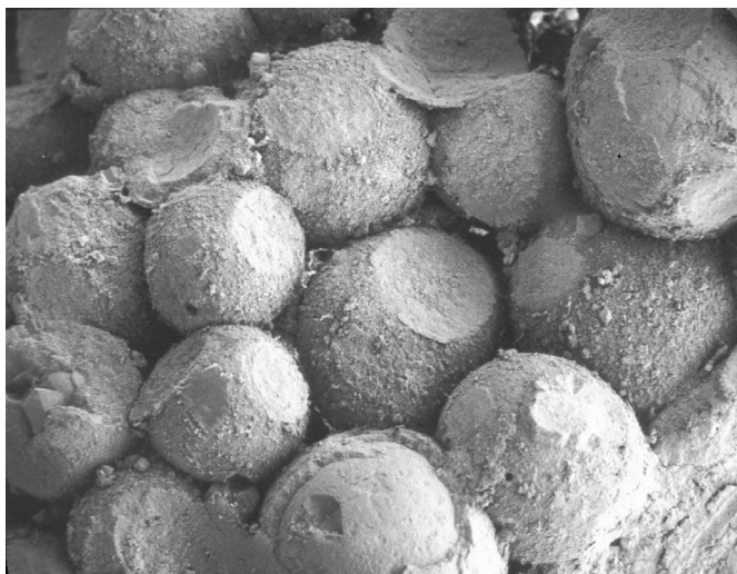
Figure 8.4 SEM micrograph of the oolitic reservoir rock at North Haynesville Field showing the relatively undeformed and uncemented oolites from the principal oolite grainstone reservoir facies that occurs along the paleostructural highs in the field. This pore system is a good example of depositional, intergranular porosity following the genetic classification system illustrated in Chapter 2. The average diameter of these ooids is about 1 mm. (Photo by H. Ben Hull in Ahr and Hull (1983).)
