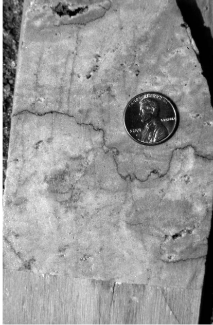
Figure 6.1 The stylolite just below the 1-cent coin is typical of these features that are formed by the combination of pressure and dissolution. Most of them are filled with insoluble material, commonly including or limited to bituminous residue and most stylolites are baffles or barriers to flow. A few may remain open, or become opened during later dissolution, in which case they may provide access for fluid migration (see the sketch in Figure 6.6). This stylolite, like most, resembles a trace on a seismograph or an electrocardiogram. Note the small natural fractures and dissolution vugs also in this core segment from a Mississippian-aged dolomitic reservoir in Texas.
