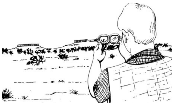
Fig. E.3 Measuring the dip of beds on a distant mesa by sighting along strike
