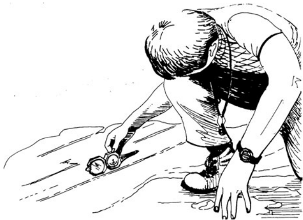
Fig. E.6 Measuring the plunge of a lineation with a Brunton™ compass
