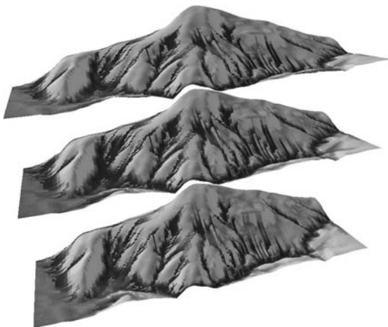
Figure 13.12 Groundwater pattern for hillslope “si7” and the three climate scenarios. Top: climate scenario 1, middle: climate scenario 2, bottom: climate scenario 3 (compare Figure 13.9). Dark: groundwater close to surface.
