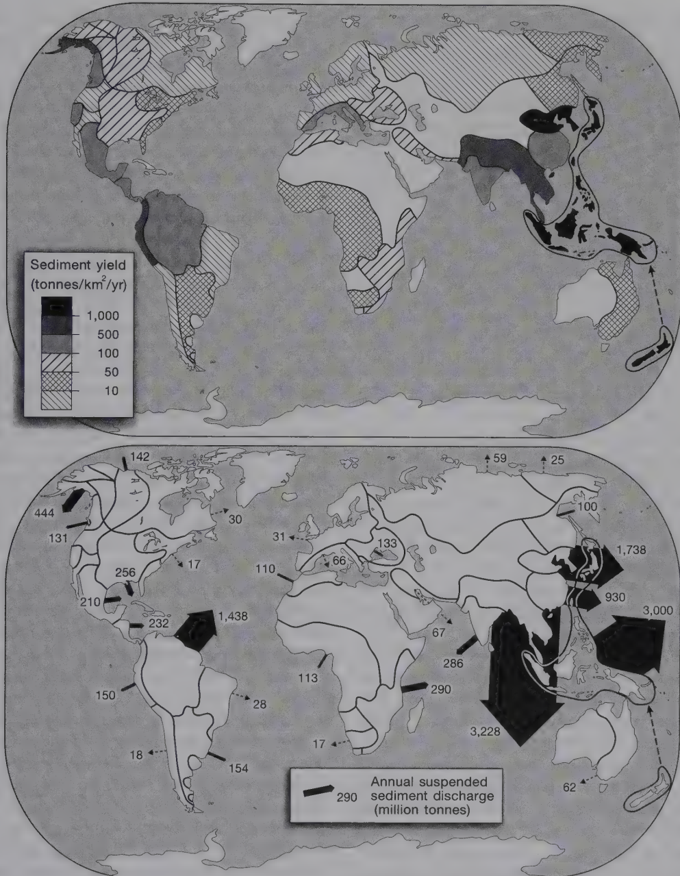
Figure 2.7 (a) Sediment yield of the world's chief drainage basins. Blank spaces indicate essentially no discharge to the ocean. (b) Annual discharge of suspended sediment from large drainage basins of the world. The width of the arrows corresponds to relative discharge. Numbers refer to average annual input in millions of tonnes. The direction of the arrows does not indicate the direction of sediment movement.
