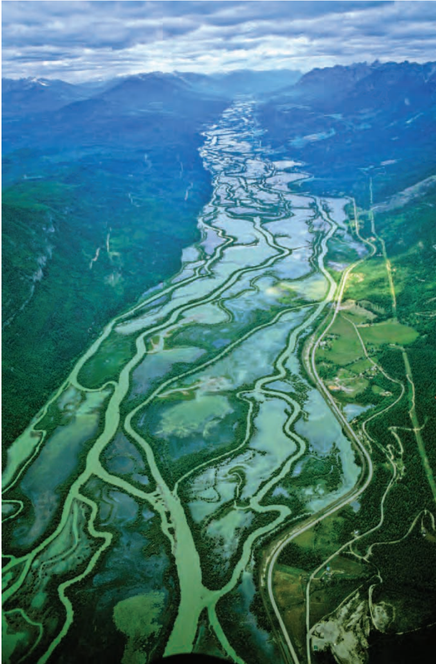
Colour Plate 9 Columbia River, near Harrowgate, British Columbia, Canada, during the annual summer floods. Levees can be seen as raised ridges bordering the channels and they have been breached in places, resulting in the deposition of splays. Photograph by Airphoto, Jim Wark.
