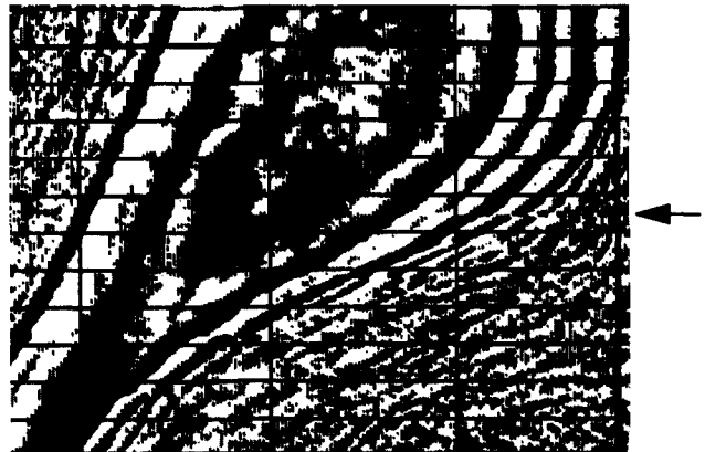
Fig. 5-10. Timeslice through stacked 3-D data set acquired with 4/4 geometry. Note discontinuities every 16th East-West midpoint line (a horizontal gridline is drawn every tenth midpoint line).
