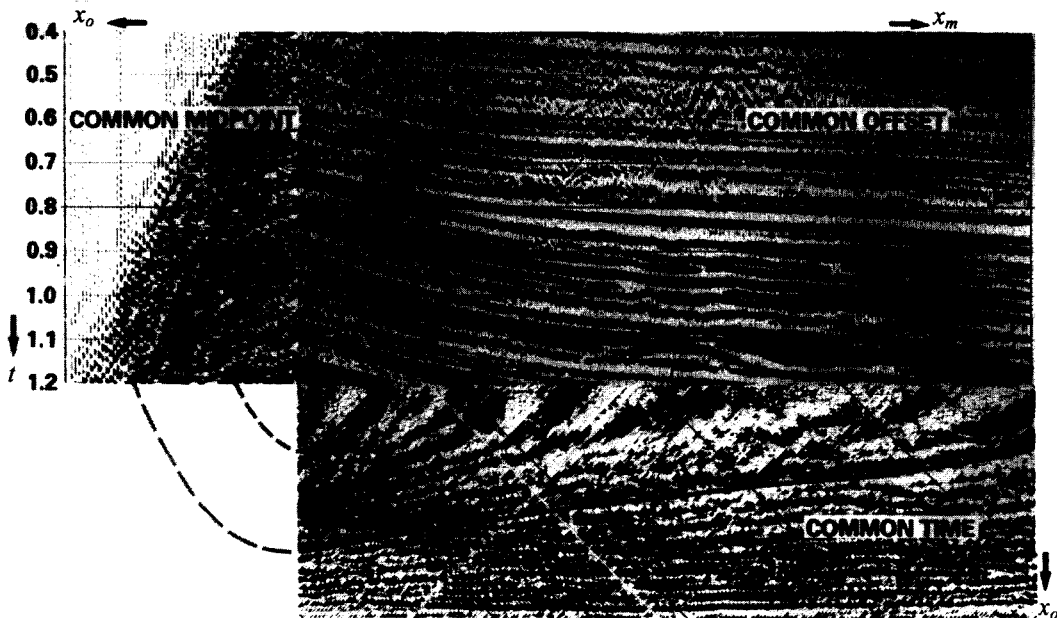
Fig. 1-4. Three cross-sections through prestack data set. Note that each event is a surface in 3-D ( t, x_m, x_o ) space.
