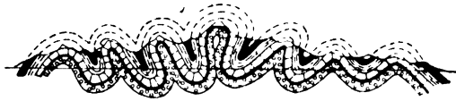
Fig. 201. Section of a folded highland after erosion. Dotted lines indicate air saddles, i.e., eroded parts of the saddles
