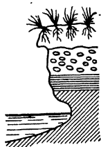
Fig. 1. River bank eroded by current
