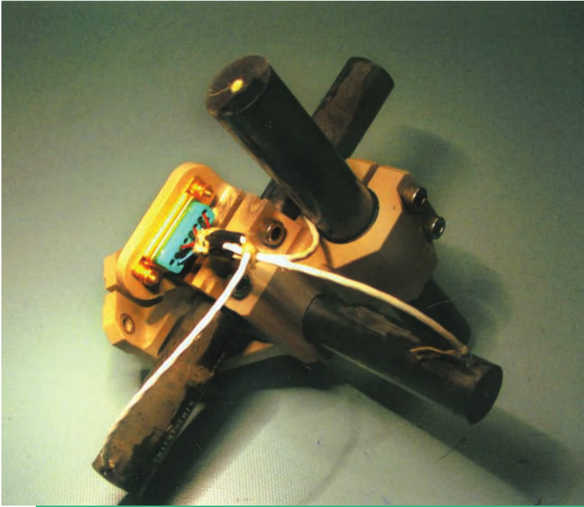
Magnetometer used to measure magnetic fields in three dimensions—note the instrument's three axes (NASA/CETP)
