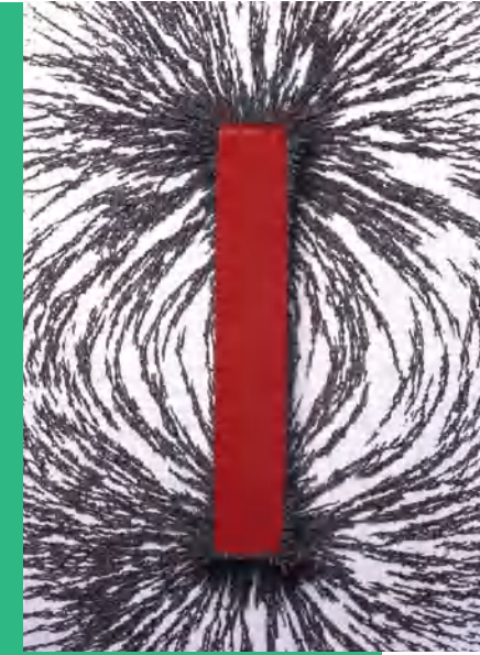
Iron filings align themselves to a bar magnet's field, showing the lines of force. (Cordelia Molloy/Photo Researchers, Inc.)
