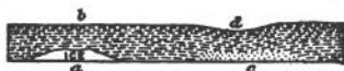
FIG. 270.—Section showing a block of ice (a) covered by aqueoglacial deposits, and a kettle hole (d) formed by the melting of a similar buried ice block. Under the kettle hole structureless sands (c) occupy the space of the melted ice. (After M. L. Fuller.)
