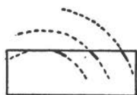
FIG. 374.—Variations in dip (short black lines) due to position of outcrops in a fold.
