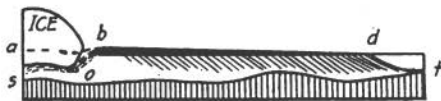
FIG. 258.—Ideal radial section of a glacial sand plain showing its relation to the ice mass and the water level. Both ice and lake were temporary. ab , esker channel; b , head of sand plain; d , front of sand plain at water level; c , backset beds; st , line of unconformity between rock floor and overlying unconsolidated deposits. (After W. M. Davis.)
