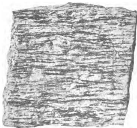
FIG. 205.—Side view of a specimen of gneiss having parallel linear structure. (Cf. Fig. 206.)
