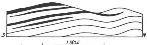
FIG. 71.—Sills of porphyry (black) in the Carboniferous formation of the Tenmile District, Colorado. (Tenmile District Special Folio, No. 48, U. S. G. S., 1898.)
