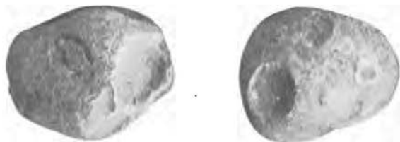
FIG. 16.—Limestone pebbles indented by solution while they were under compression in a conglomerate. The pits mark the spots where adjacent pebbles were in contact.
