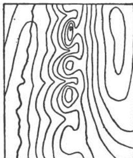
FIG. 248.—Map of a hillside ridge made by faulting. (After the California State Earthquake Investigation Commission.)
