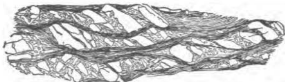
FIG. 204.—Microscopic section of "sliced" feldspars (white) in mica schist. (After C. K. Leith.)
