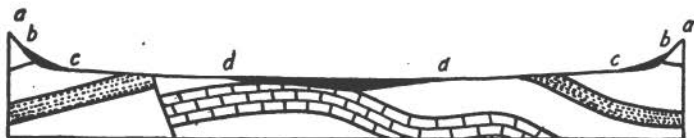
FIG. 261.—Ideal cross section of a bolson. ab , exposed mountain flanks in process of erosion; bc , relatively thick piedmont waste; cd , rock-floored plains thinly veneered with rock waste; dd , accumulating deposits of the lower central part of the basin.
