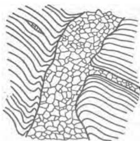
FIG. 97.—Section of a pegmatite dike cutting the foliation of a schistose rock.
