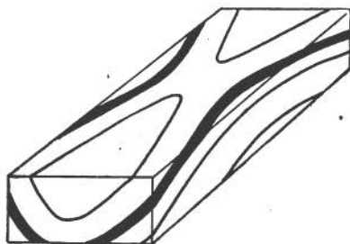
FIG. 116.—A complex fold which is synclinal in one section and anticlinal in the perpendicular section.
