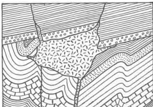
FIG. 75.—Section of a chonolith which was injected pari passu with faulting of the country rock. Intrusion was essentially passive.
