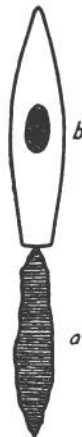
FIG. 337. — Hammer head (b) and rock specimen (a) in proper position for trimming.
