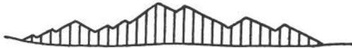
FIG. 2.—Profile section of an outcrop which is undergoing erosion through the removal of joint blocks. There are two prominent joint sets inclined in opposite directions.
