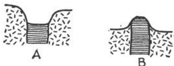
FIG. 103.—Topographic relations of a dike and its country rock. A , dike less resistant than country rock. B , dike more resistant than country rock.
