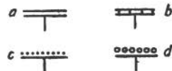
FIG. 341.—Symbols for rock type combined with a symbol for dip and strike. a, shale or slate; b, limestone; c, sandstone; d, conglomerate.
