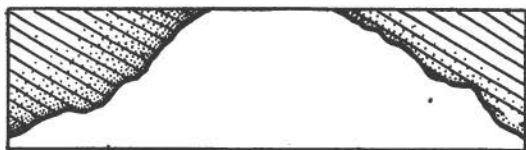
FIG. 85.—Section of an igneous contact between an intrusive rock (blank) and its stratified country rock (lined). The latter has been metamorphosed (stippling) in a wider zone on the left where the bedding is transverse to the contact.
