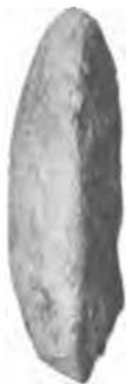
FIG. 20.—A pebble of quartzite elongated by compression in dynamic metamorphism. Length about 6 in.
