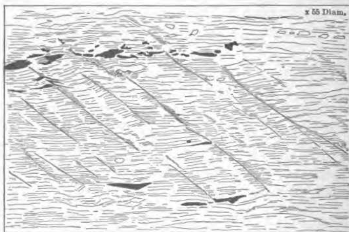
FIG. 199.—Microscopic section of fracture cleavage (diagonal) crossing flow cleavage (horizontal). (After T. N. Dale.)
