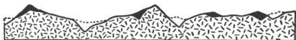
Fig. 107.—Section of part of a batholith (dash pattern) and its country rock (black). Much of the country rock has been stripped off by erosion, so that the land surface in many places essentially coincides with the roof contact. The valleys have been incised below the contact well into the batholithic mass. (The section is about 8 miles long.)
