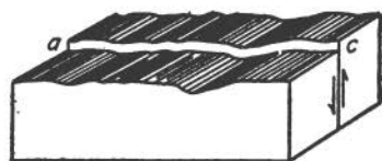
FIG. 187.—A small postglacial fault ( ac ) which interrupts the continuity of a glaciated rock surface. The edge made by the fault is about \frac{1}{4} inch high.
