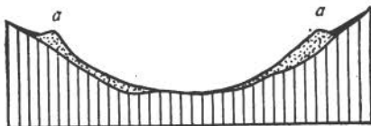
FIG. 266.—Section of a glaciated valley with lateral moraines (stippled). Talus (black) has partly filled the small valleys between the moraines and the bedrock (vertical lining).
