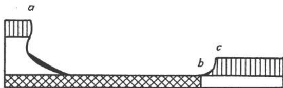
FIG. 235.—Section of a fault scarp and a fault-line scarp. Strong beds, ruled; weak beds, blank; talus, black. a has been worn back faster than c because the weak rocks are exposed in a . Before the faulting, the strong rock stratum at a and c was continuous.
