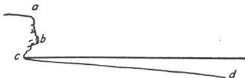
FIG 228.—Profile section of a sea cliff. ab , overhang; bc , undercut; cd , wave-cut bench.
